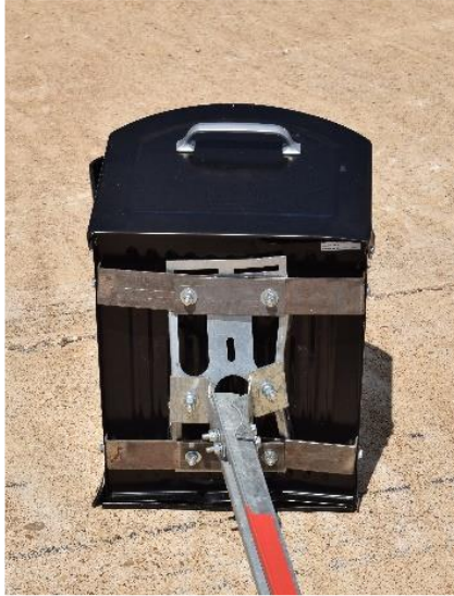
Figure 9. TxDOT Large Mailbox on Type 3 Support - Test No. 469689-1-4, Test Results
