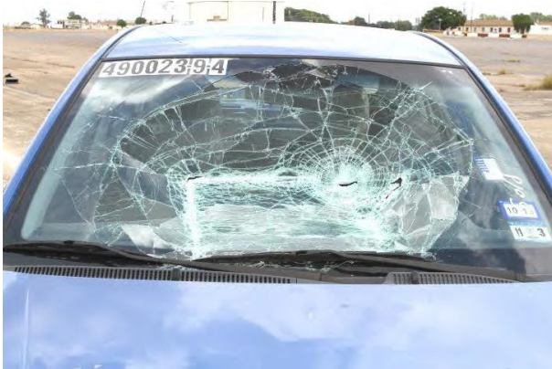
Figure 17. Locking Architectural Mailbox on Dual Mount Post - Test No. 490023-9-4, Test Results
