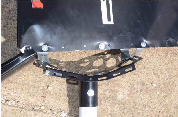
Figure 19. Single Mailbox with Recycled Rubber Support Post in Type 4 Foundation - Test No. 469468-8-1, Test Results
