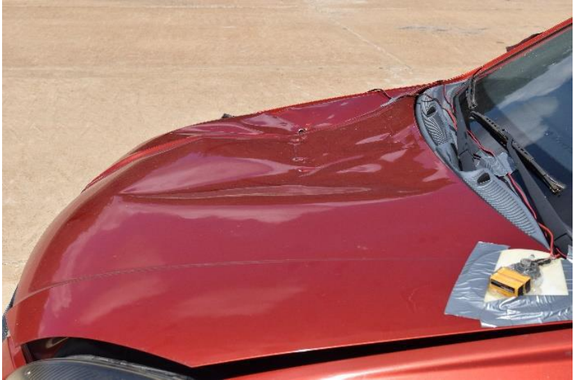
Figure 9. TxDOT Large Mailbox on Type 3 Support - Test No. 469689-1-4, Test Results
