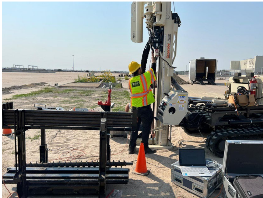
Figure 4.13 CPT test conducted by the research team.
