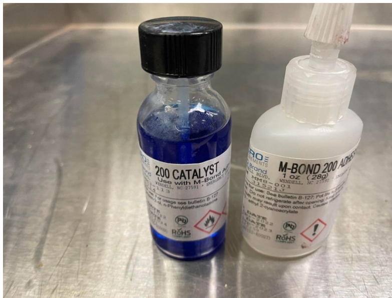
Figure 4.17 Cleaning liquid and adhesive used for resistive strain gauge installation (from Micro-Measurements VPG).
