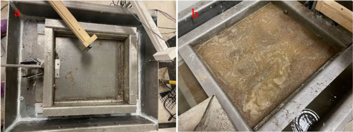
Figure 3.11 Implementation of the large-scale direct shear tests in (a) dry, and (b) submerge conditions.
