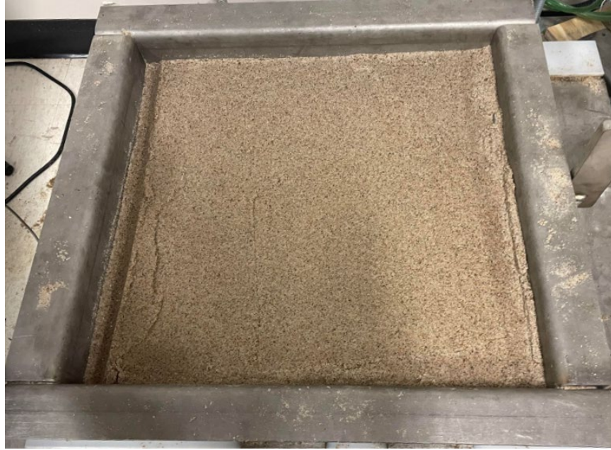
Figure 3.6 Fill sand in the shear box.
