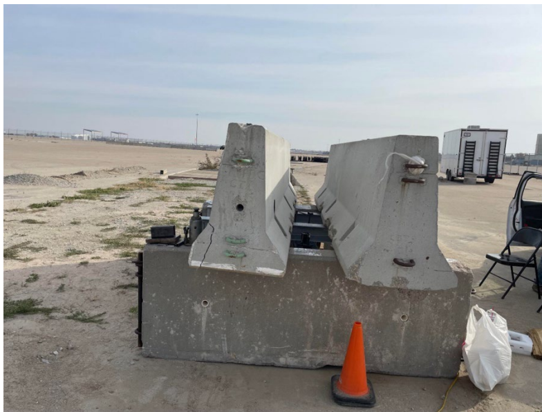
Figure 4.23 A photo of the axial loading test setup with the reaction beam (side view).
