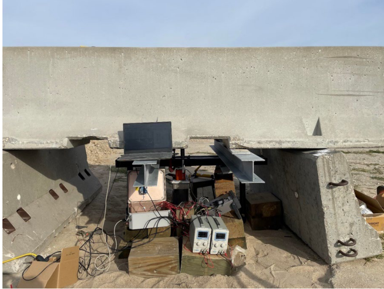
Figure 4.22 A photo of the axial loading test setup with the reaction beam (front view).
