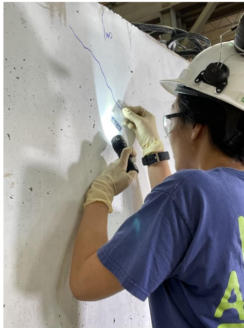
Figure 5-17 Concrete crack marking and measuring
