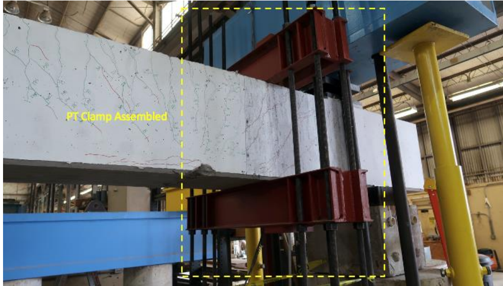
Figure 6-18 Post-tensioned clamp added to specimen after Test 1 in preparations for Test 2
