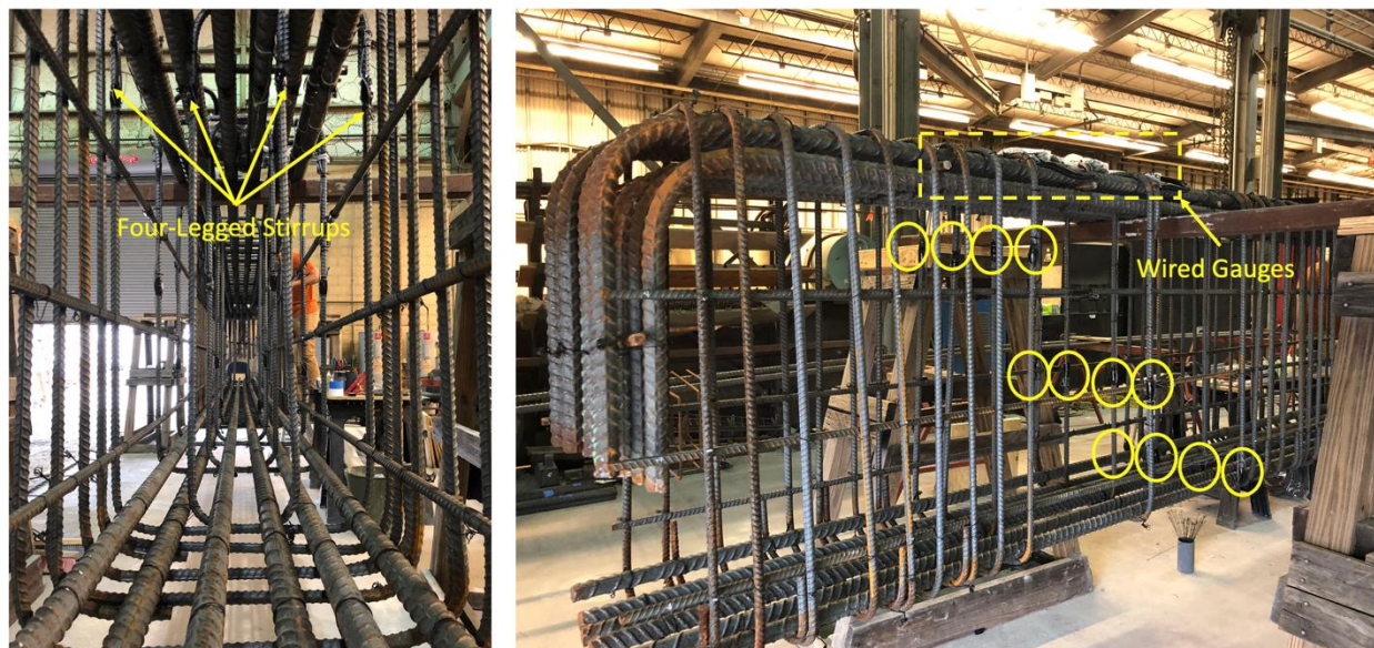
Figure 6-10 Gauges along the strut with wiring and packaging for B1
