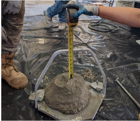
(c) Slump test
