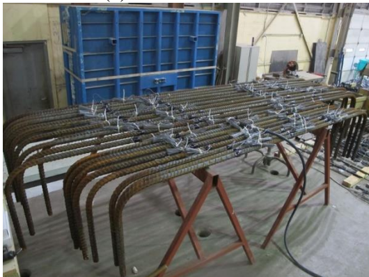
(c) Installed strain gauges
