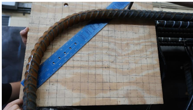
Figure 4-10 Measuring bend radius
