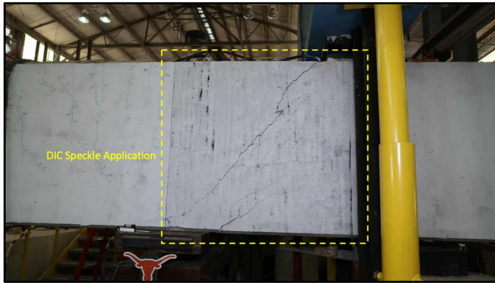
Figure 6-17 Speckling for DIC applied to area of interest
