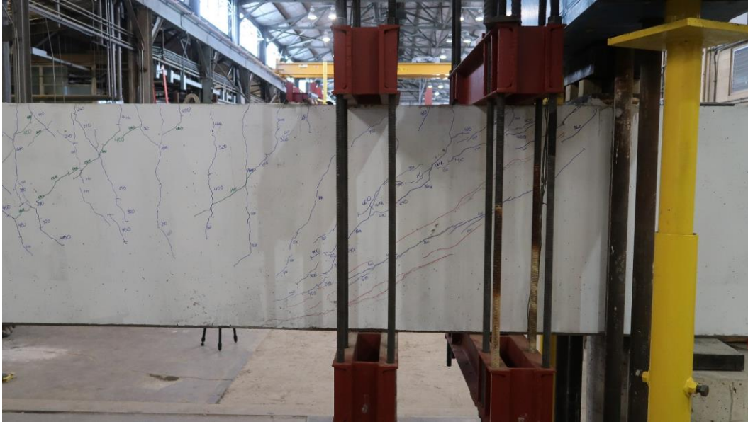
Figure 5-18 Post-tension clamping as external protection
