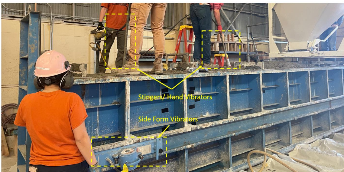
Figure 6-12 Specimen casting and vibration techniques
