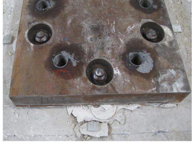
(b) Concrete spalling formed around loading plate
