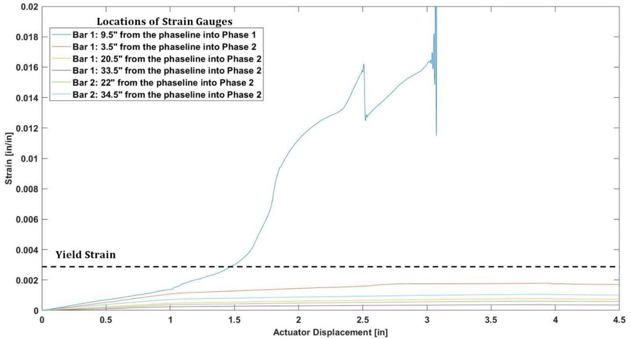
Figure 5. 20 Strain as a function of actuator displacement for Specimen 2.
