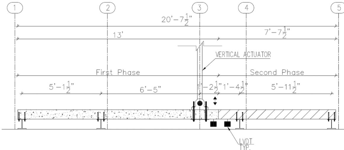
**Figure 5. 9 Elevation view of LVDT instrumentation**
