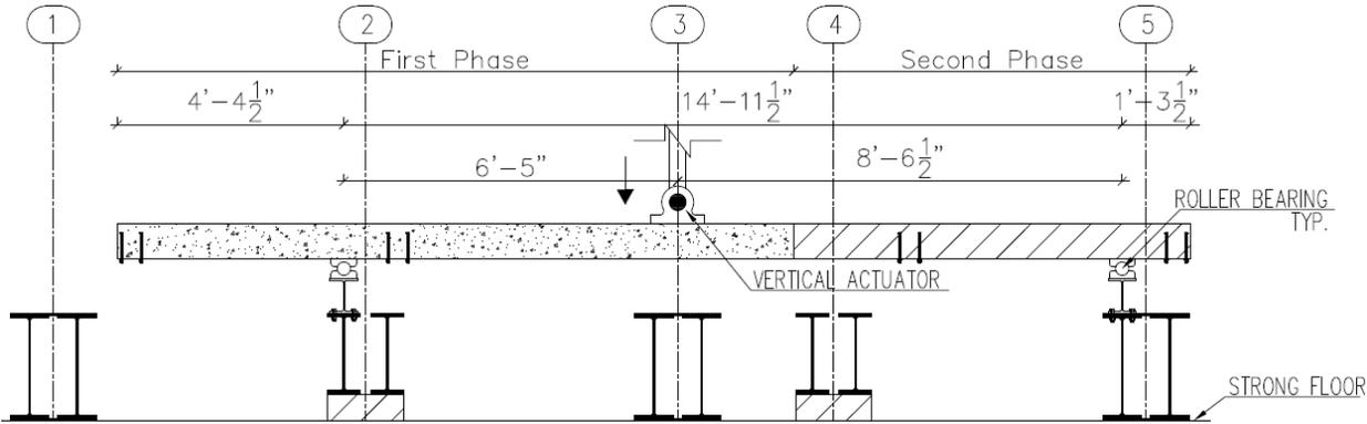
Figure 5. 6 Monotonic test setup
