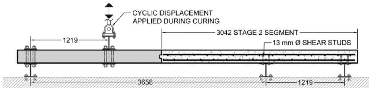
**Figure 2. 3 Physical test setup by Weatherer et al (2019). Units: mm.**
