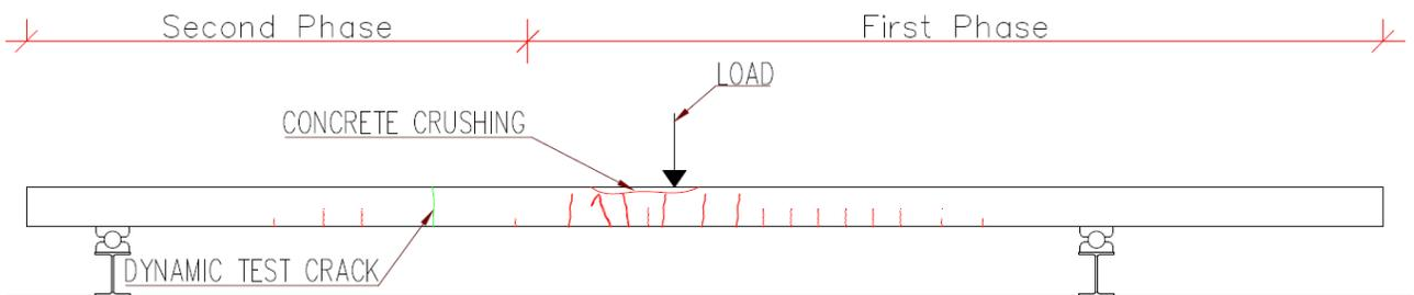
**Figure 5. 17 Crack map of Specimen 2 after the monotonic test.**
