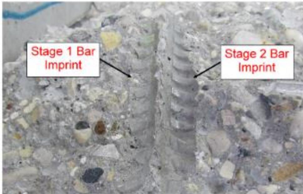
**Figure 2. 4 Rebar imprints from the full-scale test of traffic-induced vibration by Weatherer et al. (2019).**
