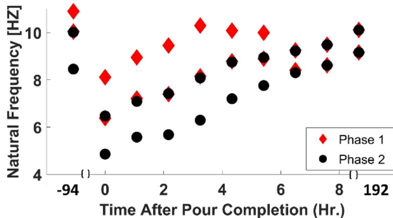
Figure 4. 12 Lowest two natural frequencies of each phase of Bridge 1 as a function of time with respect to the start of the second phase deck pour.
