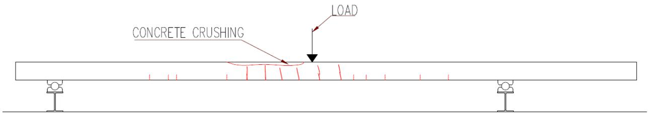
**Figure 5. 15 Crack map of Specimen 0 after the monotonic test.**
