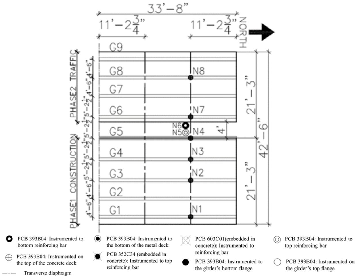
Figure 4. 6 Instrumentation layout for test T1-BR1
