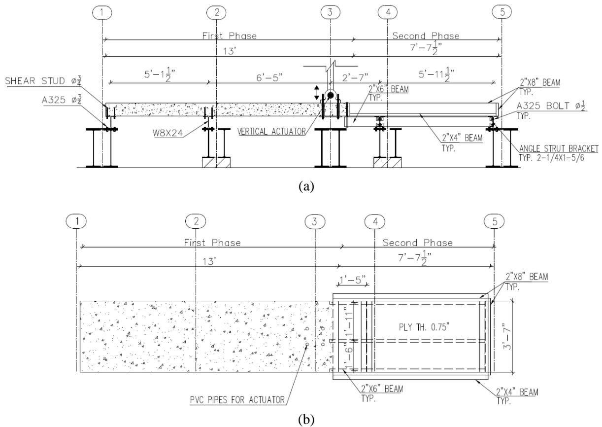
**Figure 5. 1 (a) Elevation and (b) plan view of the dynamic test setup and formwork details of the second-phase deck.**
