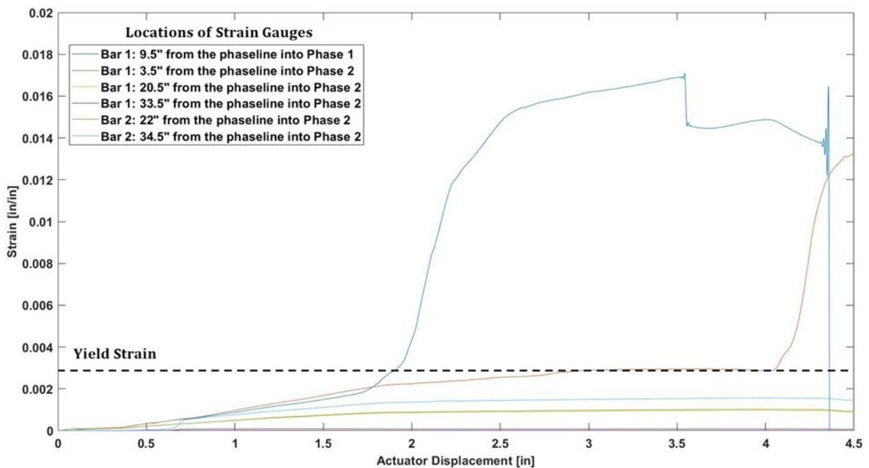
Figure 5. 18 Strain as a function of actuator displacement for Specimen 0.
