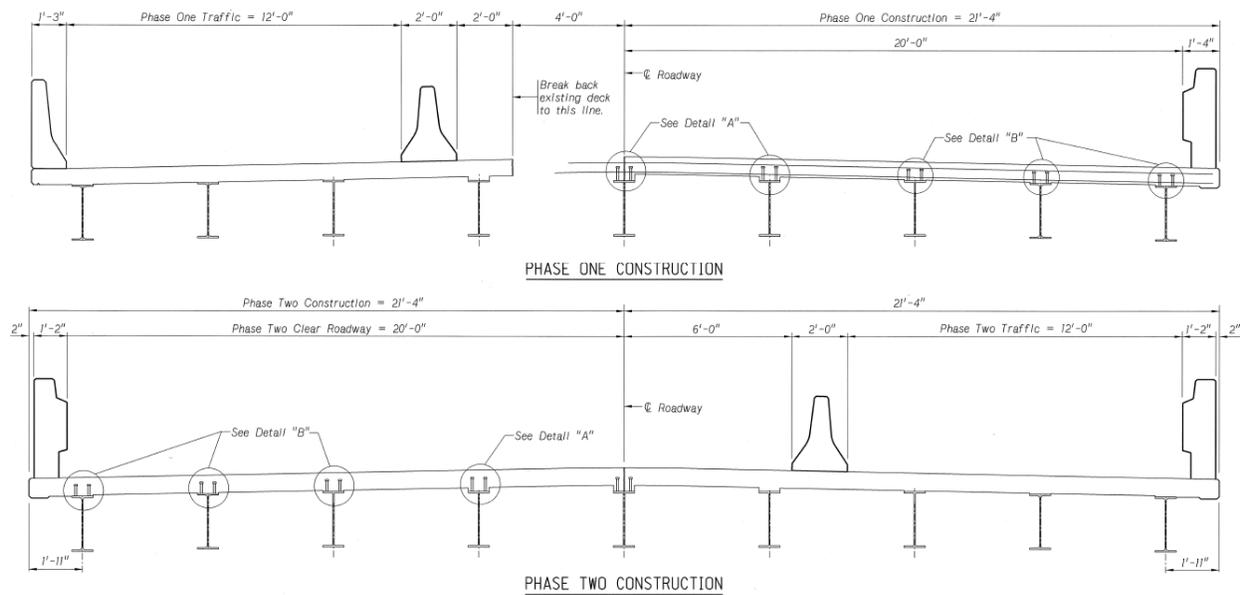
**Figure 4. 1 Phasing of the deck replacement at Brunswick Viaduct Bridge (Bridge 1)**
