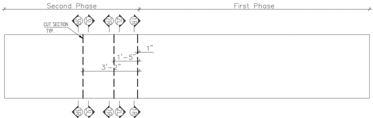
**Figure 5. 21 Locations of cutting planes for Specimens 0, 1, and 2.**
