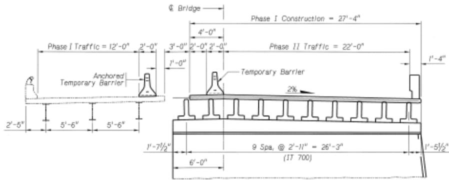
**CROSS SECTION AT NEW BENT**
