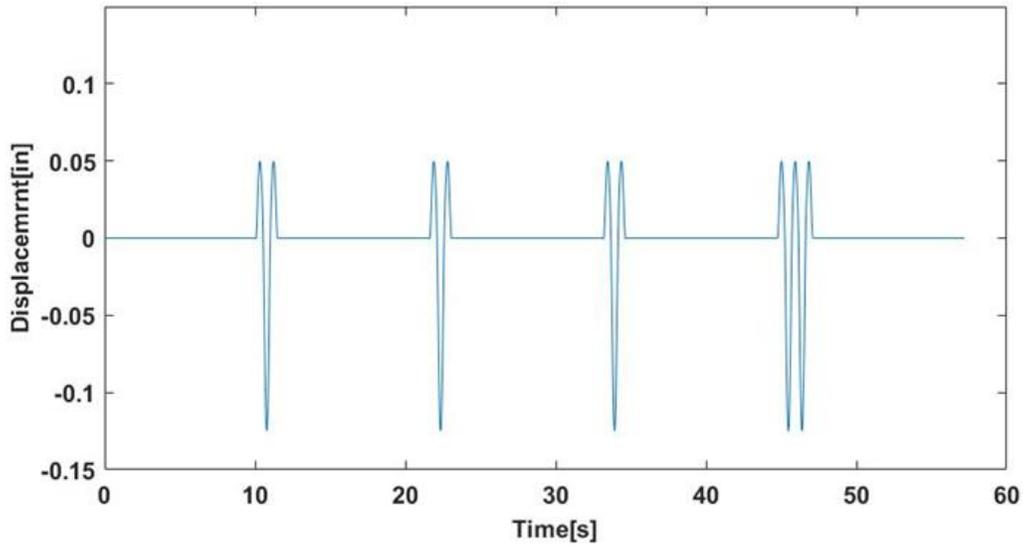
Figure 5. 5 Simulated traffic-induced vibration displacement protocol for 0-3 hours.
