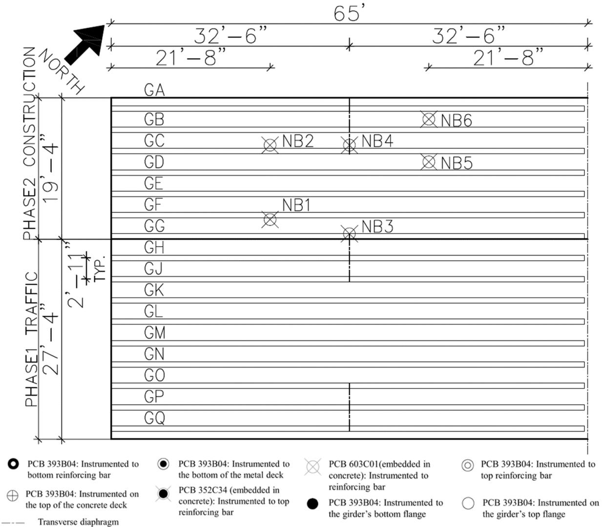
**Figure 4. 10 Instrumentation layout for the rebar during T2-BR2, T3-BR2, and T4-BR2**
