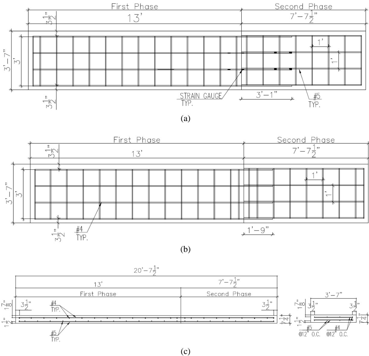
**Figure 5.3 Plan view of the specimen's (a) bottom and (b) top reinforcement details; and (c) side views of the specimen's reinforcement details.**
