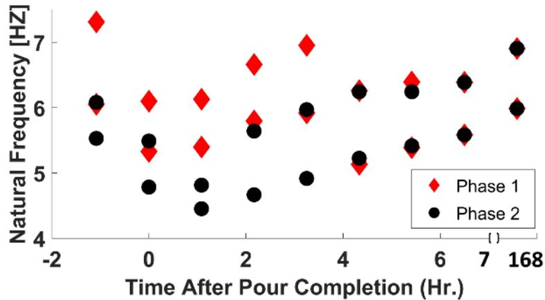
Figure 4. 13 Lowest two natural frequencies of each phase of the Bridge 2 as a function of time with respect to the start of the second phase deck pour.
