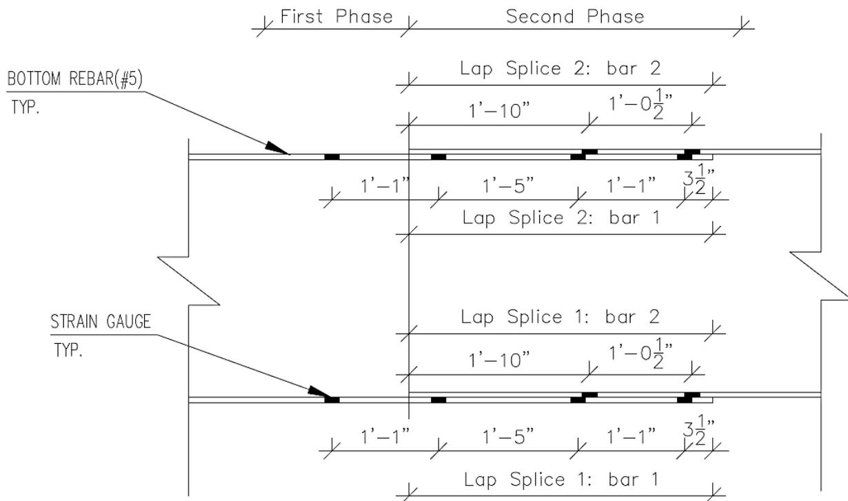
Figure 5. 8 Plan view of strain gauge instrumentation
