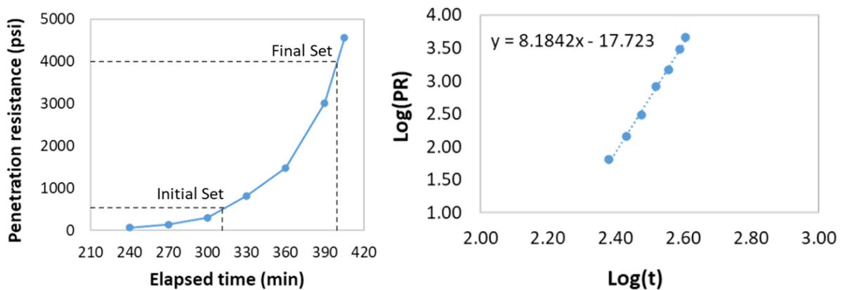
**Figure 5. 10 Penetration resistance versus elapsed time and log-log plot with linear regression.**
