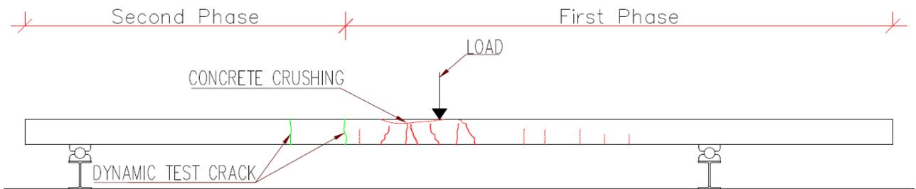
**Figure 5. 16 Crack map of Specimen 1 after the monotonic test.**
