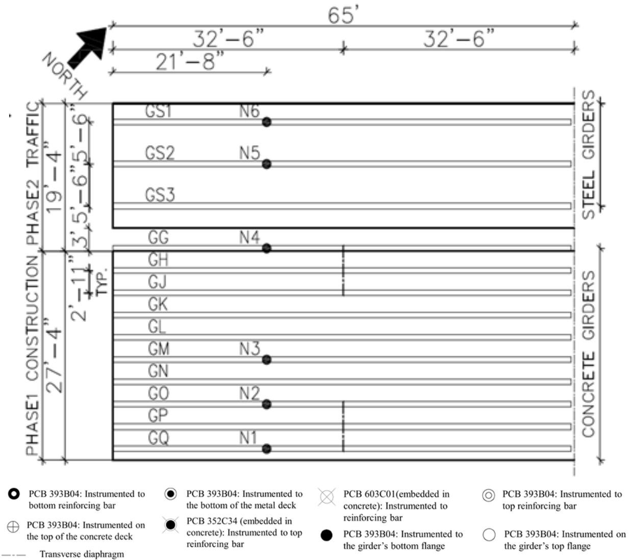
**Figure 4. 9 Instrumentation layout for test T1-BR2**
