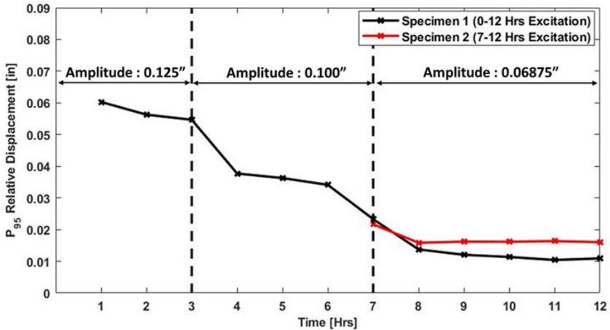
Figure 5. 11 Relative displacements between the first and second phases over the dynamic test duration.
