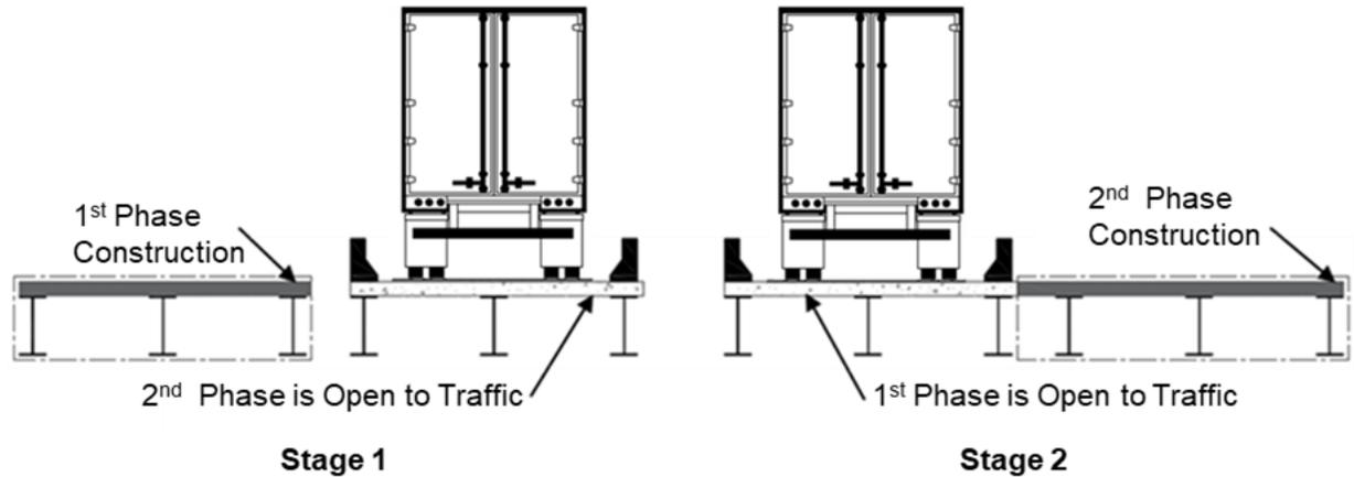
**Figure 1. 1 Typical phased construction sequence of a bridge.**
