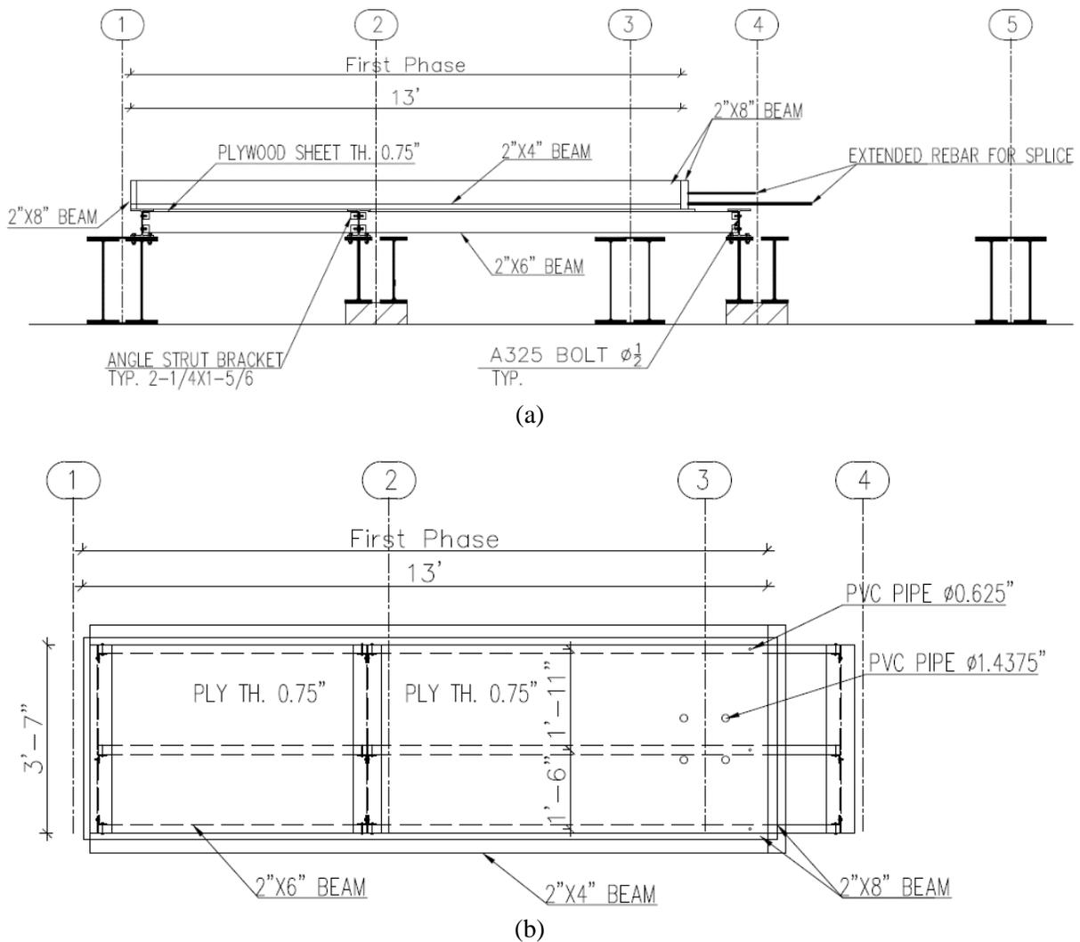
**Figure 5. 4 (a) Elevation and (b) plan view of the first phase of construction formwork.**
