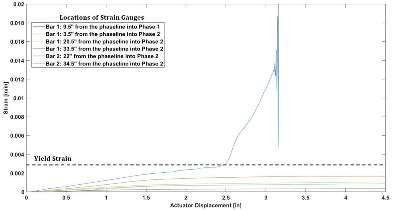
Figure 5. 19 Strain as a function of actuator displacement for Specimen 1.
