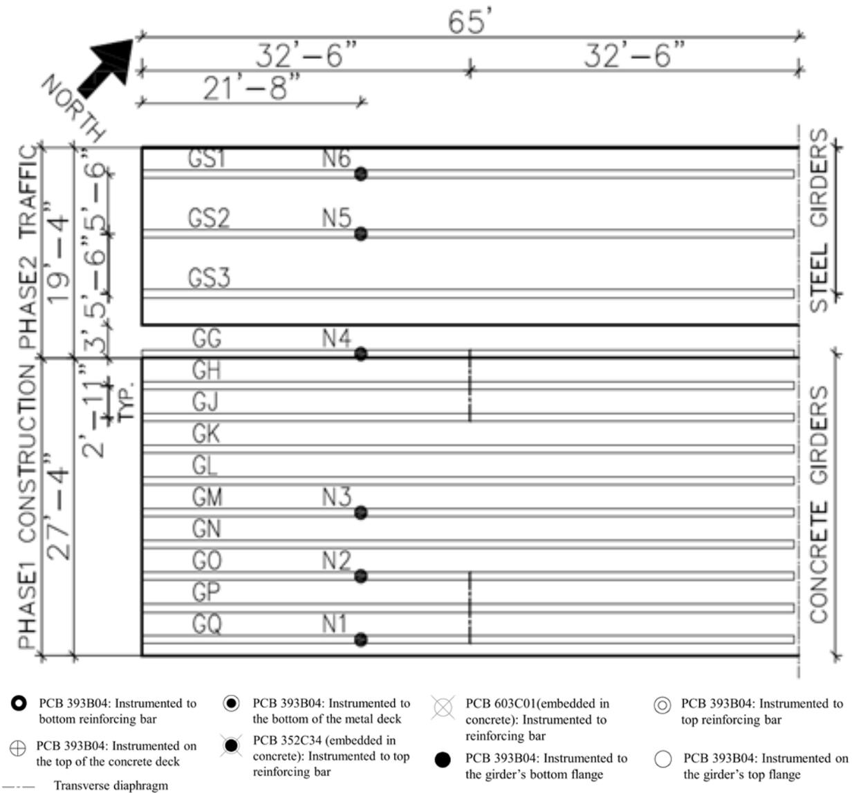
**Figure 4. 11 Instrumentation layout for girders during T2-BR2, T3-BR2, and T4-BR2**
