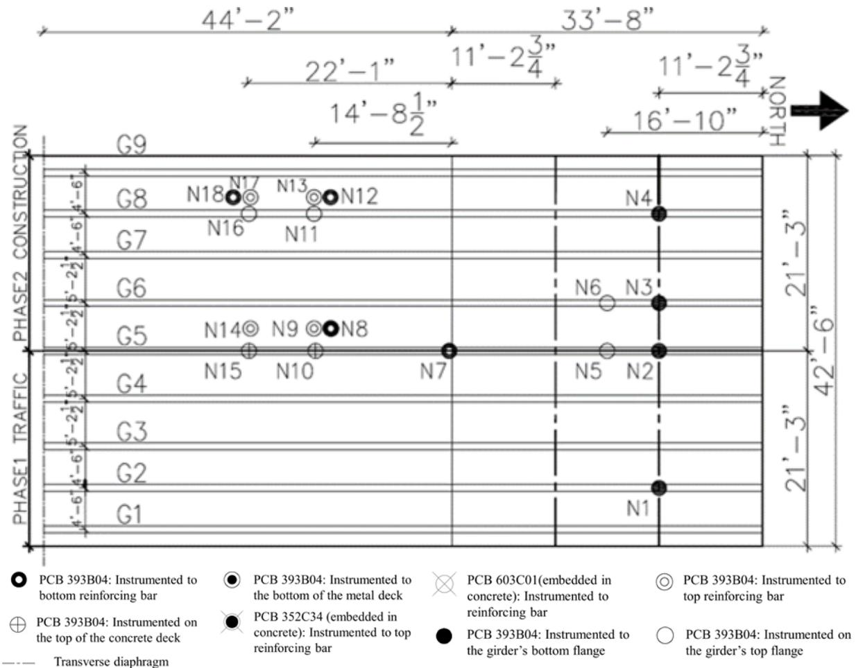
Figure 4. 7 Instrumentation layout for test T2-BR1
