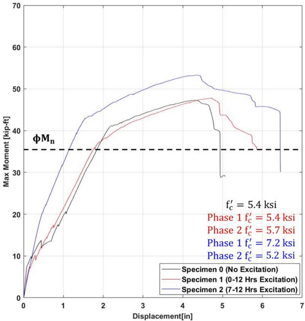
Figure 5. 14 Maximum moment as a function of actuator displacement for monotonic tests.
