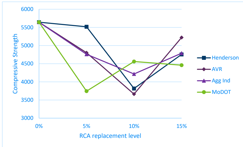
Figure 4.9: 28-day compressive strength versus RCA replacement level
