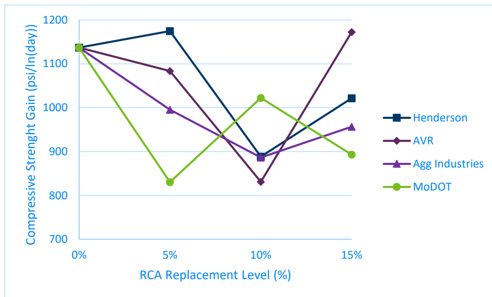
Figure 4.10: Rate of compressive strength gain versus RCA replacement level
