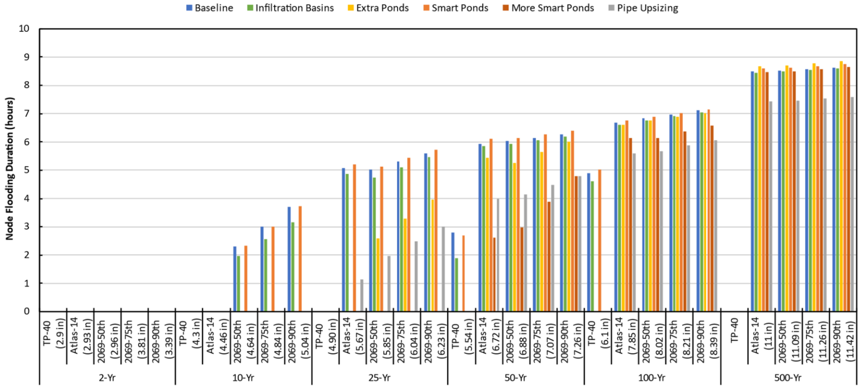
Figure A-42: Flood duration in hours for the 2-, 10-, 25-, 50-, 100-, and 500-year storms at node SP64 in Rochester.
