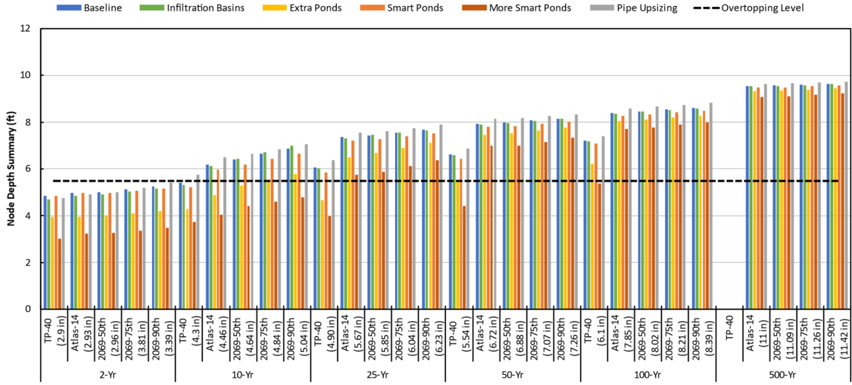
Figure A-35: Node Depth in ft for the 2-, 10-, 25-, 50-, 100-, and 500-year storms at node SP113 in Rochester.
