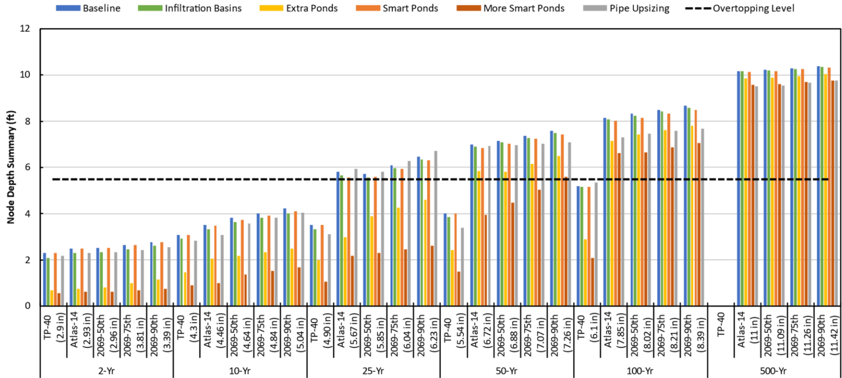
Figure A-34: Node Depth in ft for the 2-, 10-, 25-, 50-, 100-, and 500-year storms at node RN176248 in Rochester.
