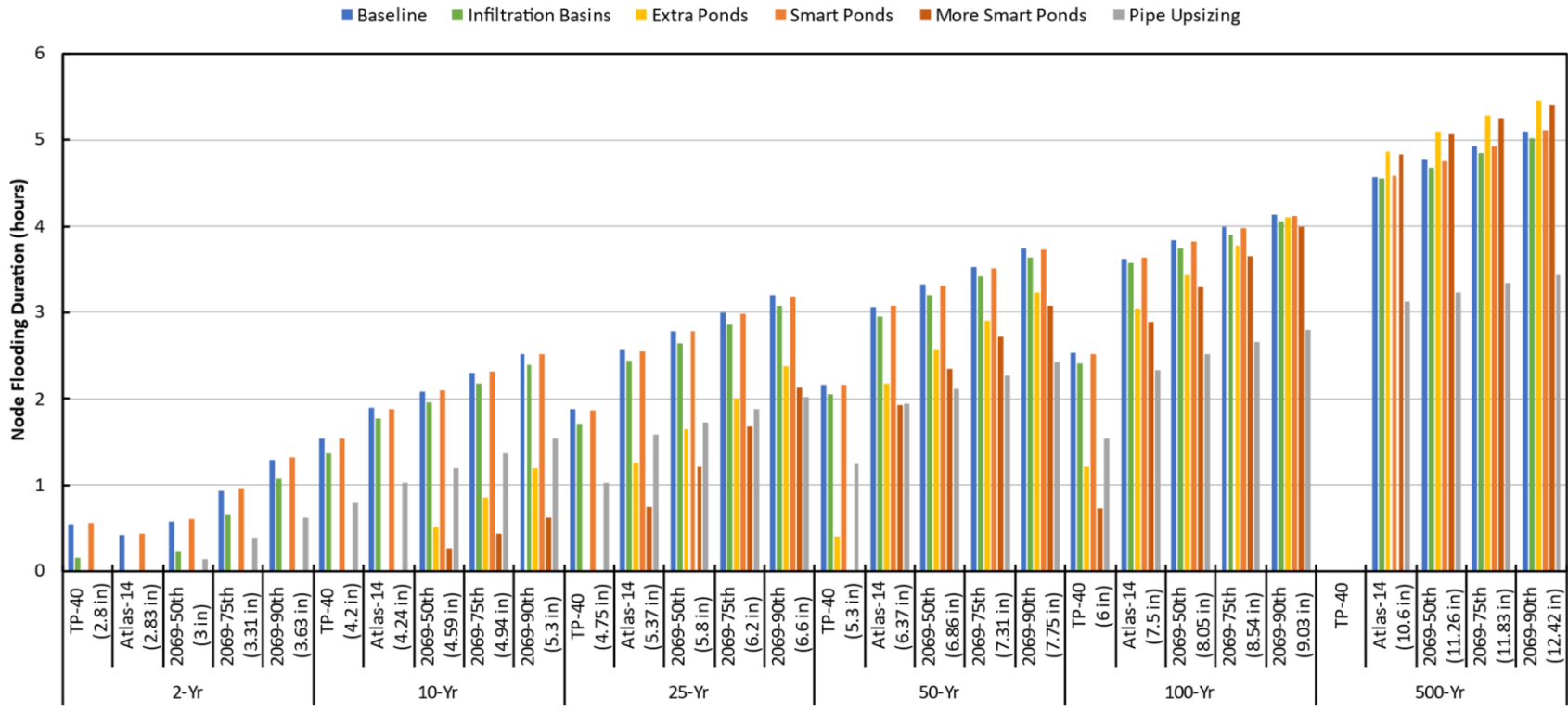
Figure A-26: Flood duration in hours for the 2-, 10-, 25-, 50-, 100-, and 500-year storms at node MH420743 in Minneapolis.
