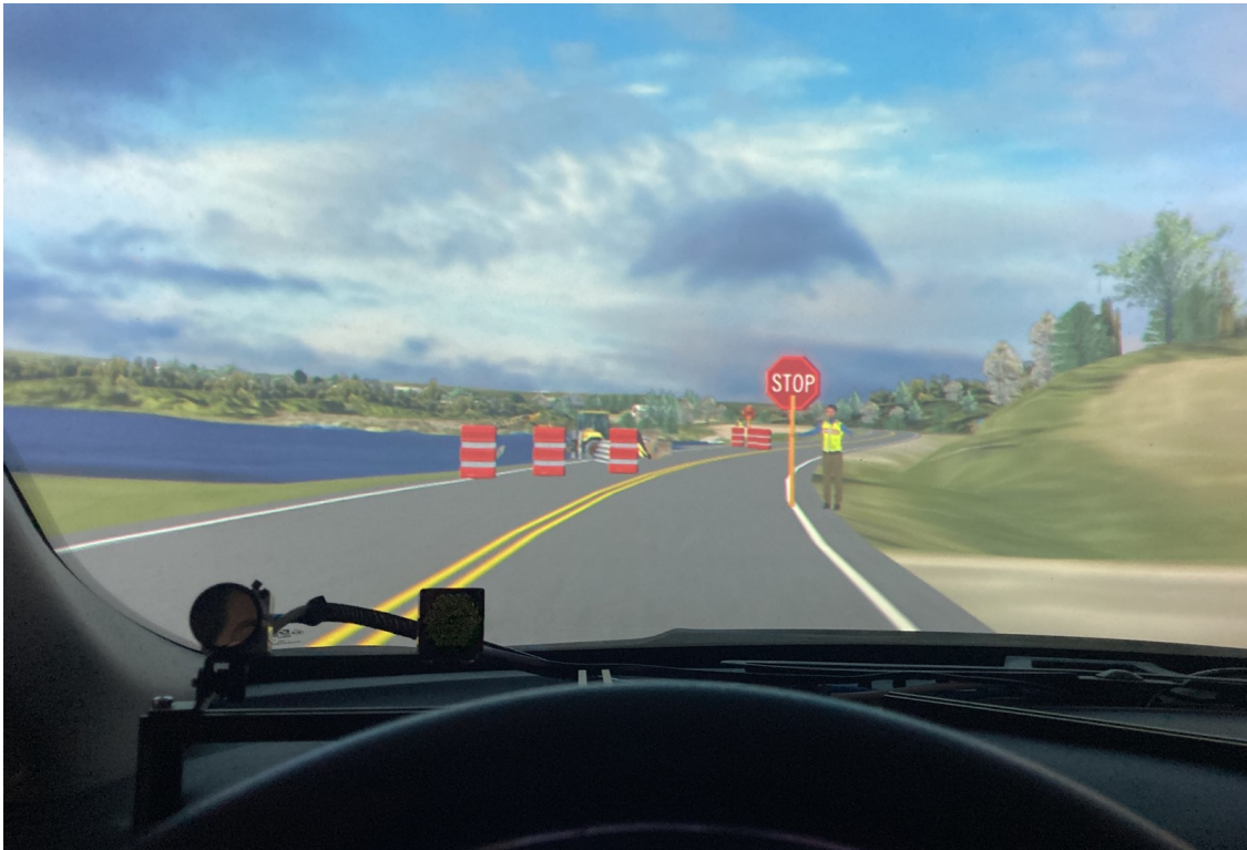
Figure 5.2 Image of flagger displaying STOP sign at work zone
