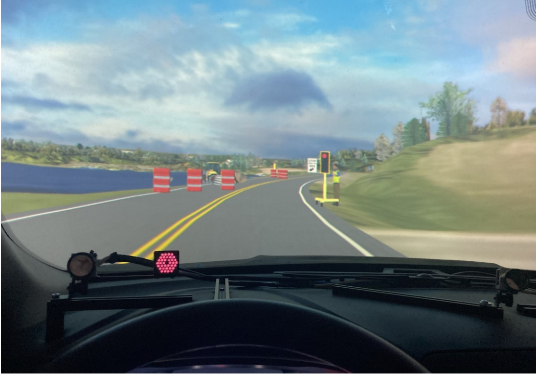
Figure 5.4 Image of experimental traffic signal signaling to stop at work zone
