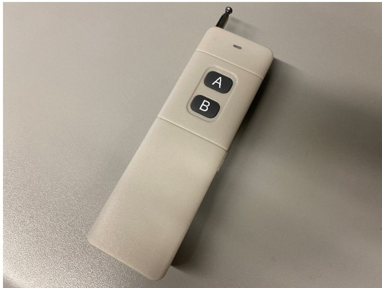
Figure 2.3 Remote controller for operating smart traffic signal.
