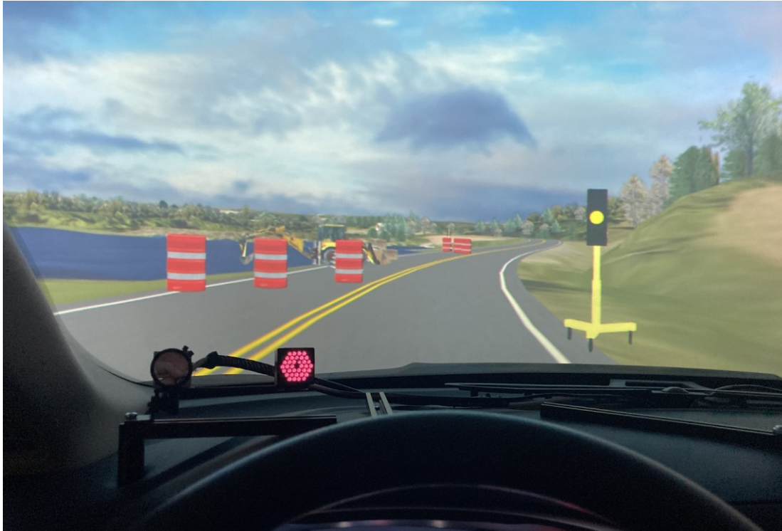
Figure 4.11 Image of driver's perspective of signal displaying flashing yellow light at work zone
