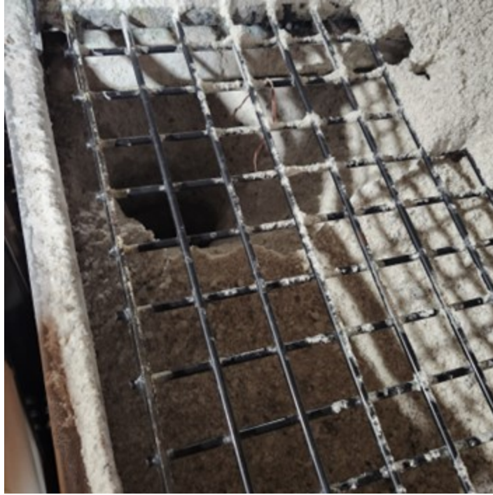
Figure 7.2. Salt bridging on a slurry spreader.
