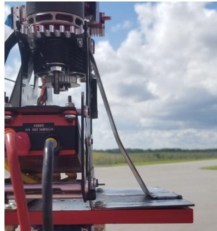
Figure 30. Rotor mount supports buckle due to vibrations
