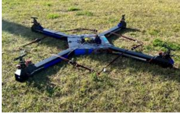
Figure 60. PAVER V.1 strapped on the ground for testing
