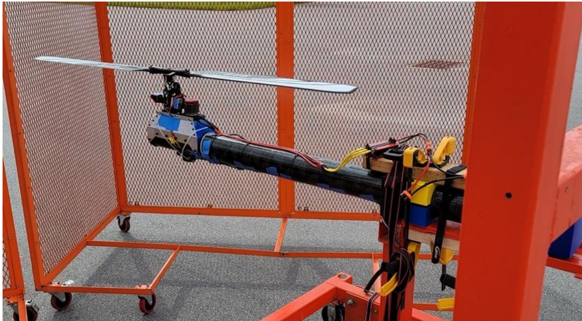
Figure 113. Single arm structural test setup
