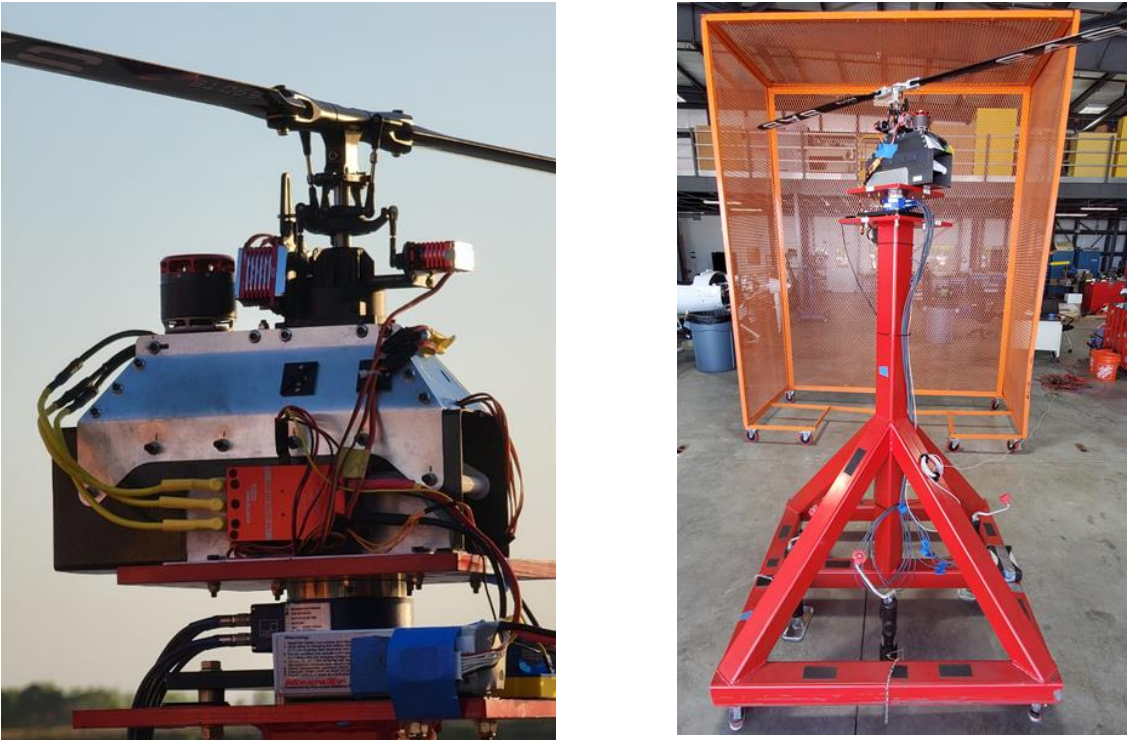
Figure 35. Rotor test stand configuration
