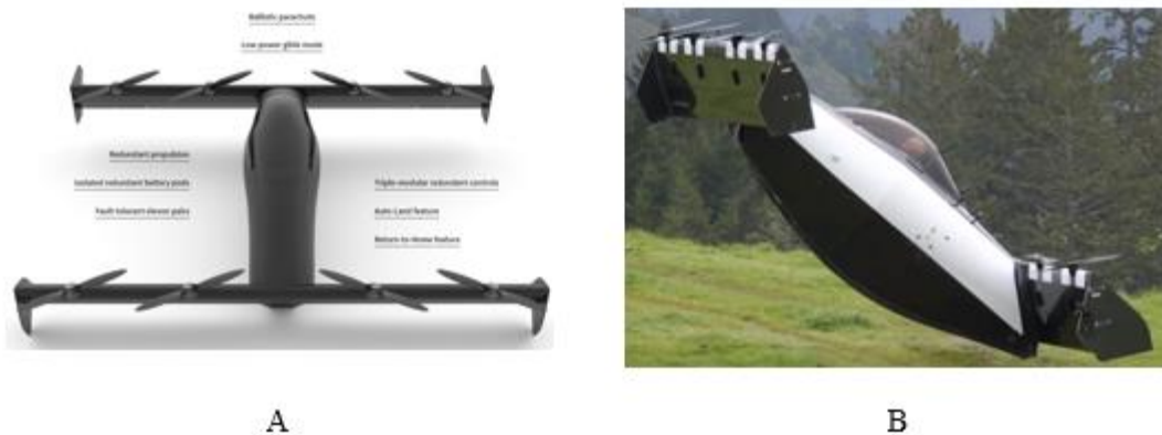
Figure 7. Opener’s Ultra-light BlackFly A) features list and in B) vertical landing (credit: opener.aero)
