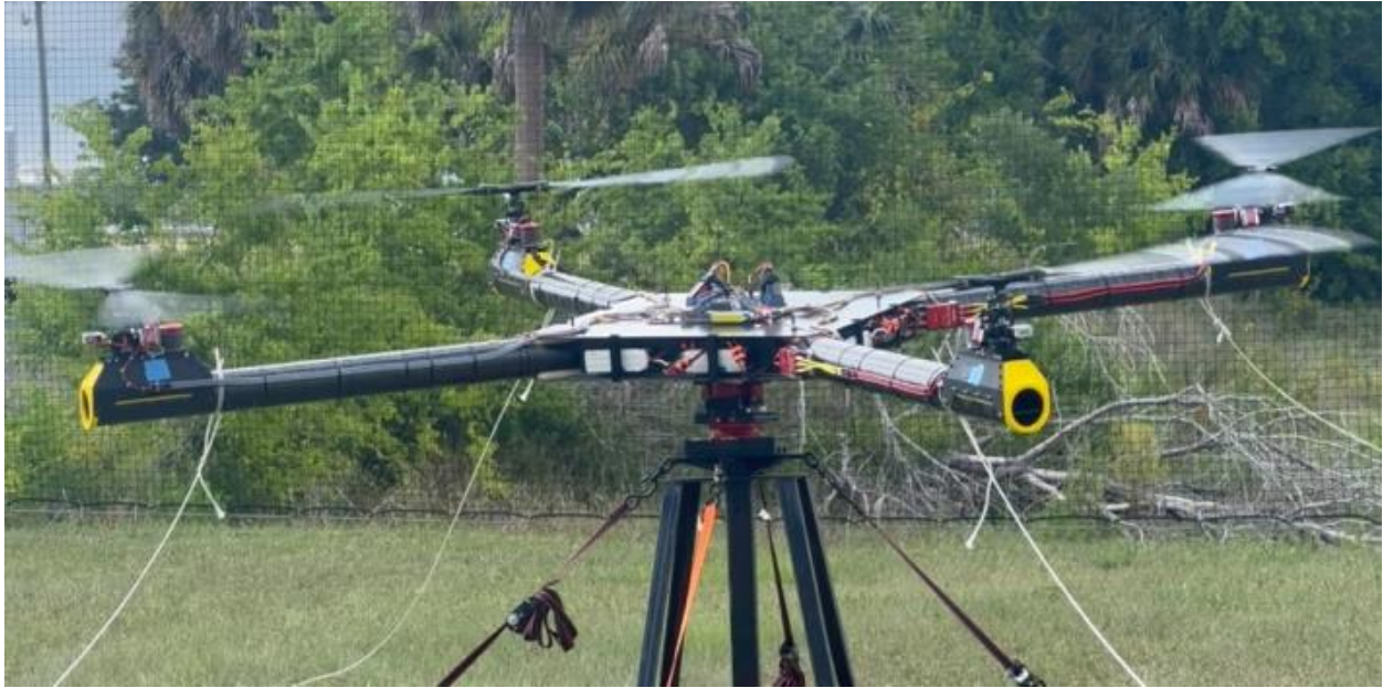
Figure 97. Attitude test stand with vehicle's arms tethered
