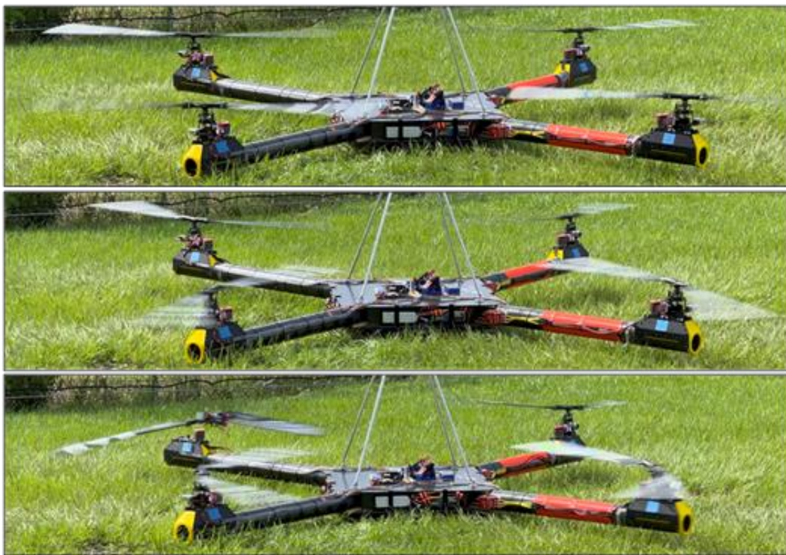
Figure 143. Key frames of PAVER ground resonance
