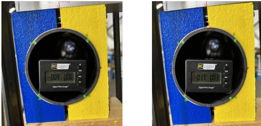
Figure 65. Twist angle indicated on the pitch gauge
