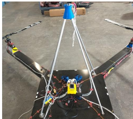
Figure 107. First iteration of the test harness mounted to PAVER
