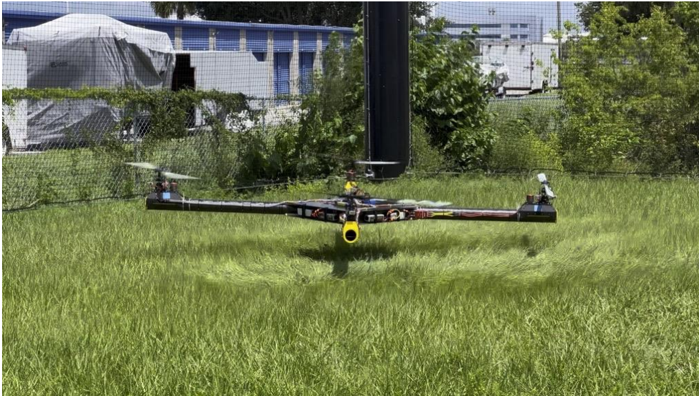
Figure 106. PAVER hovering with one rotor off (motor-out condition)
