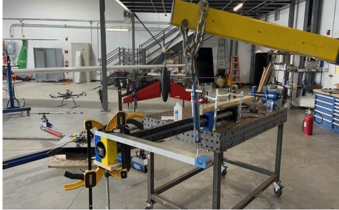
Figure 64. Test setup of the carbon fiber drive shaft
