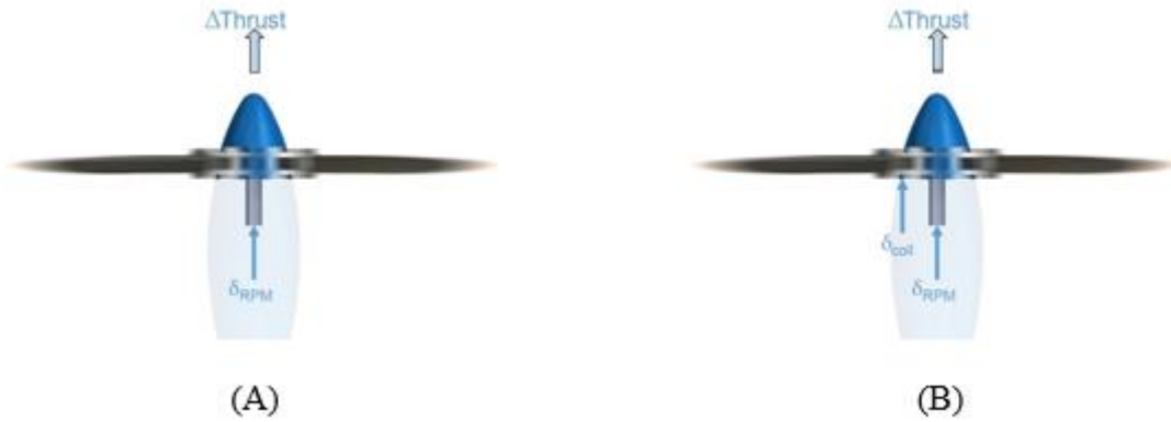
Figure 2. A) Thrust change by RPM only and B) by collective pitch and/or RPM change
