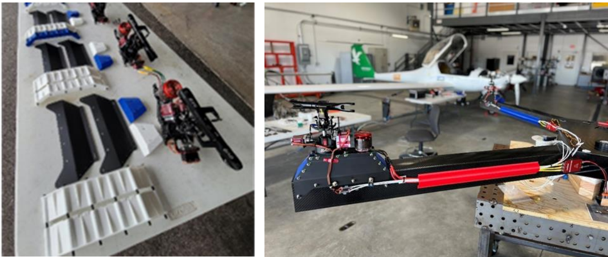
Figure 59. The DEP units are assembled on the end of carbon fiber square tubes
