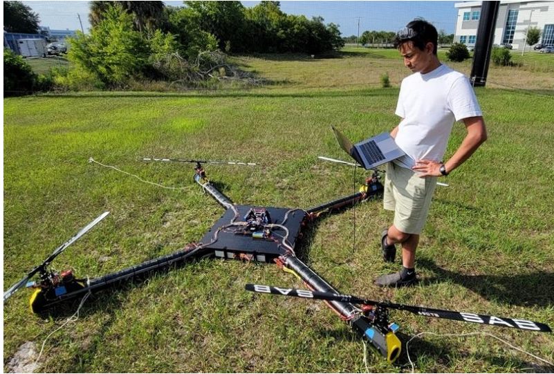
Figure 103. Conducting pre-flight checks on cyclic pitch control
