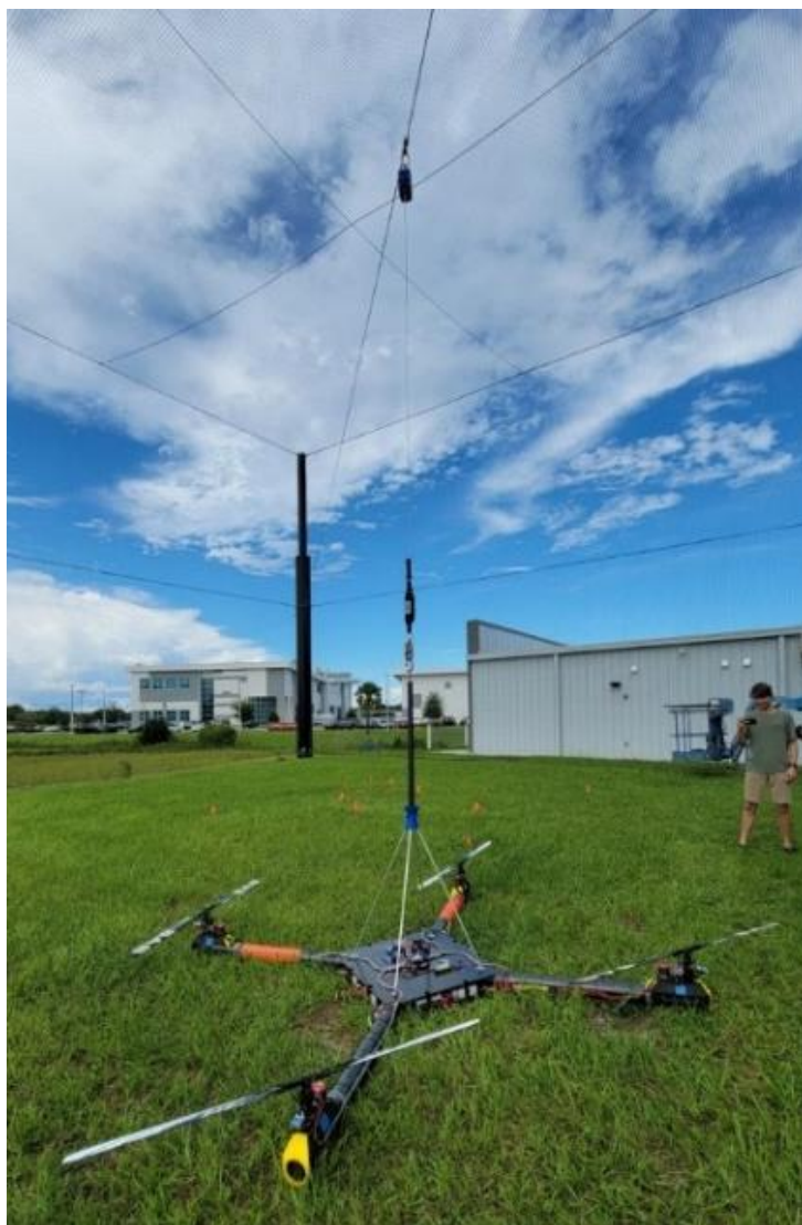
Figure 109. PAVER strapped to the zipline in the test cage
