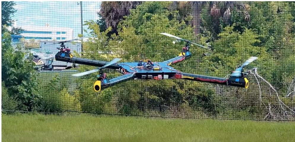
Figure 105. PAVER performing maneuvers in an untethered flight-test
