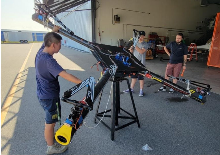
Figure 104. Checking the vehicle's bank & pitch limits on the ATS
