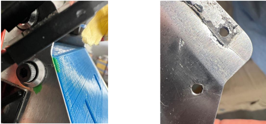
Figure 32. Cracks found on aluminum unit plates after tests
