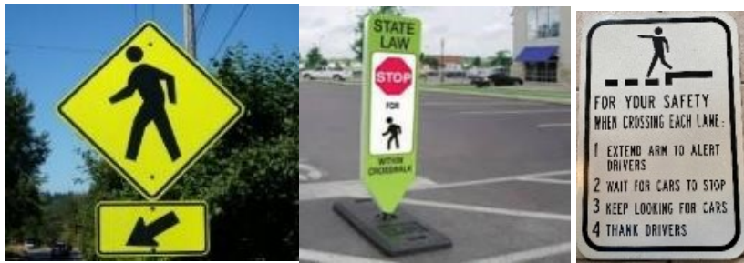
Figure 2.6 Standard crosswalk sign (W11-2 with W16-7) (Left), R1-6 In-street pedestrian sign (Center), and Pedestrian signage to encourage gesturing (Right) (Crowley-Koch et al., 2011)
