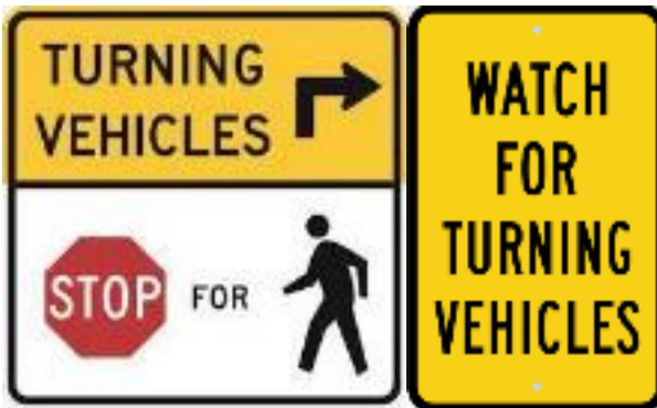
Figure 2.5 Proposed signalized intersection signage treatments for driver of turning vehicles (left) and pedestrians to watch for turning vehicles (right)
