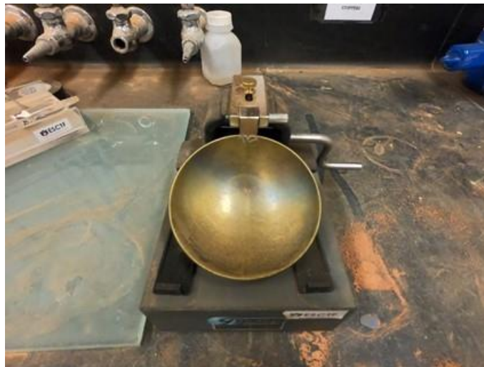
Figure 4-20: Manual Casagrande Liquid Limit Tool.
