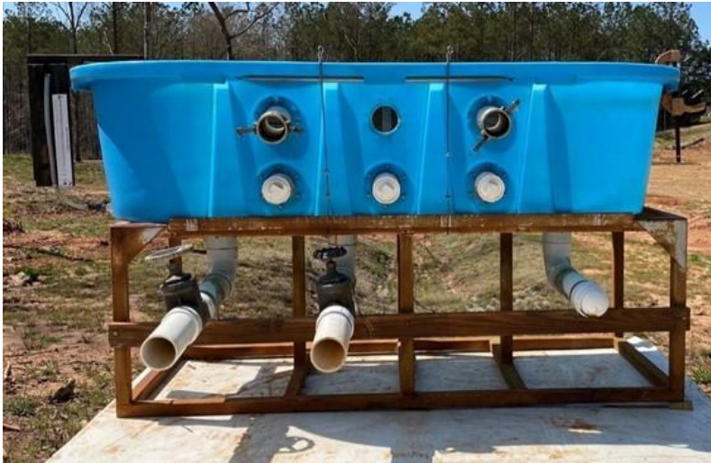
(a) the backside of the equalizing flow tank
