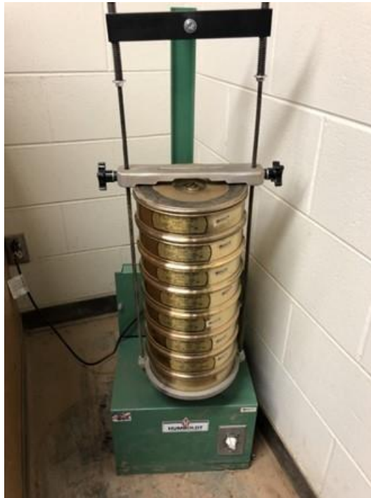
Figure 4-18: Sieve Machine Setup.
