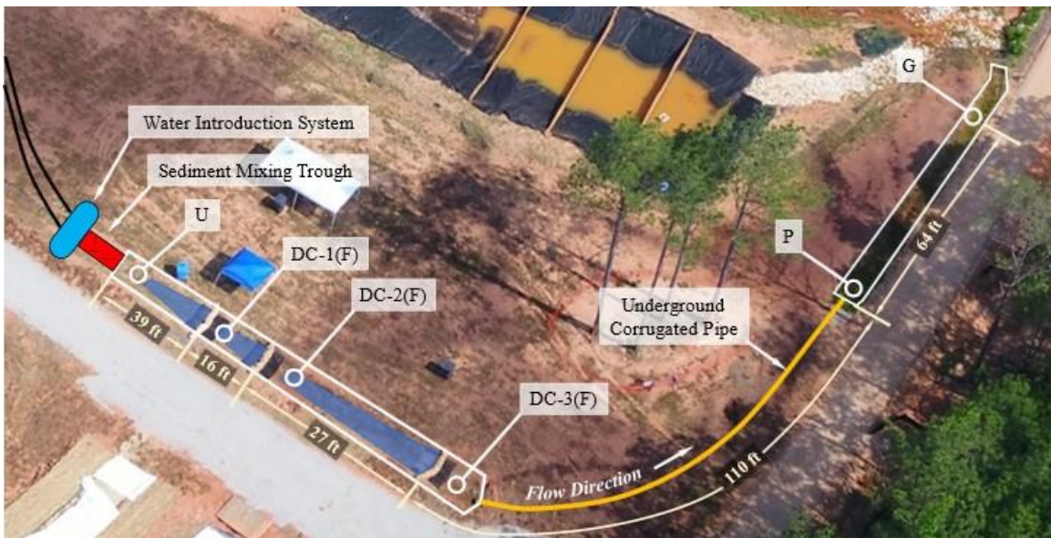
Figure 6-10. Wattle Product A-G Large-Scale-Testing Setup
