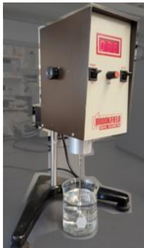
Figure 4-4. Brookfield Digital Viscometer Testing Apparatus
