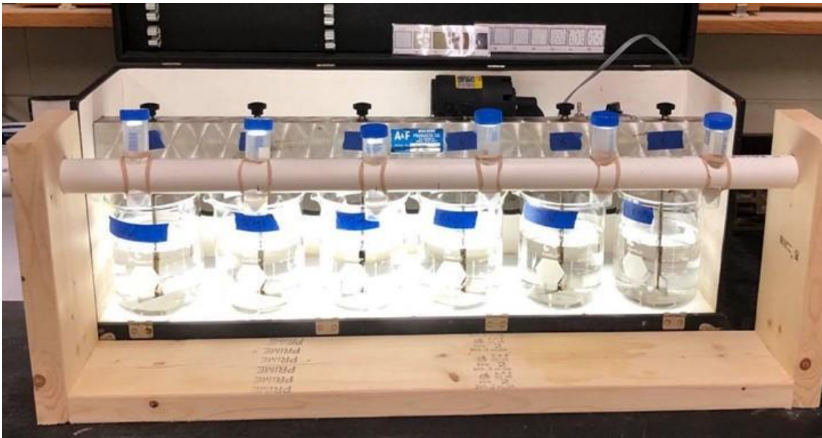
Figure 4-22: Flocculant Injection Rack
