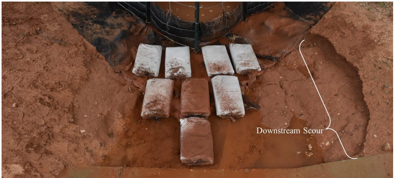
Figure 6-29. Observed Downstream Scour After Large-scale Block Test
