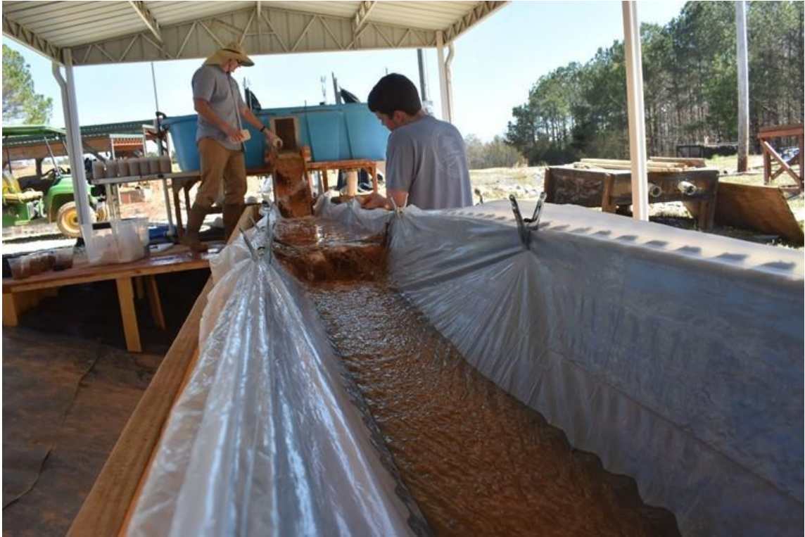
Figure 5-17: Subcritical Flow Evaluations
