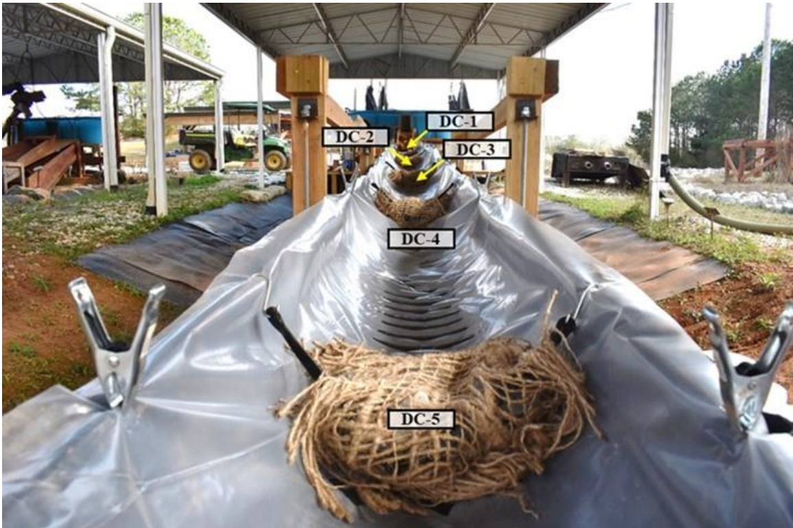
Figure 5-11: Scaled-down Rock Ditch Checks in the Flume
