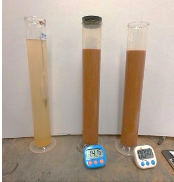
Figure 4-19: Hydrometer Testing Setup.
