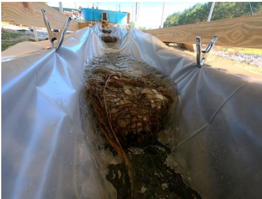
Figure 5-13: Clearwater Flume Experiments with a Granular Form
