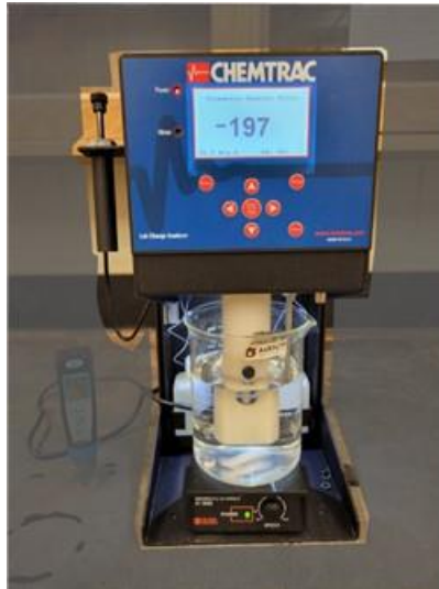
Figure 4-7. Laboratory Charge Analyzer Testing Apparatus
