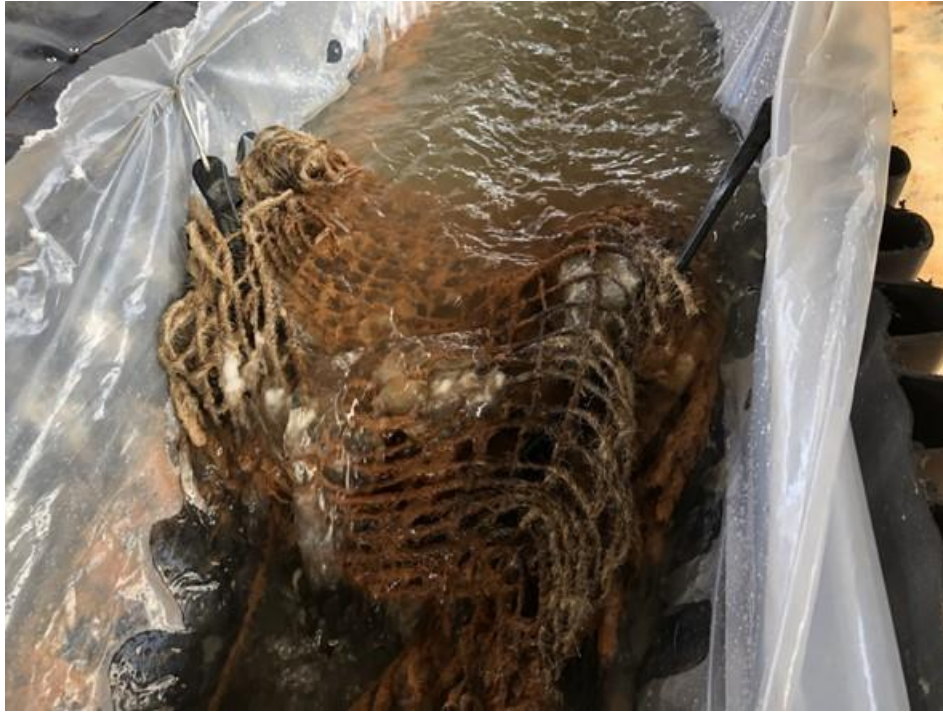
Figure 5-18: Longevity Test Clear Water Introduction
