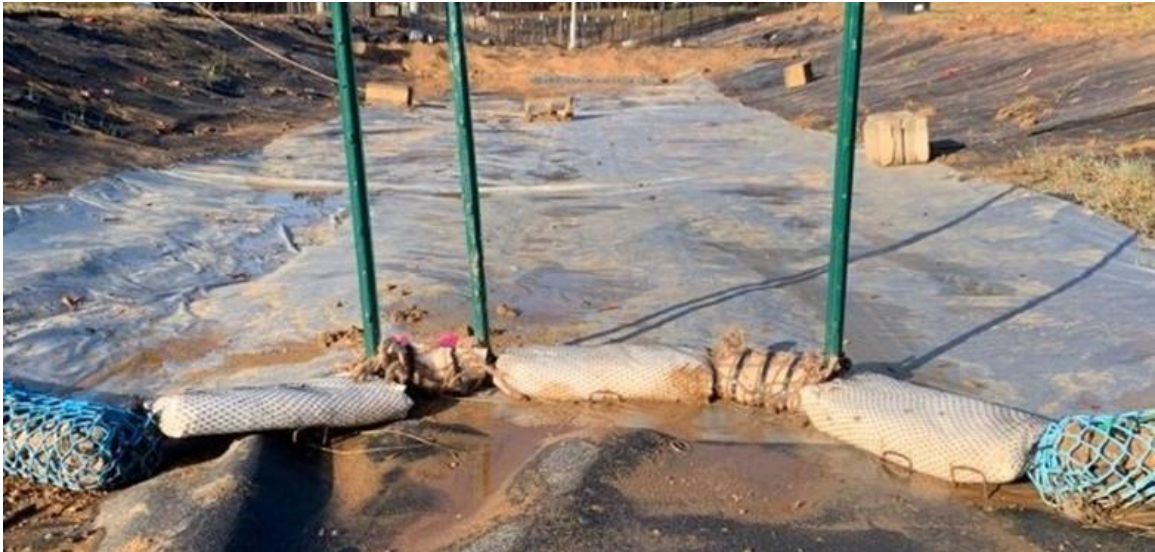
Figure 6-2. Flocculant introduction in testing channel (Schussler 2022)
