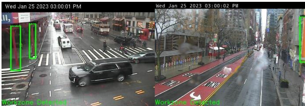
Figure 13. False positive example: Incorrect steam vent detection
