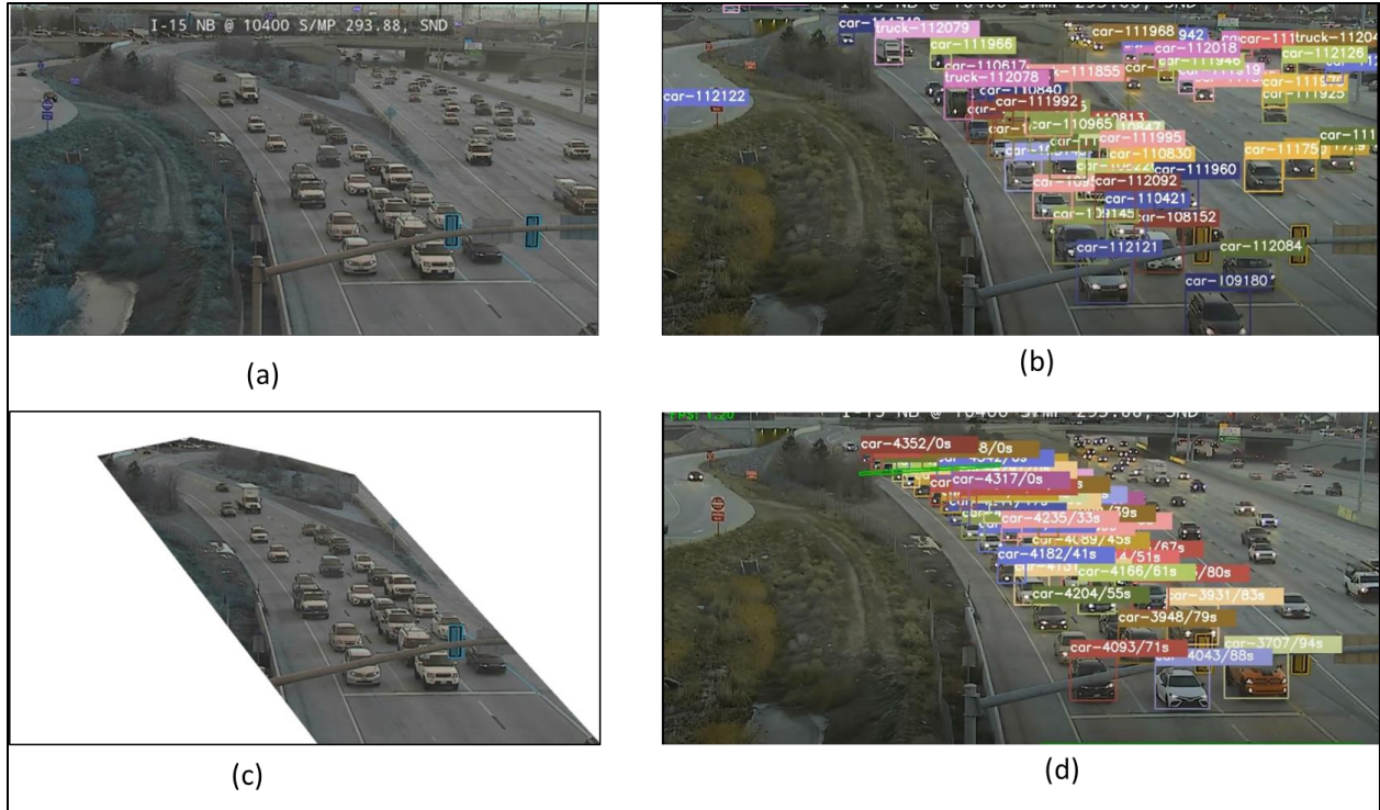
Figure 18: (a) Input Frame without Mask (b) Result for Frame without Mask (c) Input Frame with Mask (d) Result for Frame with Mask
