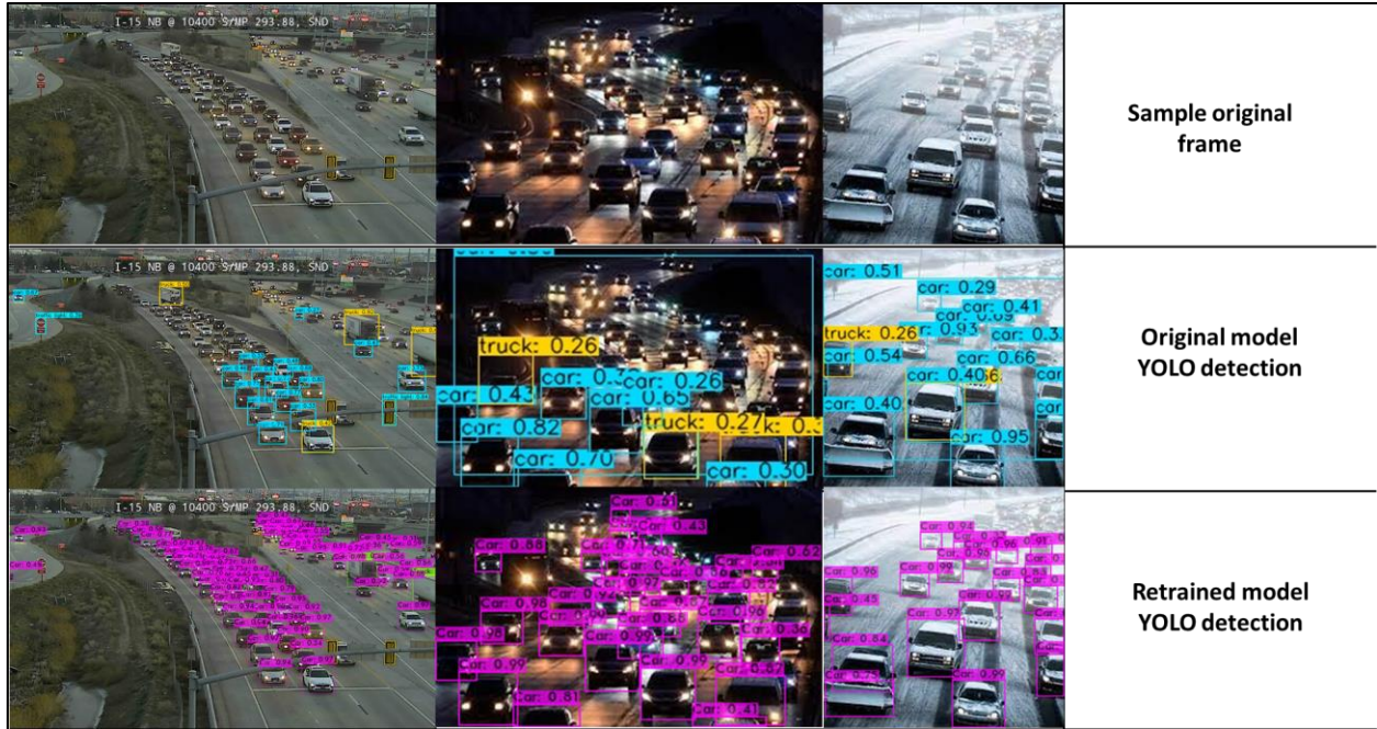
Figure 26: Comparison of Base YOLO Model and Retrained YOLO Model
