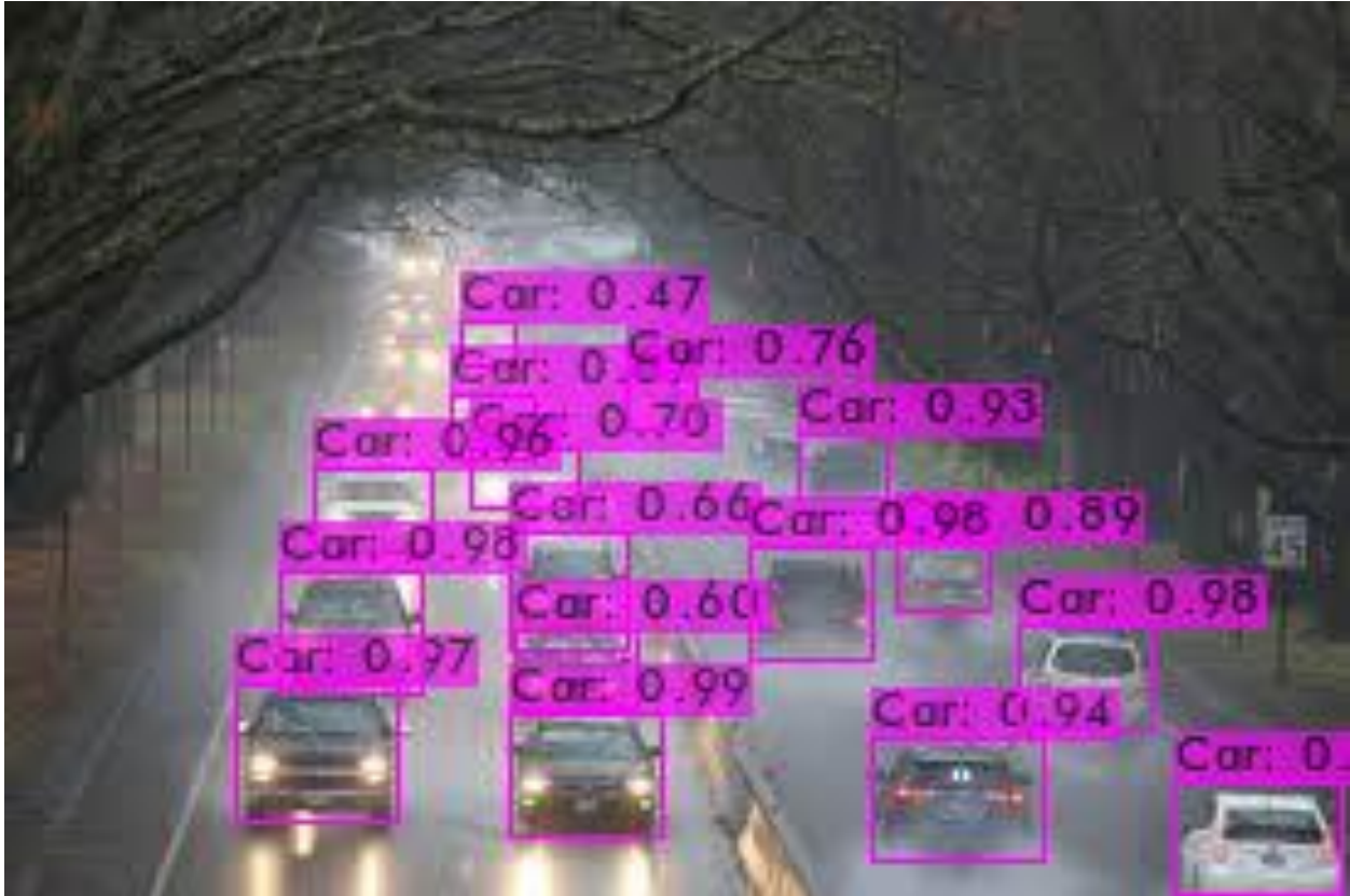
Figure 19: Object Detection and Recognition Using YOLOV4.
