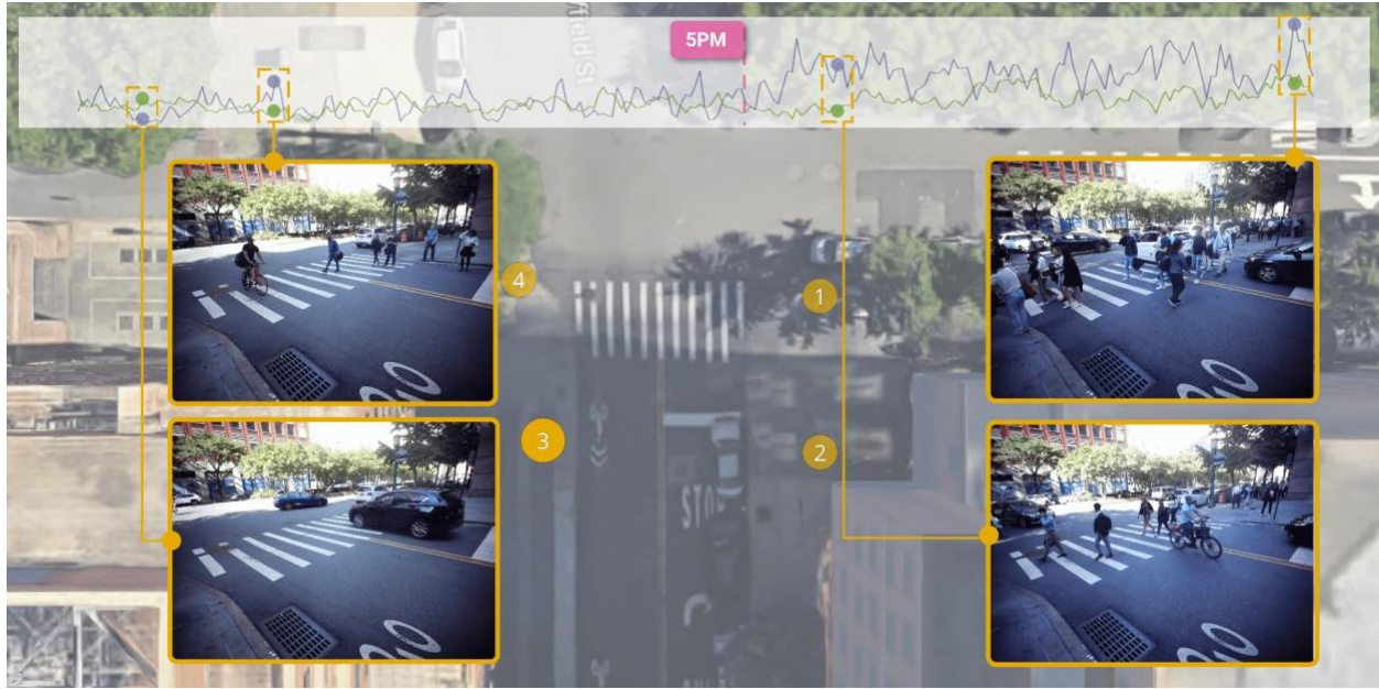
Figure 7. Chase Center intersection occupancy by object type during a recording session in the afternoon. Purple lines representing people and green lines representing cars on the top chart.
