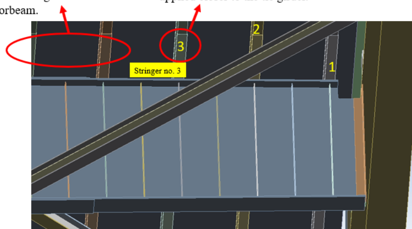
Fig. 7.9 – Load transfer mechanism between stringer 3 and FB19 under pristine and damage scenario 3.
