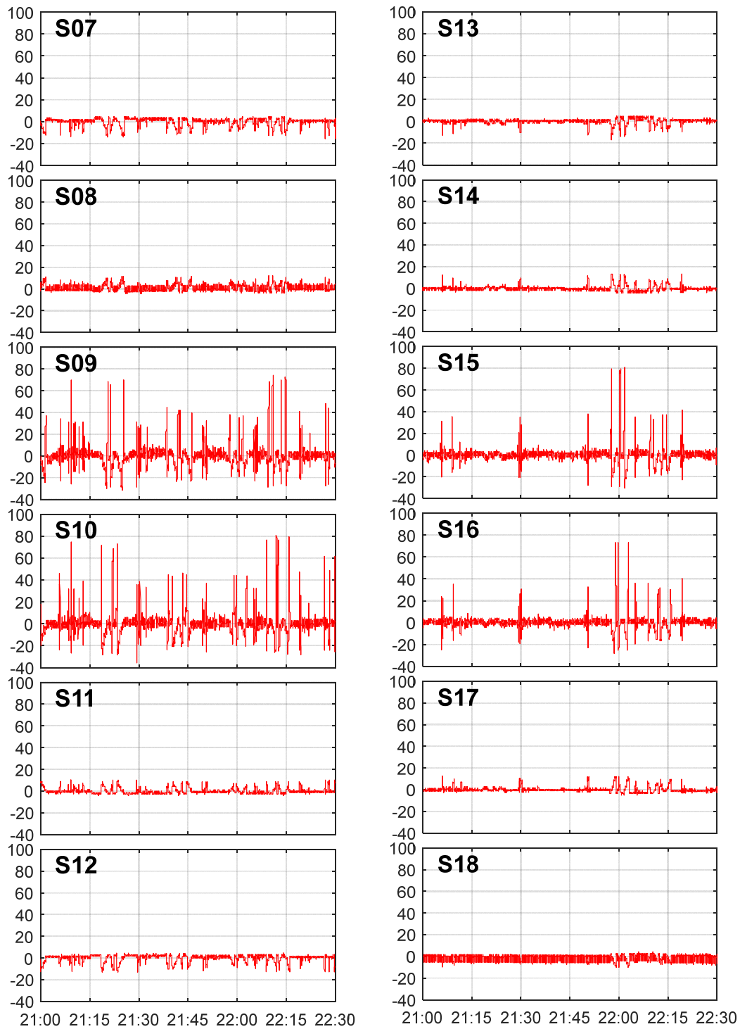
Fig. 5.10 – True strains from gages S07 – S18 extracted from the raw strains stored during the controlled load truck test. (The values on the vertical axes indicate strains and are expressed in microstrains)
