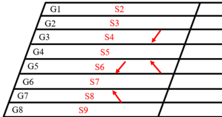
Fig. 6.13 – (a) The shear keys that their contacts with the adjacent beams were changed to “No separation”
