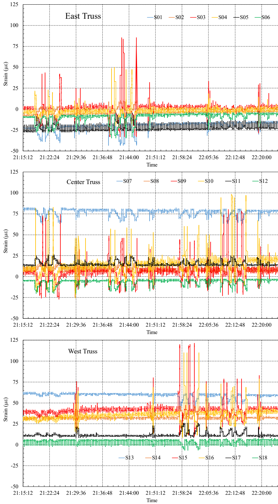
Fig. 5.9 – Strain measured during the truck test performed by Vendor.
