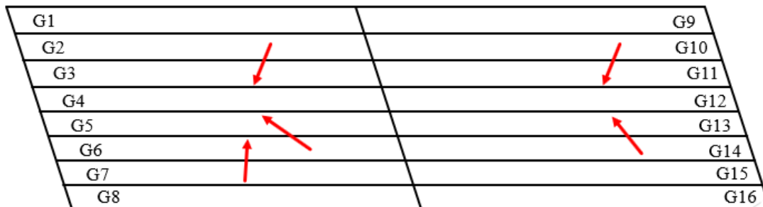
Fig. 6.10 – The shear keys at the Somerset Bridge that their contacts with the adjacent beams were changed to “No separation”
