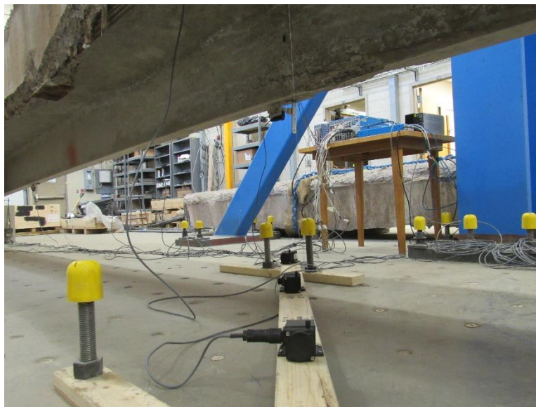
Figure 8.16 – String Pot Installation at Midspan of 50-ft (15.24-m) Long Girder
