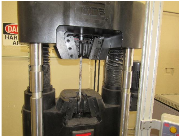
(a) Bar in Tensile Test Machine
