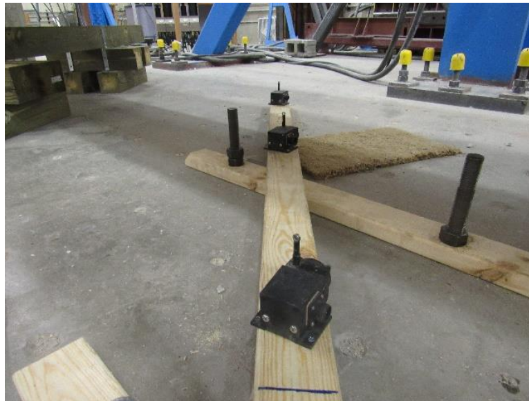
Figure 8.21 – String Pot Installation at Midspan of 30-ft (9.14-m) Long Girder
