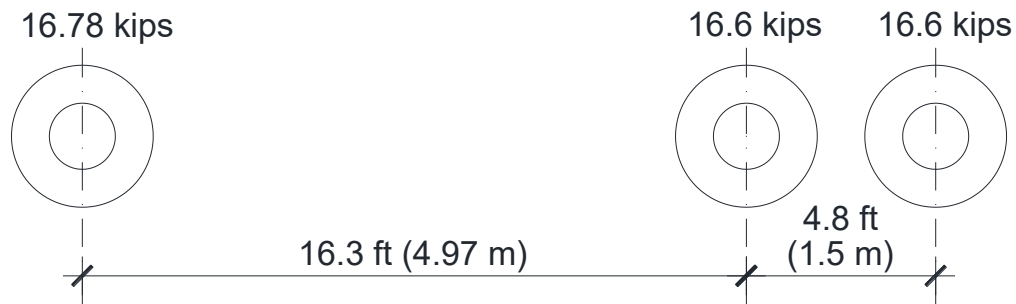
(c) Test Truck Axle Weight Distribution
