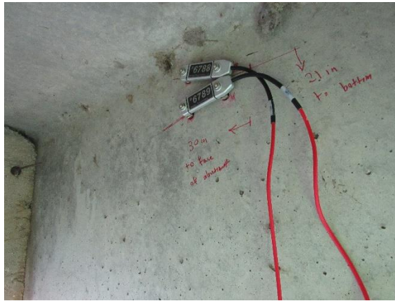
(a) Lines for Gauge Installation
