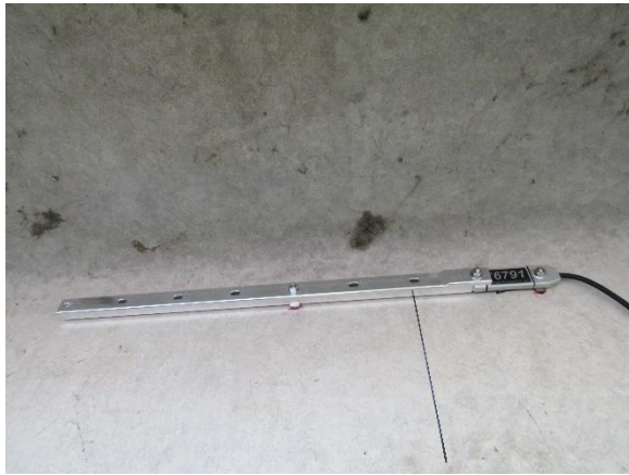
(a) Installation of Strain Gauges with Extension
