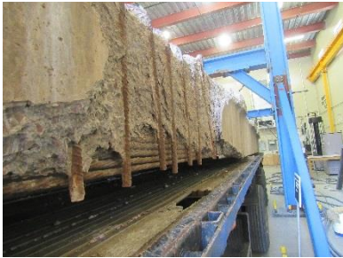
(p) Stem Exposure of Strand (CS-2)
