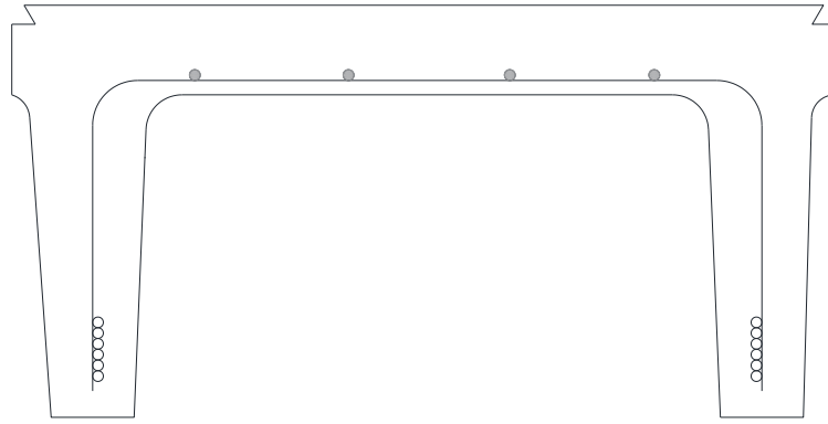
Figure 9.1 – Stem Cover Deterioration with Condition State 1 equivalent to Undamaged Section
