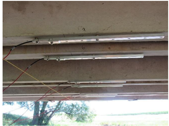
(b) Strain Gauges at Stem Bottom Face
