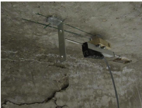
(c) LVDT underneath Flange for Rotations
