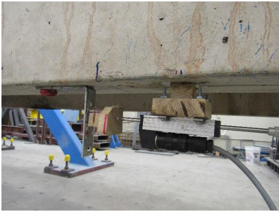
(a) LVDT as Concrete Strain Gauge
