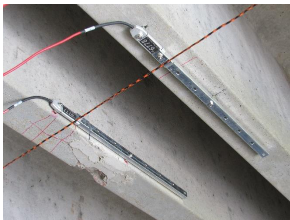
(c) Strain Gauges on Stem Side due to Damage
