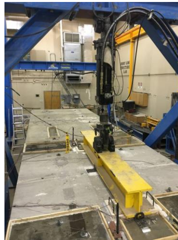
(b) Two-Point Loads in Phase II
