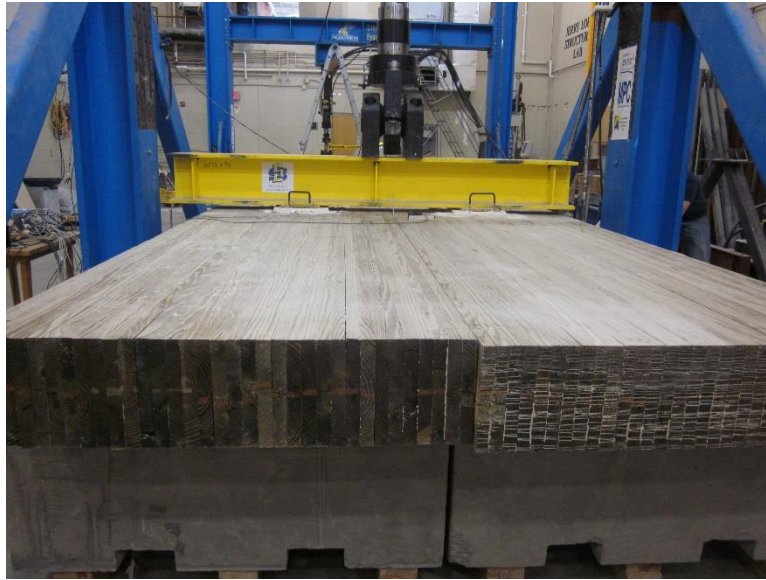
Figure 6.71: Strength Test Setup for Glulam Timber Slab Bridge
