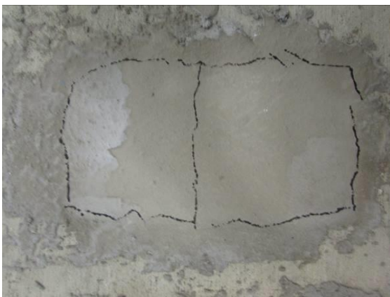
(c) Latex Modified Concrete at 125,000 Cycle
