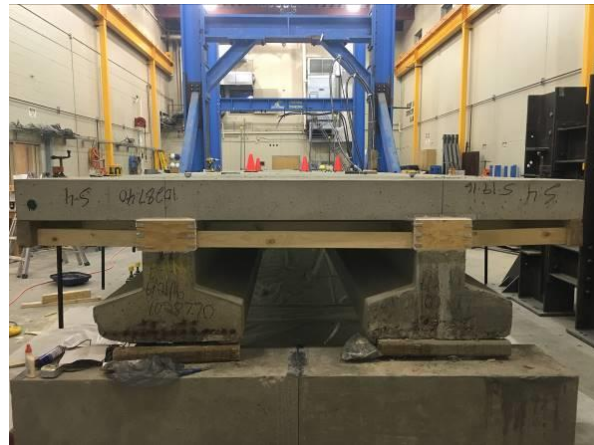
Figure 6.12 Grout Haunch Region Formwork
