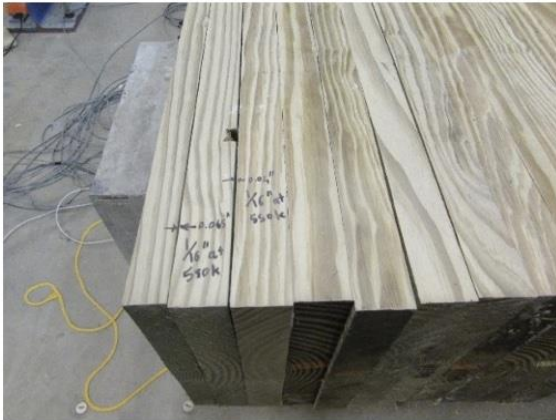
(c) Separation of Lamination after 550k Cycles at Southwest Support
