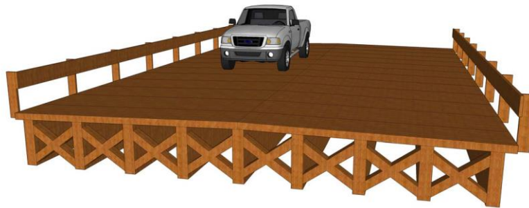
Figure A.10: Typical Glulam Timber Girder Bridge
