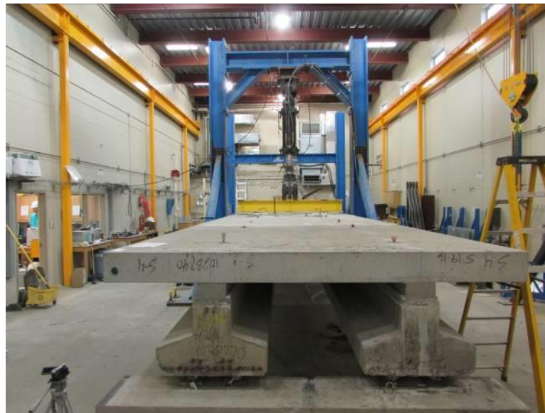
Figure 6.16: Ultimate Test Setup for the Precast Bridge Specimen
