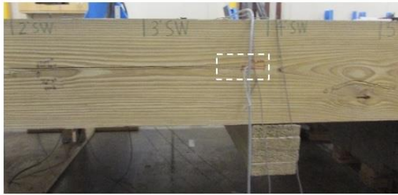
(a) Crack Growth after 550k Cycles – Elevation View
