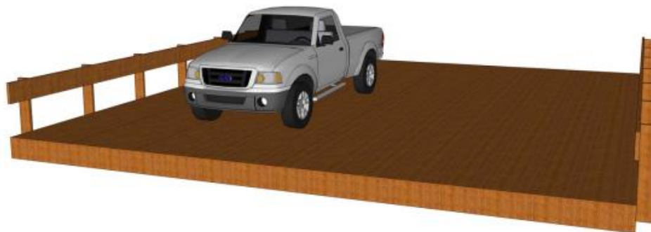
Figure A.18: Typical Glulam Timber Slab Bridge
