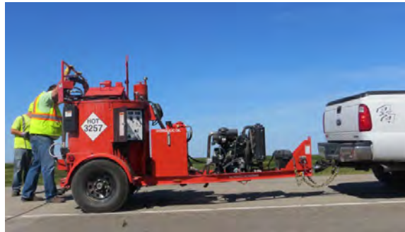
Figure 19 Kettle used for Crafcro, Inc. crack sealant products
