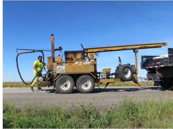
Figure 18 Kettles used by Asphalt Technologies Corp. for heating and installing crack sealants
