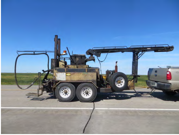
Figure 18 Kettles used by Asphalt Technologies Corp. for heating and installing crack sealants
