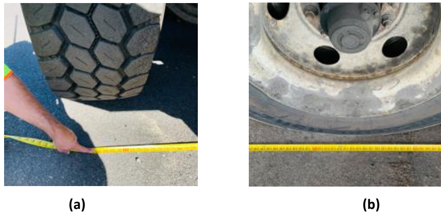
Figure 10: Axle Spacing Measurements; (a) wheel width, and (b) axle spacing
