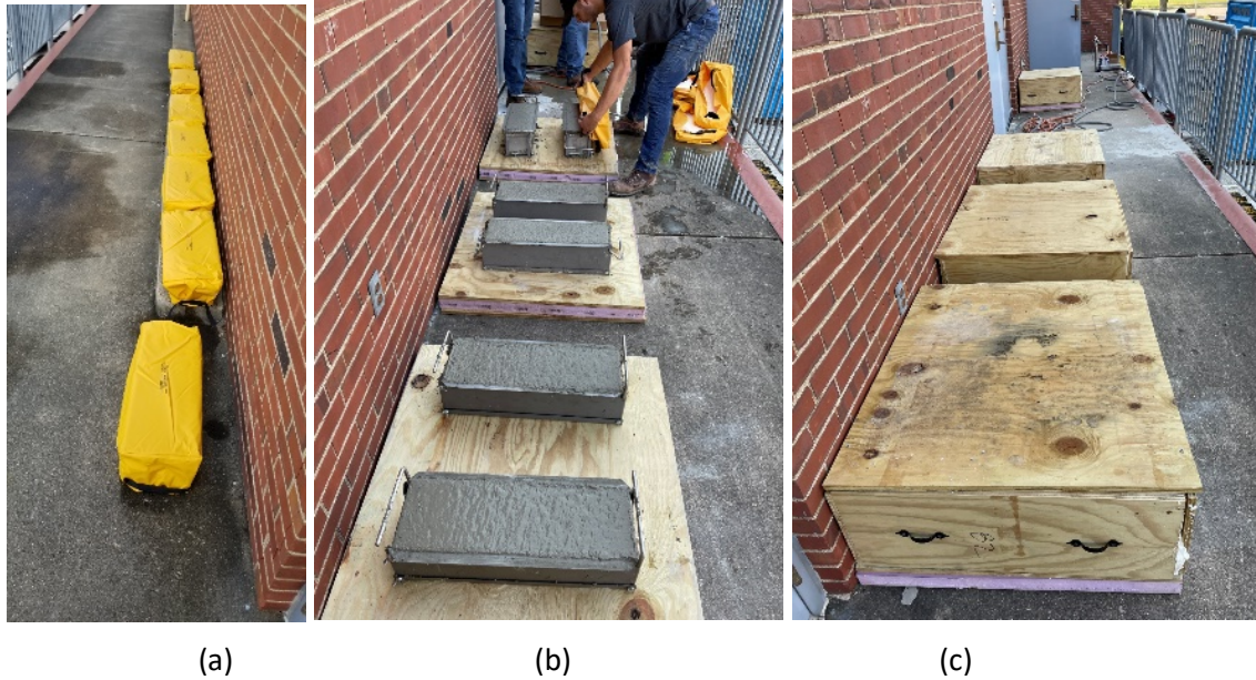
Figure 5. Photos. Beams under curing for (a) Method #B1—October 2021, (b) Method #B2 without a top lid, (c) Method #B2 with a top lid.
