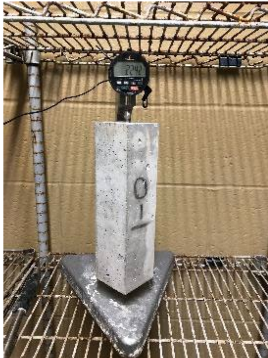
Figure 16: ASTM C157 Drying Shrinkage Length Measurement
