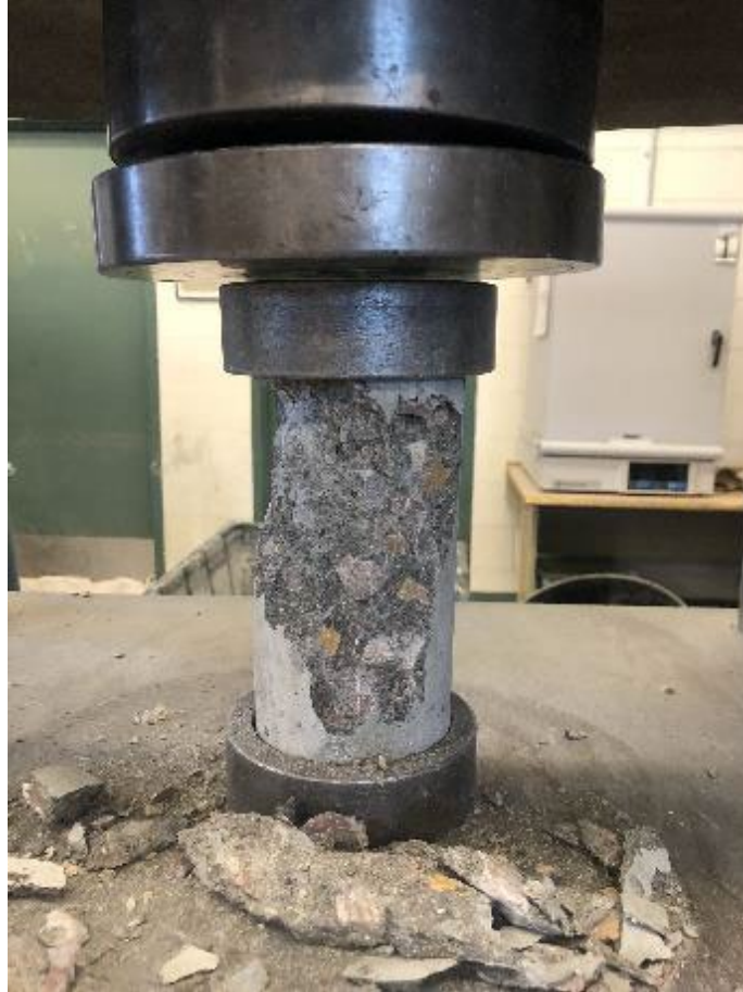
Figure 12: 4" x 8"-Cylinder Mold Failure During Compression Testing
