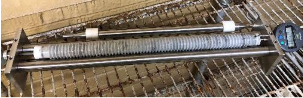
Figure 15: Dilatometer Bench Used to Measure Length of Paste and Mortar Samples
