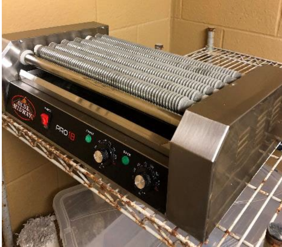
Figure 14: Machine Used to Rotate Samples Until Final Set was Reached
