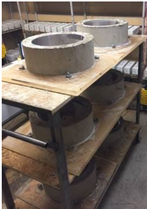
Figure 17: ASTM C1581 Restrained Shrinkage Ring Test Setup
