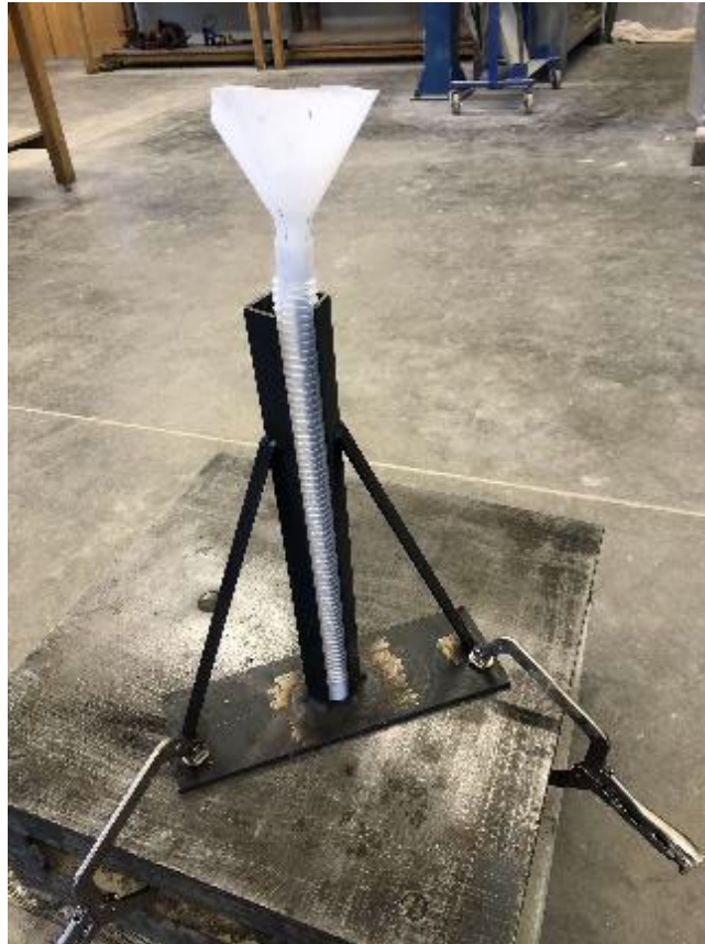
Figure 13: Support Fixture for Filling Corrugated Tube Molds
