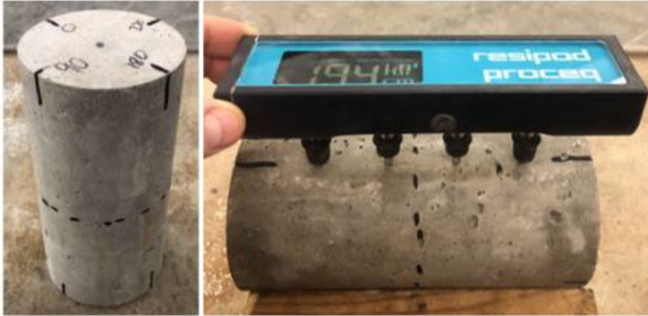
Figure 11: Electrical Resistivity Meter and Sample Marking
