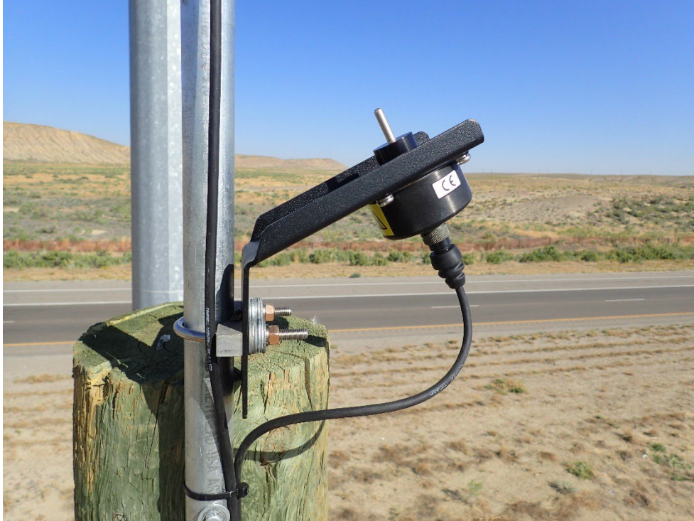
Figure 16. Freezing rain sensor and mounting kit
