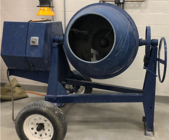
Figure 3-1: Concrete mixer used
