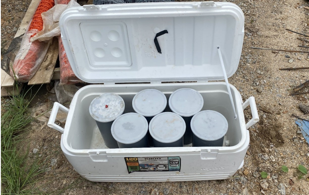
Figure 6-29: Jobsite 4 NSIC Curing Box
