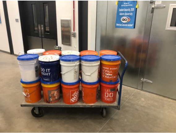
Figure 3-2: Concrete materials before entering environmental chamber
