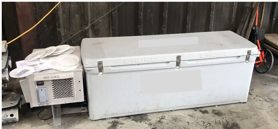
Figure 6-1: Jobsite 1–Contractor Curing Box
