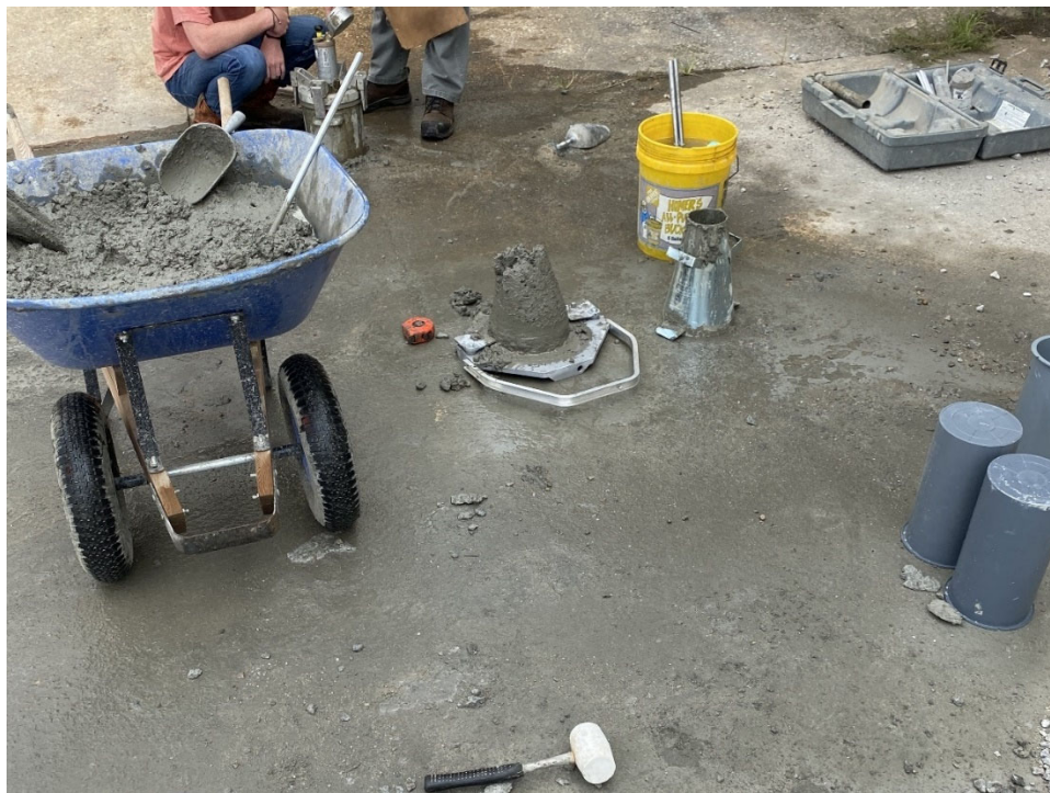
Figure 6-8: ALDOT Technicians Performing Fresh Concrete Property Tests
