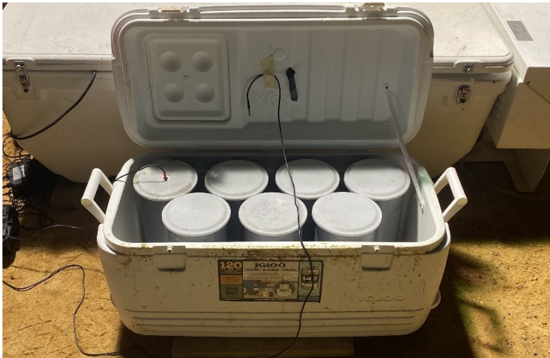
Figure 6-22: Jobsite 3 NSIC Curing Box
