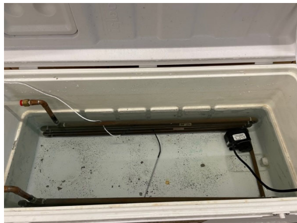
Figure 3-5: Initial Curing Tank
