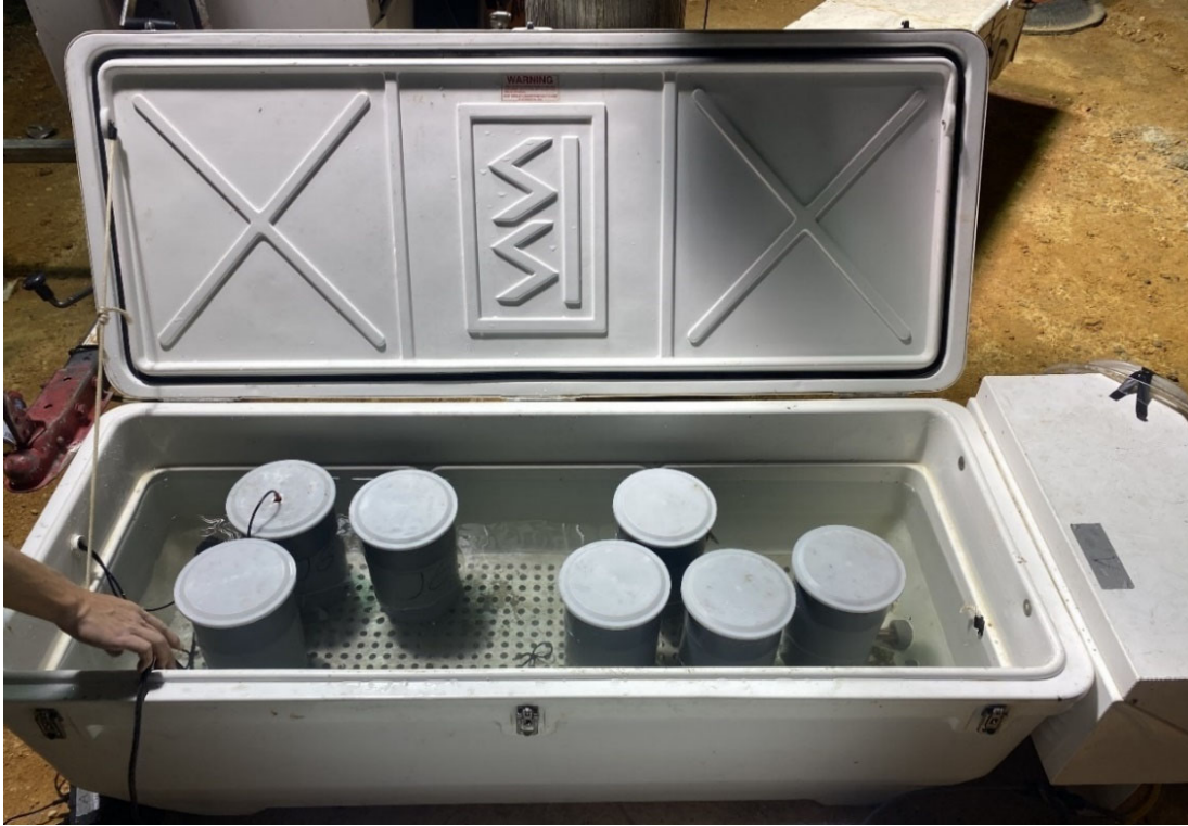
Figure 6-21: Jobsite 3 SIC Curing Box
