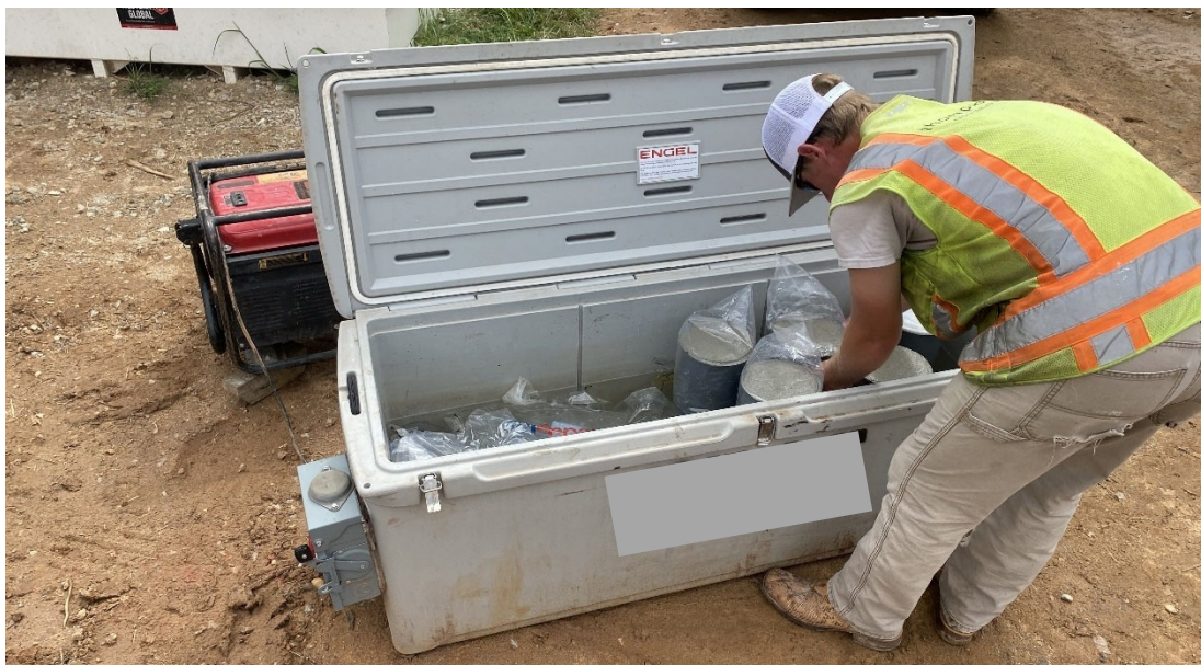
Figure 6-27: Jobsite 4 Contractor Curing Box
