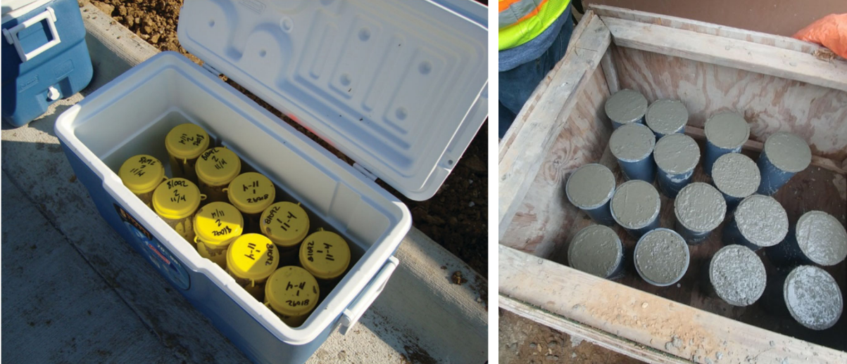
Figure 1-3: Improper jobsite cylinder curing boxes that do not meet ALDOT requirements: (Left) Coolers without temperature control and (Right) Plywood box without temperature control (Source: NRMCA)
