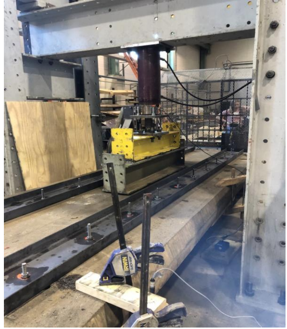
Figure 3.4 Strengthened slab test setup with two steel channels on top.
