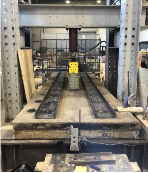
Figure 3.4 Strengthened slab test setup with two steel channels on top.
