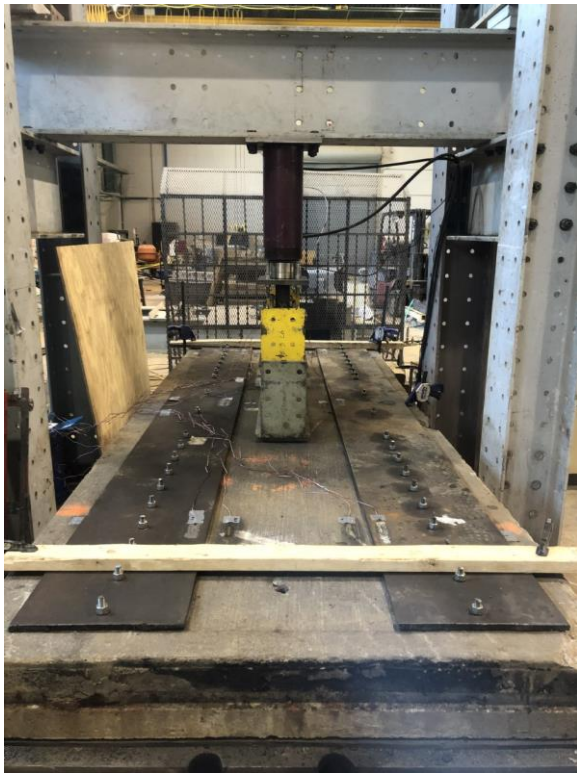
Figure 3.5 Strengthened slab test setup with two plates on top.
