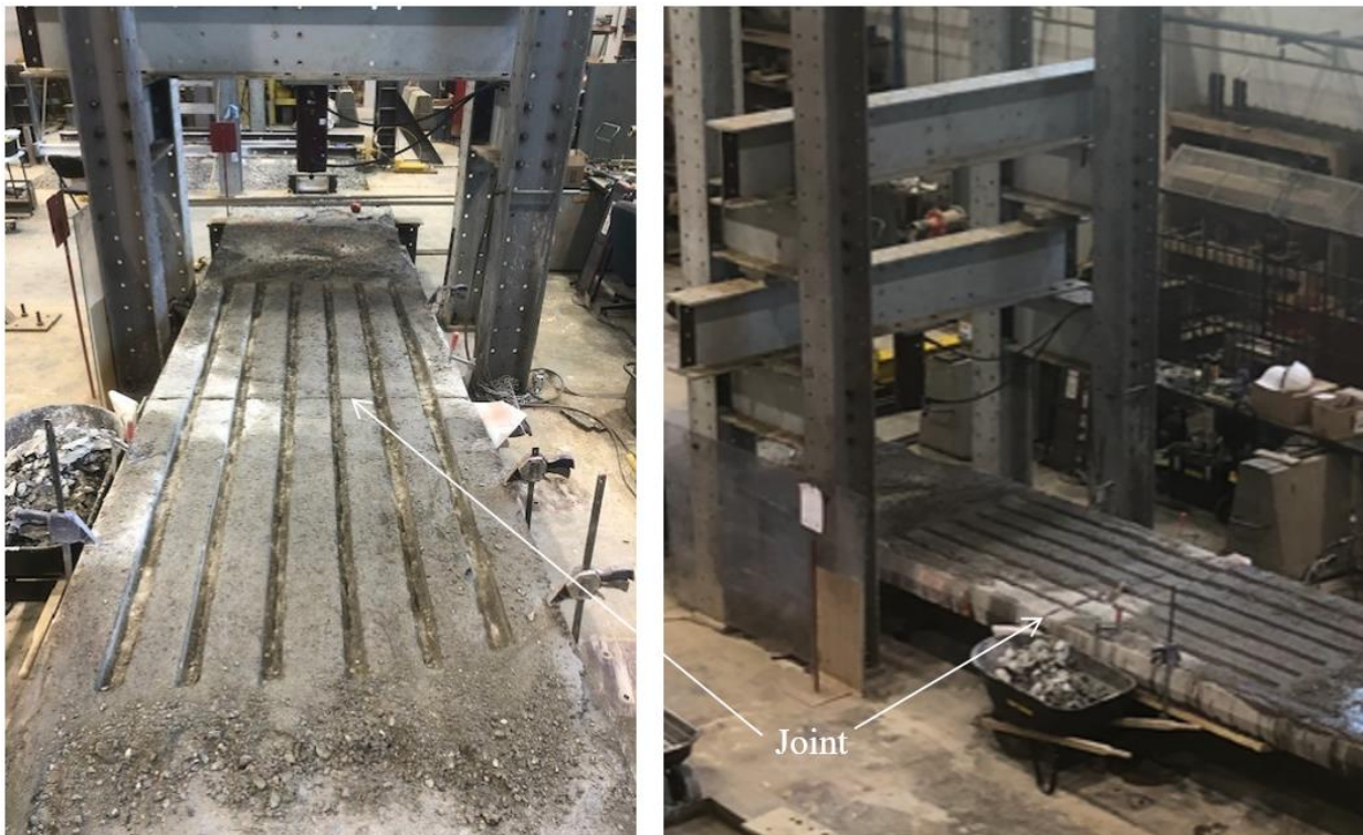
Figure 3.17 Concrete grooves cut into slab and over joint
