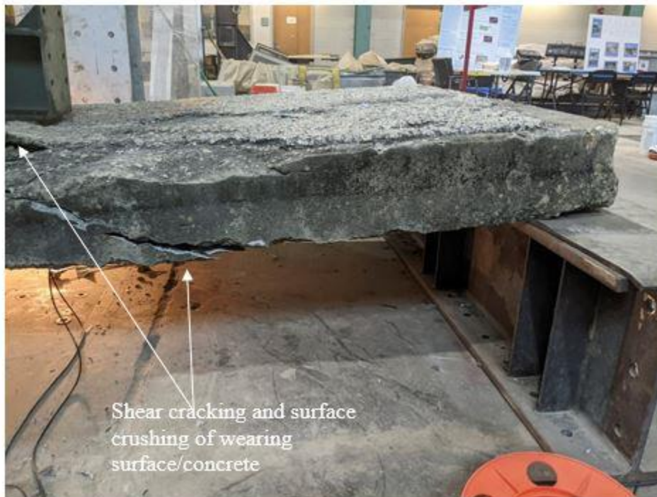
Figure 4.9 Failure mode of NSM test
