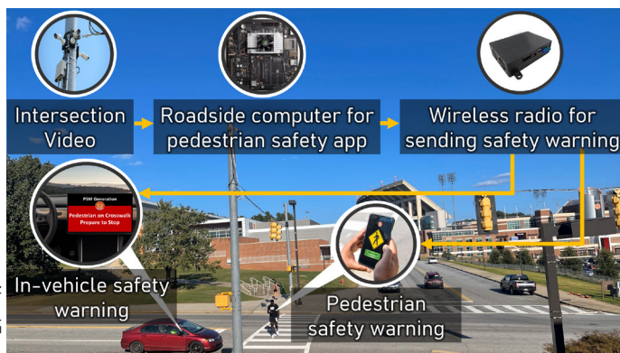
Figure 1. System components for generating vision-based pedestrian safety warning messages.
