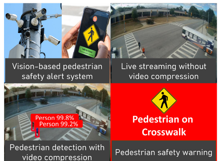
Figure 2. Pedestrian safety alert system using dynamic lossy video compression.
