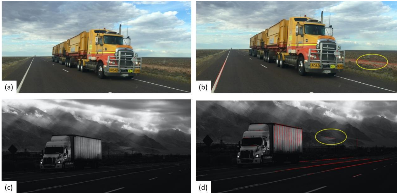
Figure 11. (a) Truck Image on Highway, (b) line segments filtered from [a], (c) Truck Image at Night on Highway, (d) line segments filtered from [c].
