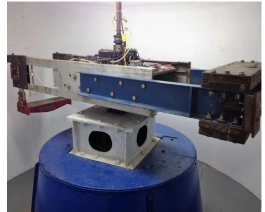
A centrifuge test set up shows the various parts of the small-scale load test model.
