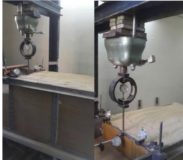
Figure 0-24. Pictures of the sheet pile under axial loading (Azzam & Elwakil, 2017)
