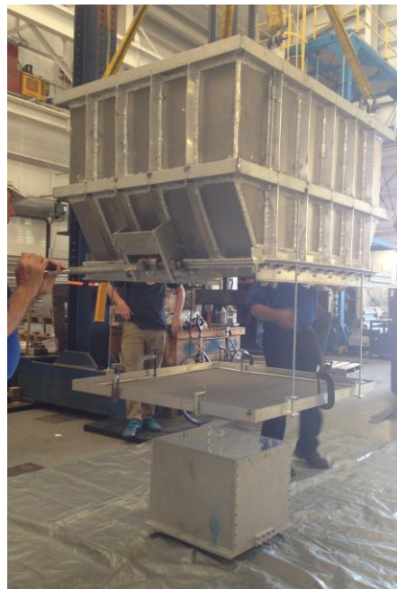
Figure 3-14. Pluviator used for constructing the soil profile
