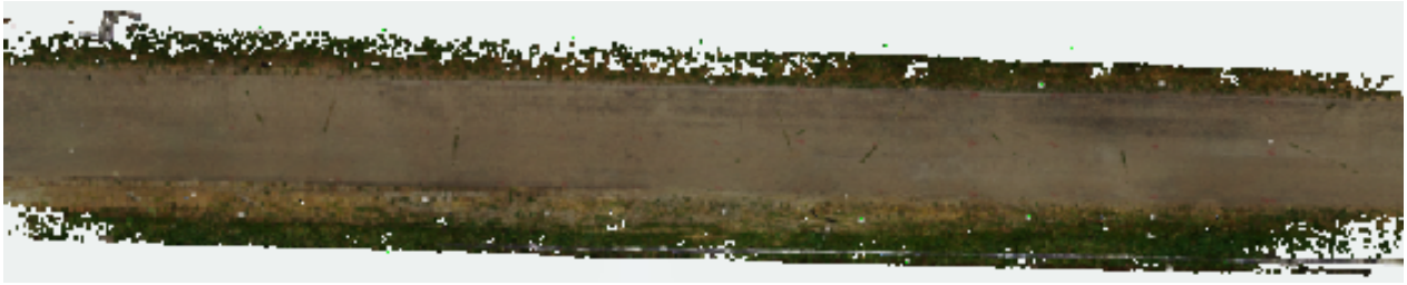
Figure 7. Lidar Point Cloud of Stenner Road Segment
