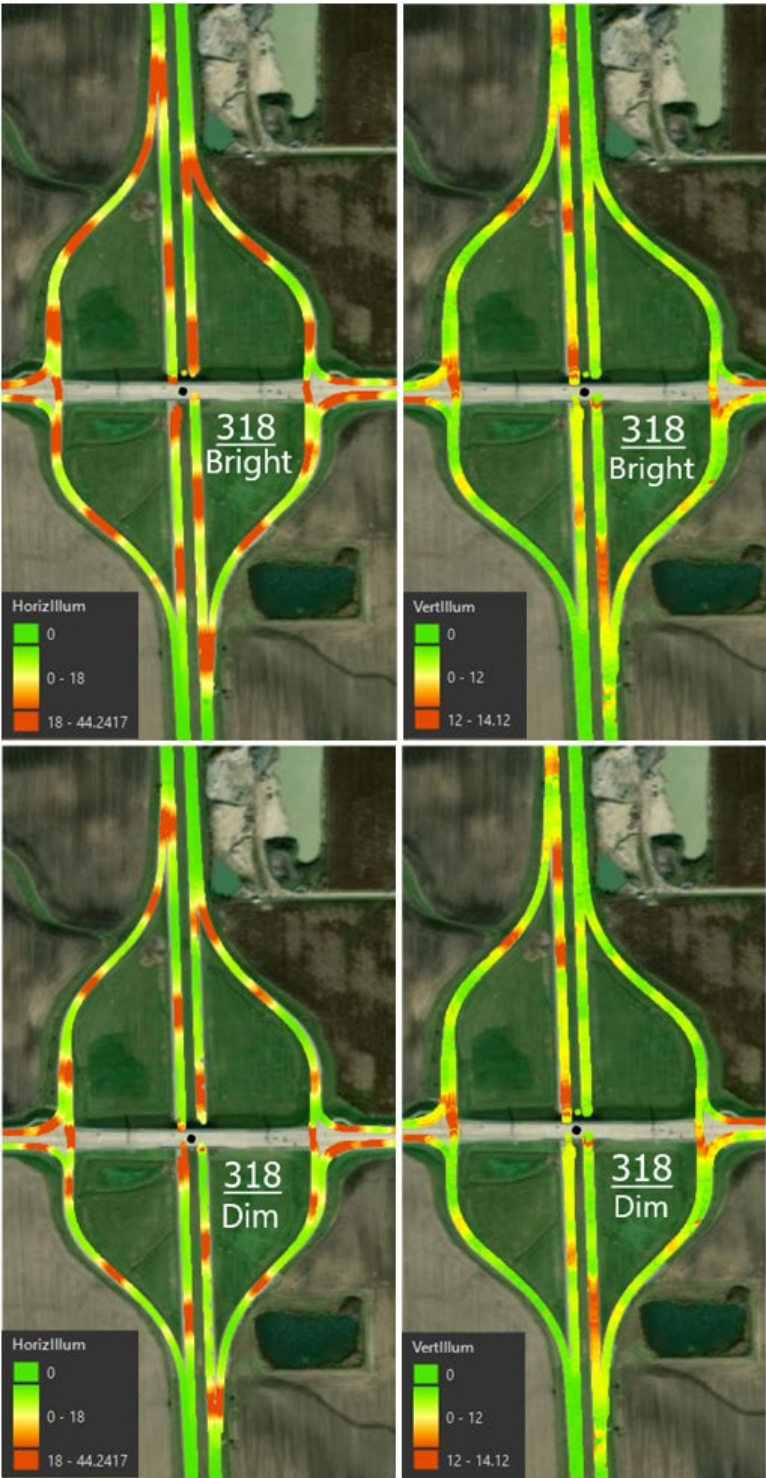
Figure 13. Photo. Horizontal illuminance (left) and vertical illuminance (right) heatmaps for Interchange 318 (High-Mast) while at full brightness (top) and dimmed to 50% (bottom).
