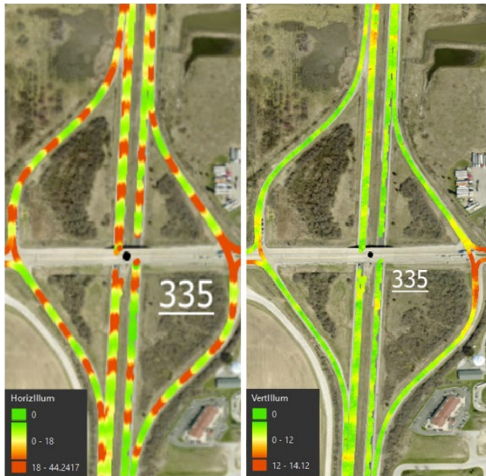
Figure 16. Photo. Horizontal illuminance (left) and vertical illuminance (right) heatmaps for Interchange 335 (conventional).
