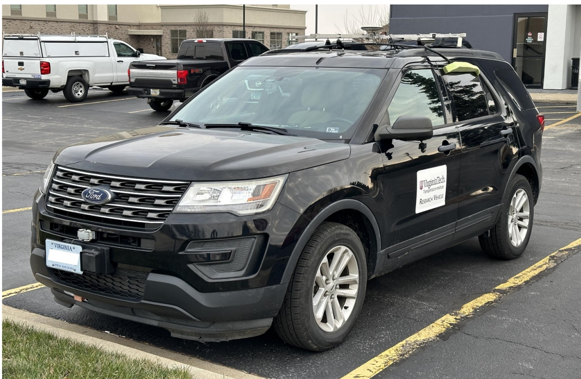
Figure 5. Photo. Experimental vehicle (2017 Ford Explorer) with RLMMS deployed.
