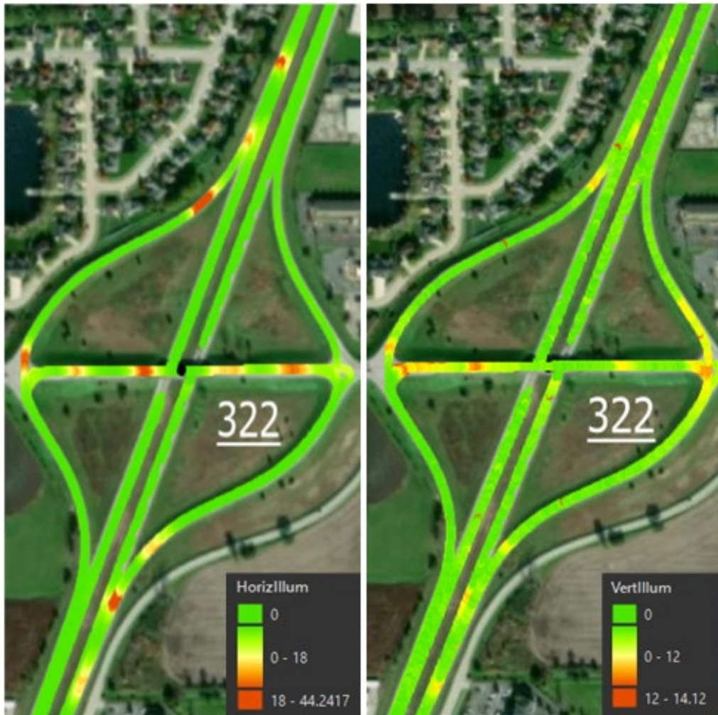
Figure 14. Photo. Horizontal illuminance (left) and vertical illuminance (right) heatmaps for Interchange 322 (conventional exit only).
