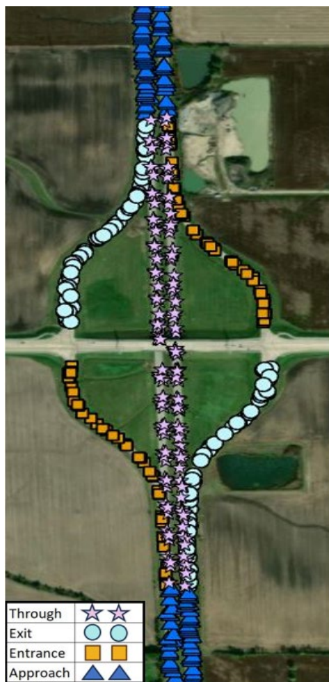
Figure 6. Photo. Interchange segment type selection with symbol indicating the allocation of data.
