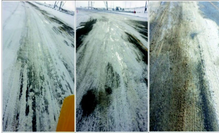
Figure E6. Sand applied on icy road surface at IRRF test road in Canada (Hayhoe, 1984).
