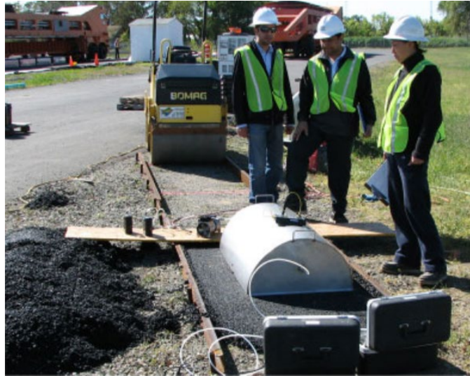
Figure E7. Measuring VOCs using the transportable flux chamber (Jones et al., 2012b).
