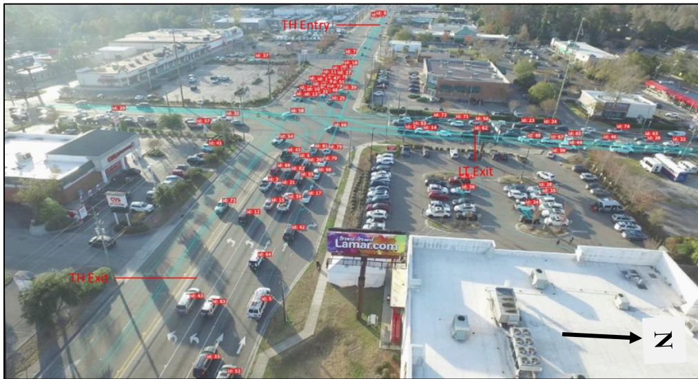
Figure 5-4: Processed Drone Video for Oleander Dr. and S. College Rd Showing Vehicle ID's and Entry and Exit Sensor Locations for EB-TH and EB-L Movements
