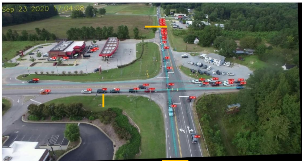
Figure 3-3: Processed Drone Video Showing Vehicle ID's and Sensor Locations
