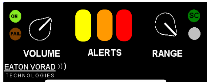
Figure 20. Eaton® VORAD® driver display unit for the forward sensor.
