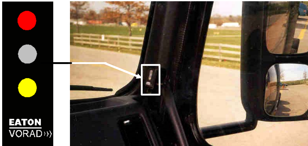
Figure 22. Eaton® VORAD® driver display unit for the side sensor.
