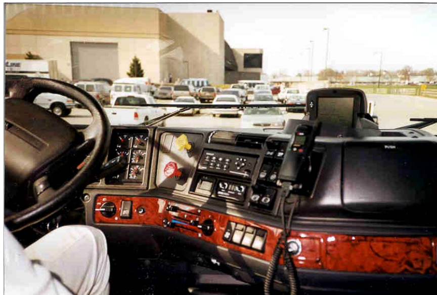
Figure 21. Eaton® VORAD® forward sensor driver display unit mounted in the dashboard. (Note: This picture was not taken on a U.S. Xpress unit. The DDU is on the dashboard in the U.S. Xpress trucks.)
