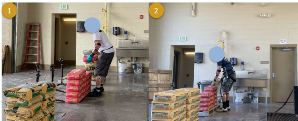
Figure 8.9 Lifting 31.5-pound bags, 50-pound bags, and 80-pound bags: (1) without back exoskeleton and (2) with back exoskeleton.
