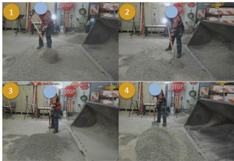
Figure 8.11 Shoveling with (1) regular shovel, (2) back exoskeleton, (3) ergonomic handle, and (4) both ergonomic handle and back exoskeleton.
