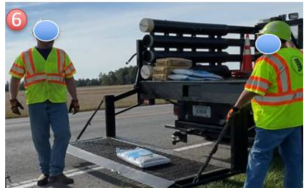
Figure 7.25 Pulling deer step six—lowering down the liftgate to let a worker step off.
