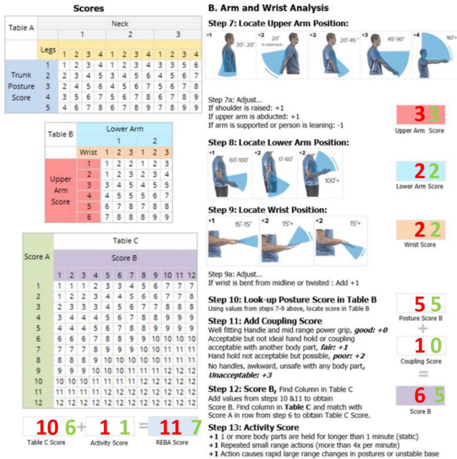
Figure 8.18 Part B arm and wrist analysis of REBA for evaluating the risk of musculoskeletal disorders associated with tasks (Middlesworth, 2023).
