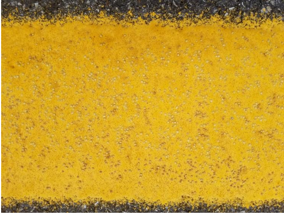
Figure 6. Yellow All-Weather Marking with Discolored Wet-Weather Optics.
