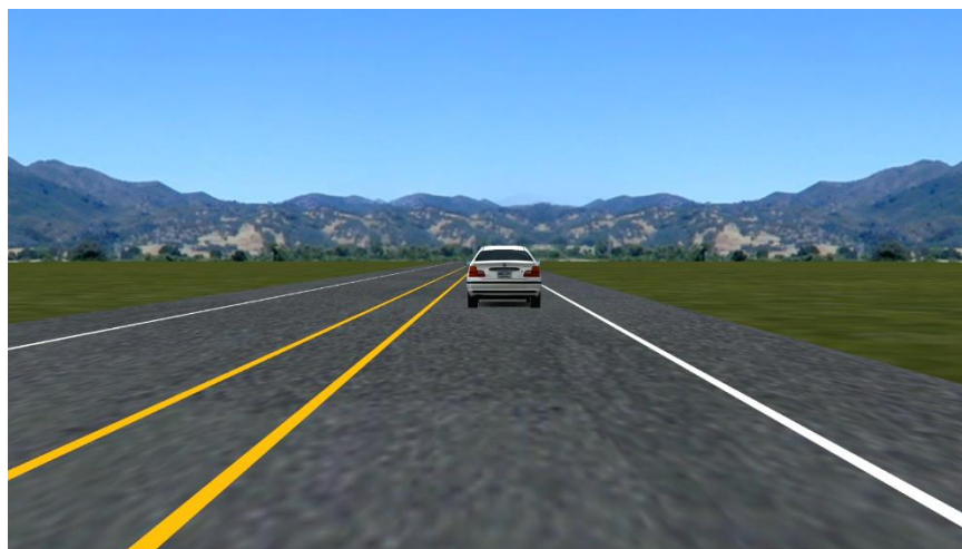
Figure 10. Experimental 4-ft Centerline Buffer Image—Treatment 3.
