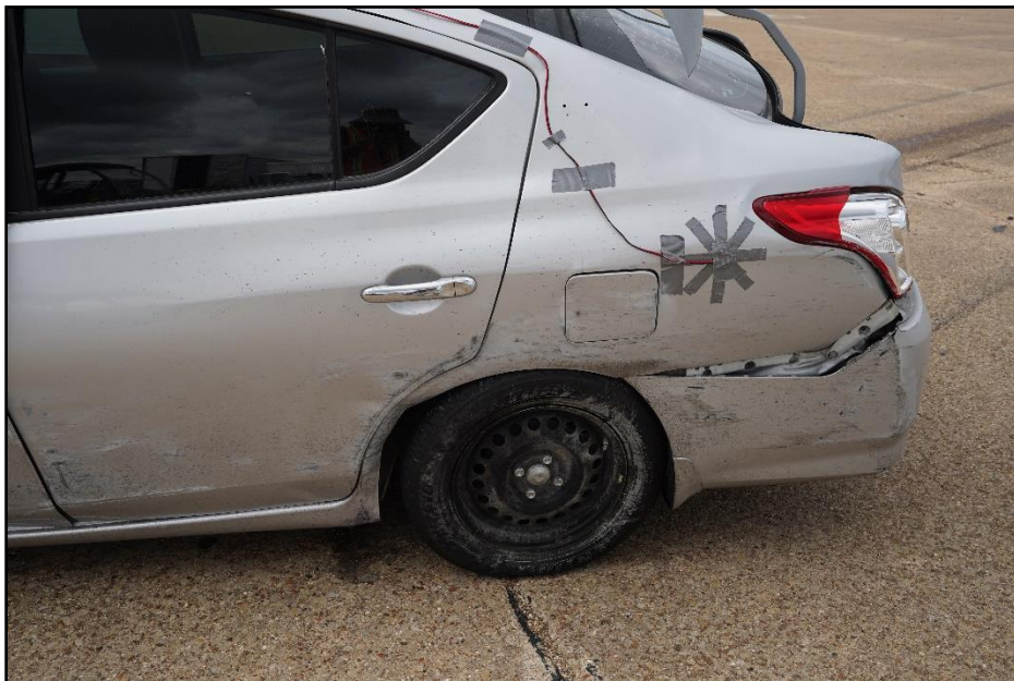
Figure 7.8. Rear Impact Side of Test Vehicle after Test 440862-03-4.
