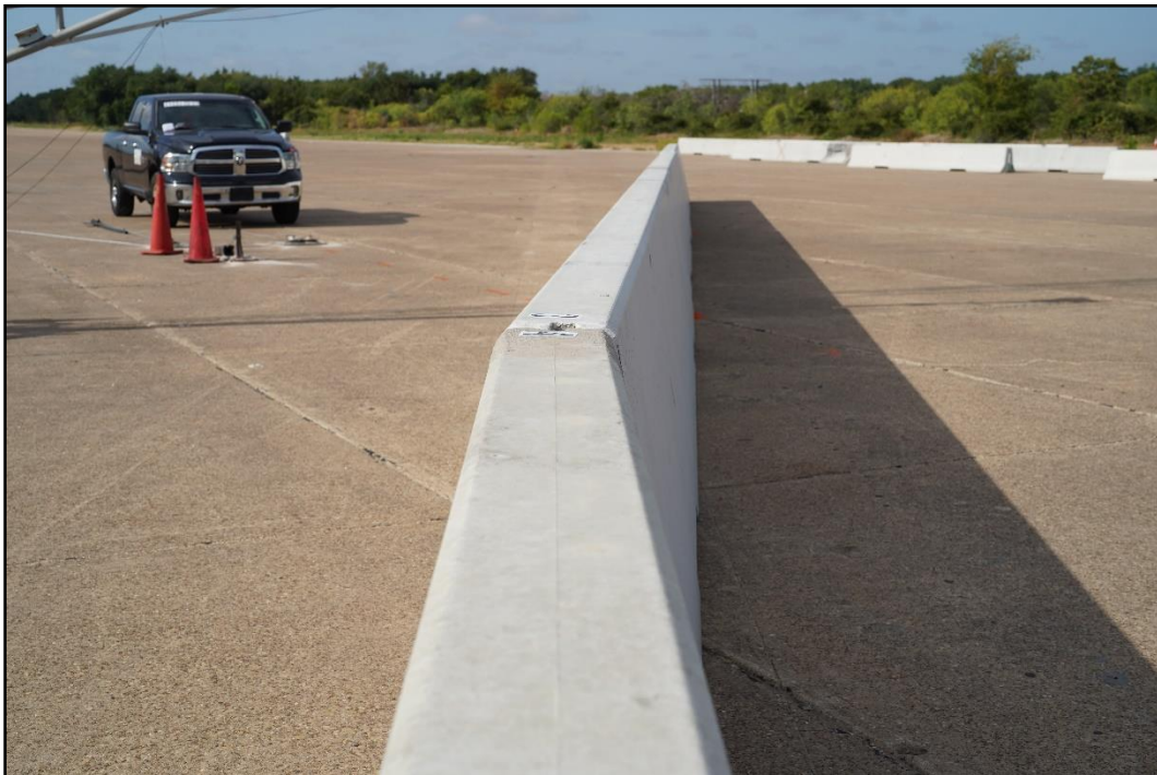
Figure 3.7. Downstream View in Line with the Length of Need of the Flared Single-Slope Portable Concrete Barriers prior to Testing.
