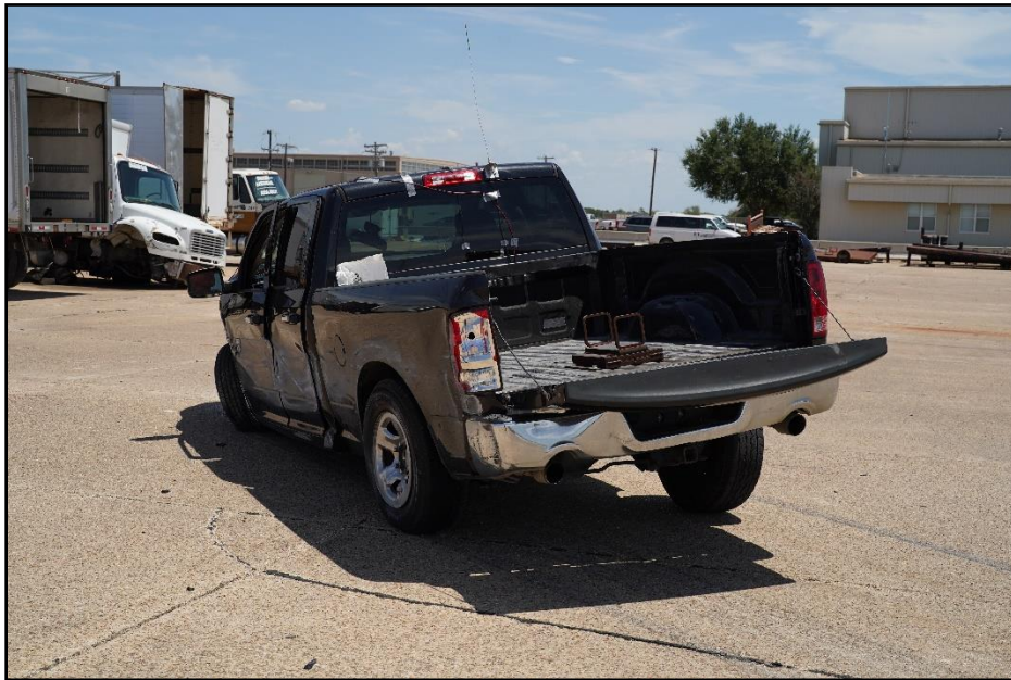
Figure 6.8. Rear Impact Side of Test Vehicle after Test 440862-03-3.
