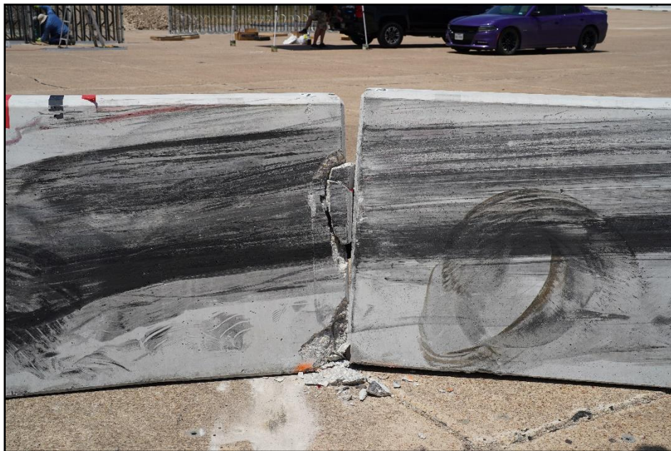
Figure 6.6. Flared Single-Slope Portable Concrete Barriers after Test at Impact Location, Test 440862-03-3.
