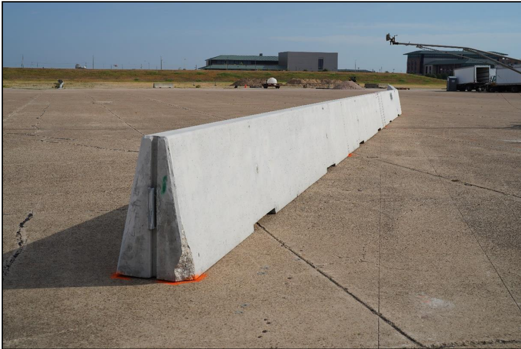
Figure 3.2. Flared Single-Slope Portable Concrete Barriers Prior to Testing.
