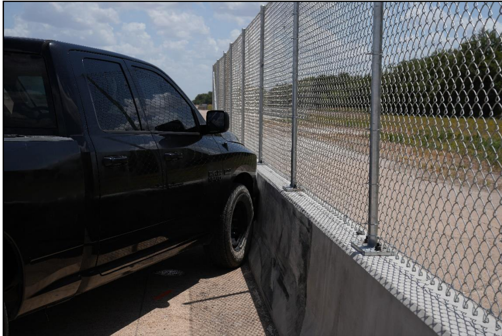
Figure 9.3. Chain-Link Fence on F-Shape Barrier/Test Vehicle Impact Location, Test 440822-01-5.
