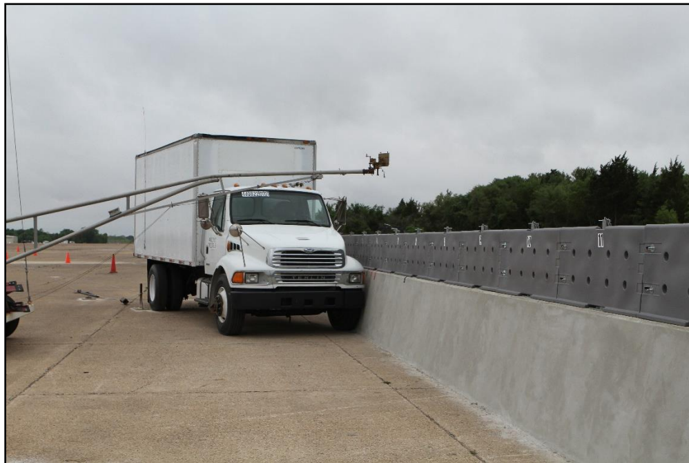
Figure 5.2. Armorcast® Gawk Screen on Single-Slope Barrier/Test Vehicle Geometrics for Test 440822-01-1.
