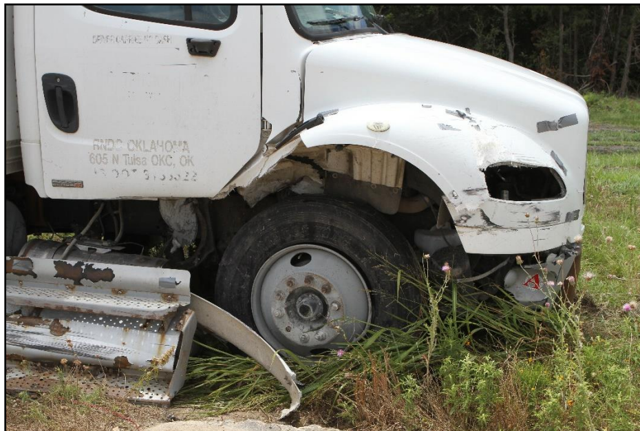
Figure 6.8. Impact Side of Test Vehicle after Test 440822-01-2.
