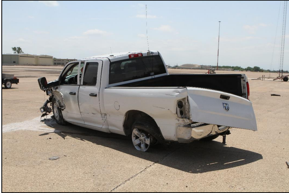
Figure 7.9. Rear Impact Side of Test Vehicle after Test 440822-01-3.
