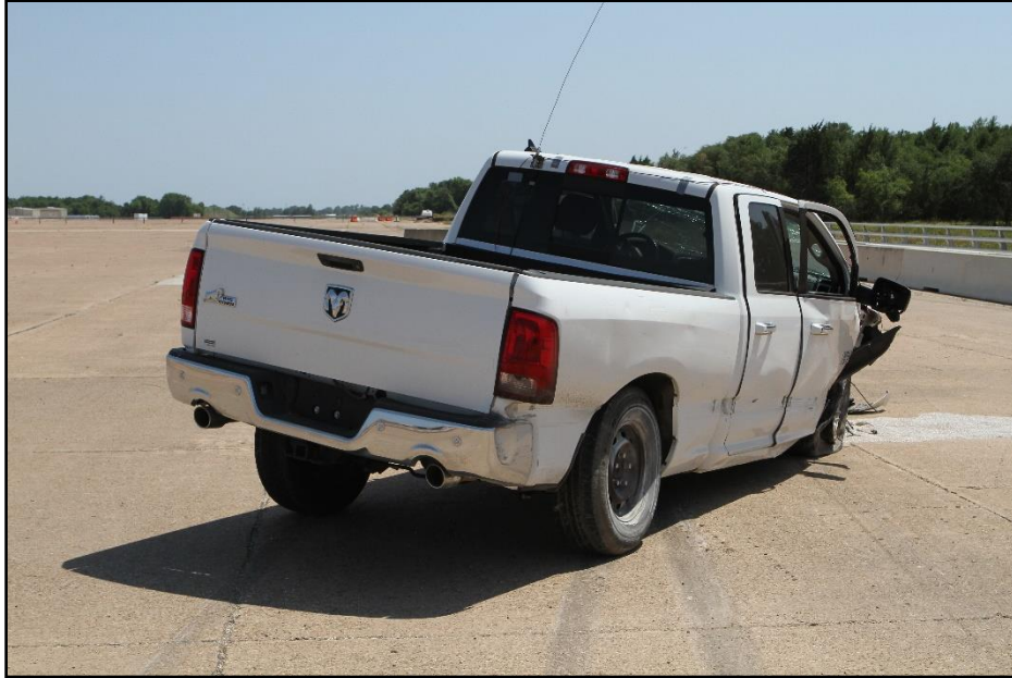
Figure 8.9. Rear Impact Side of Test Vehicle after Test 440822-01-4.
