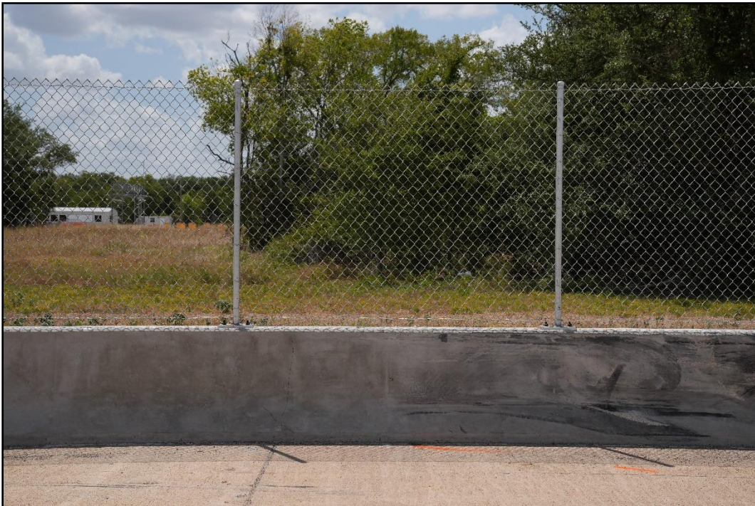
Figure 2.15. Impact Side of Chain-Link Fence on F-Shape Barrier prior to Testing.
