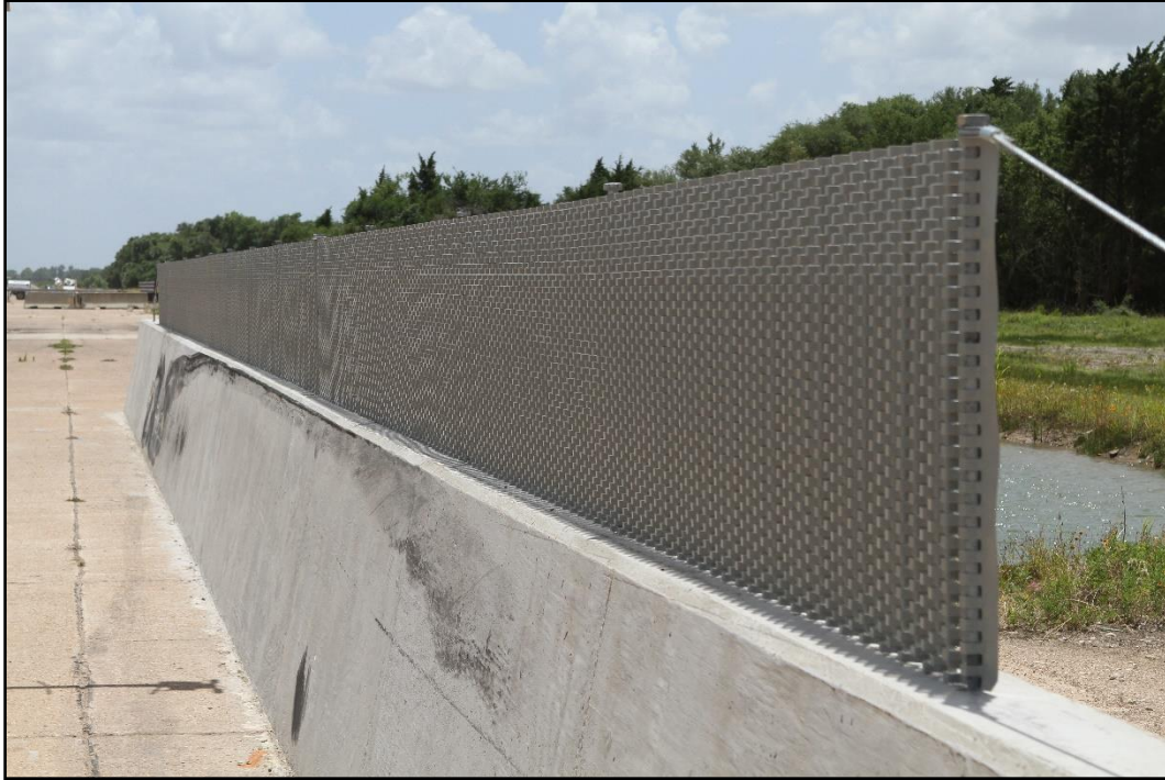
Figure 2.8. Impact Side of Screen-Safe® Glare Screen on Single-Slope Barrier prior to Testing.
