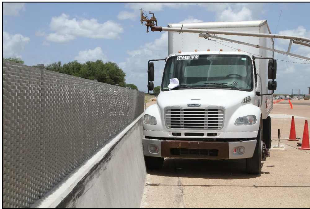
Figure 6.2. Screen-Safe® Glare Screen on Single-Slope Barrier/Test Vehicle Geometrics for Test 440822-01-2.
