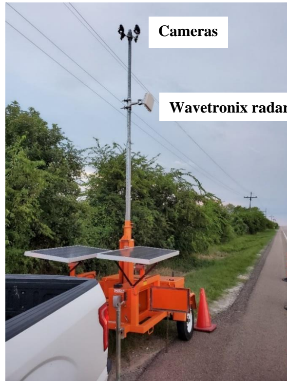
Figure 5. TTI Portable Video Data Collection Equipment.
