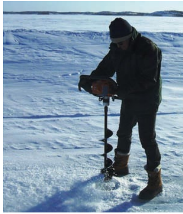
An auger being used to drill a Test Hole through the ice 1
