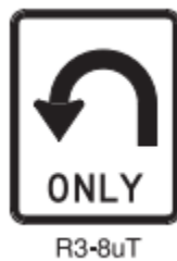
Source: TMUTCD 2014 Edition, Figure 2B-4, page 60. Figure 135. Example of U-Turn Turnaround Only Sign Included in the TMUTCD (59).
