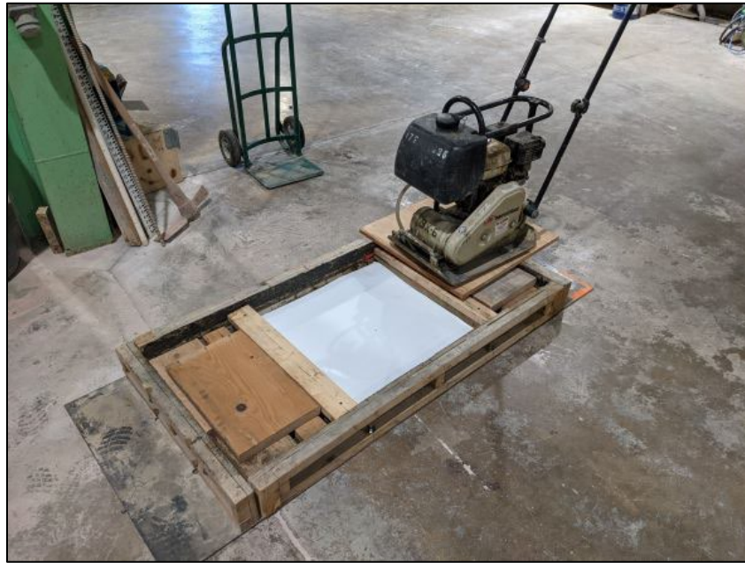
Figure 16. Plate Compactor and Wooden Mold.
