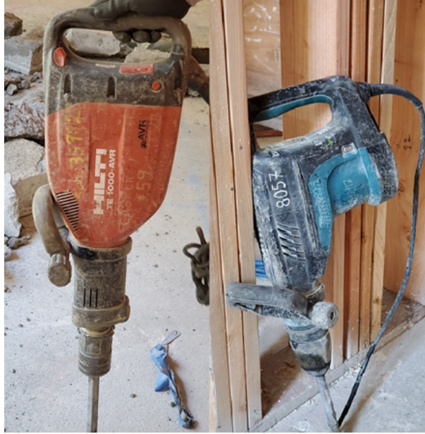
Figure 5. Two different jackhammer types were used by the worker.
