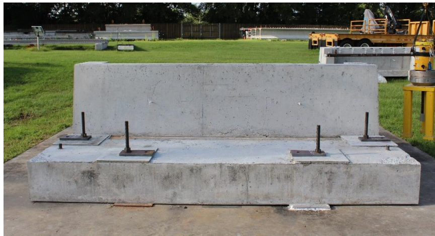
Figure 7-13 Anchored test specimen
