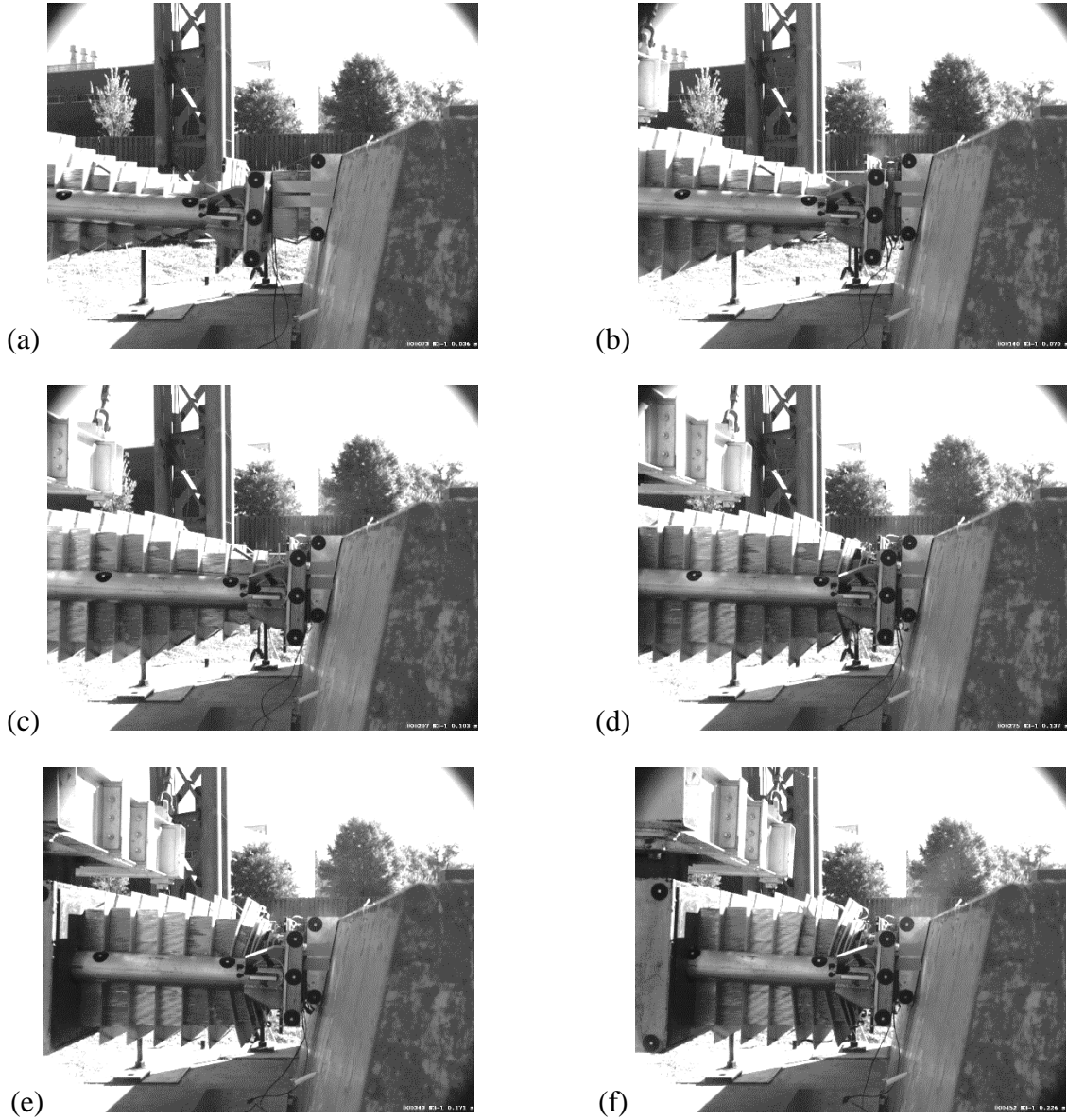
Figure 8-19 High-speed video frames from HSC-1 (R/C COR test 2) showing crush deformation of aluminum honeycomb: (a) At initial impact; (b) – (c) Intermediate frames; (f) At peak impact force
