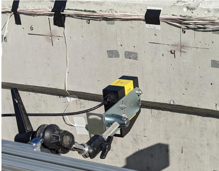
Figure 7-24 Laser displacement sensor mounted behind a test specimen
