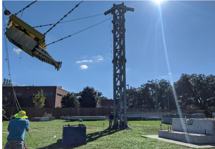
Figure 8-1 Impactor pulled back to 15-ft drop height (prior to release)
