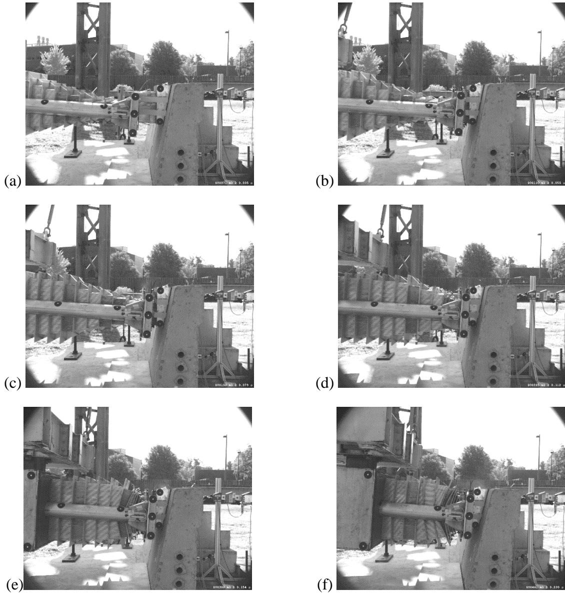
Figure 9-22 High-speed video frames from HSC-1 (GFRP EOR test 1) showing crush deformation of aluminum honeycomb: (a) At initial impact; (b) – (c) Intermediate frames; (f) At peak impact force
