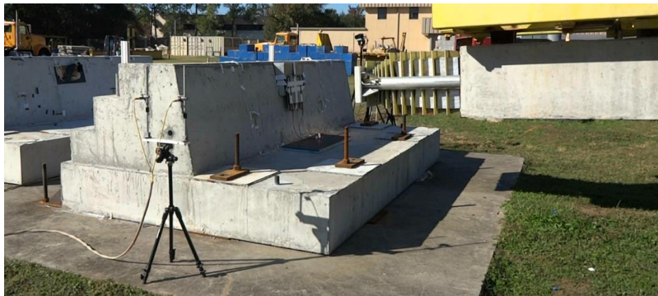
Figure 8-21 R/C COR test 2 specimen after completion of impact test
