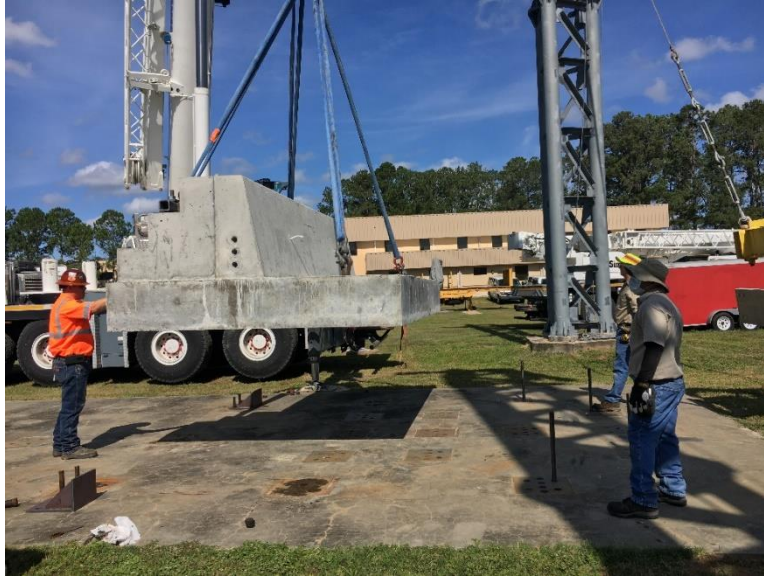
Figure 7-8 Test specimen being moved into position on the pendulum foundation
