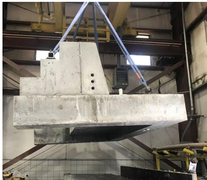
Figure 7-7 Test specimen lifted out of the formwork by crane
