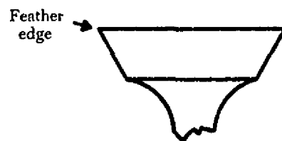
FIGURE 10-16. Engine valves showing normal margin and a feather edge.
