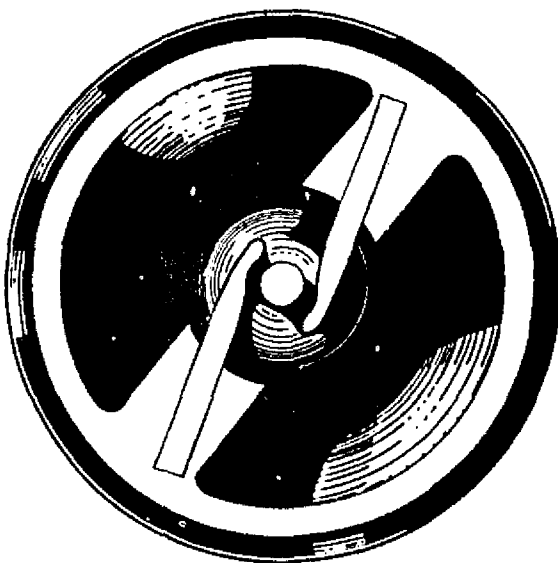
FIGURE 4-54. Spark plug gap erosion.
