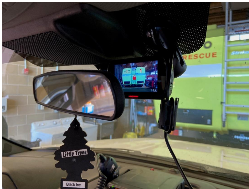
Figure 3.2: Mounted Dash Camera Inside the Airport Maintenance Vehicle
