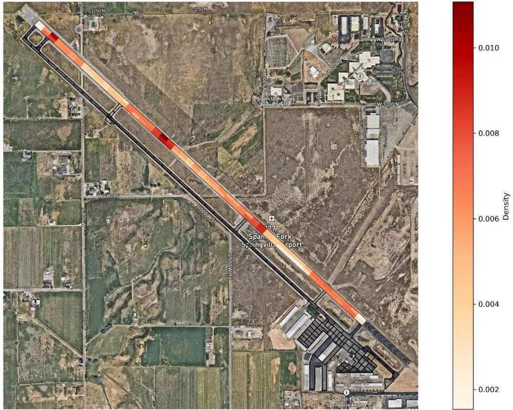
Figure 5.11: Density of detected distresses where (a) is longitudinal and transverse cracking, (b) rutting/depression, (c) weathering within pavement segments.
