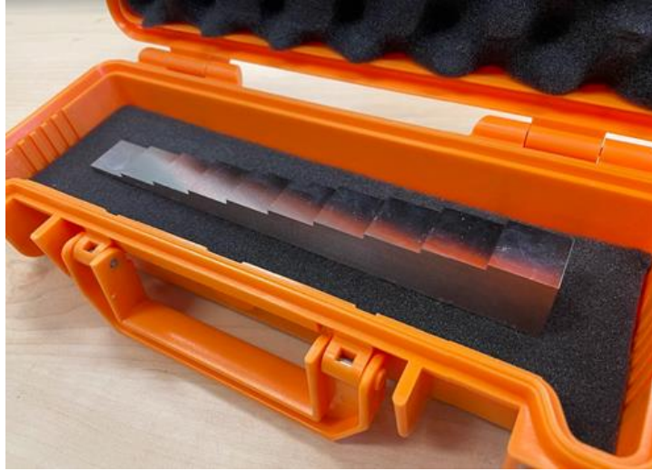
Figure 4. Photograph. Steel calibration block from 0.1- to 1.0-inch thicknesses.
