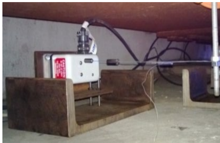
Figure 7.2: Linear potentiometer (string potentiometer) for measuring displacements.
