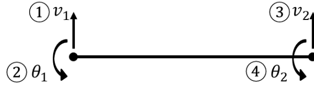
Figure 8.8: Degrees of freedom for a 2-noded frame element.
