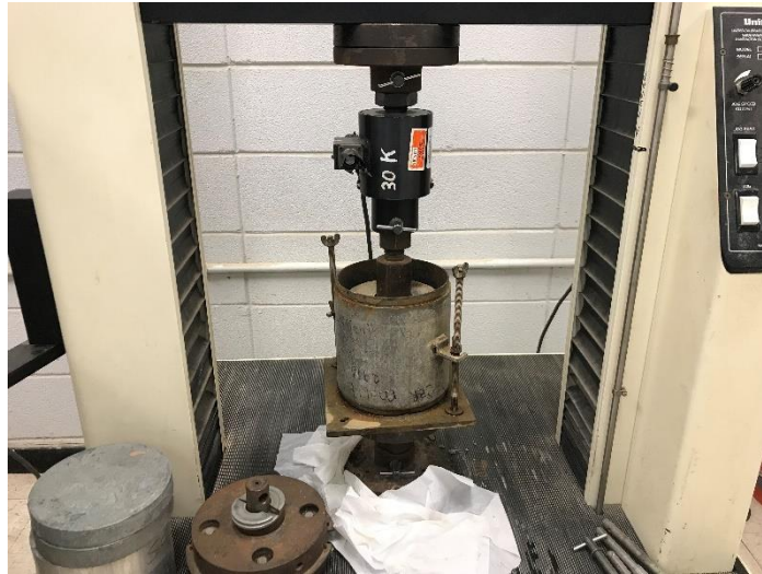
Figure 42. California bearing ratio (CBR) test
