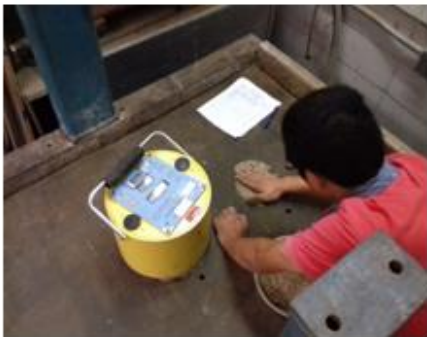
(a) Geogauge test
