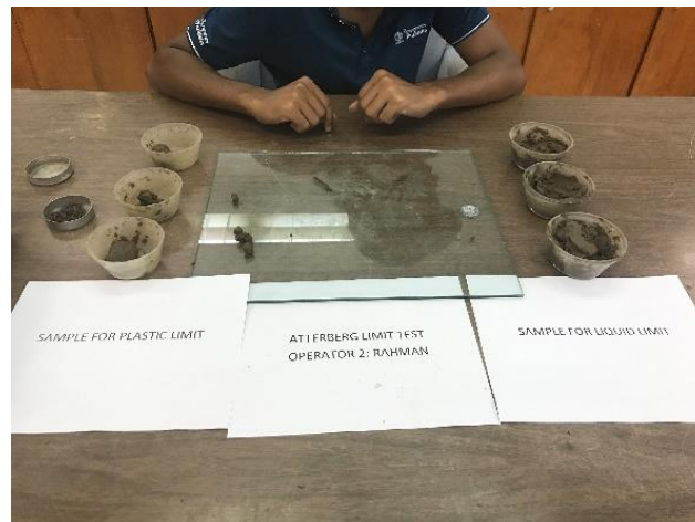
Figure 39. Samples prepared for the Atterberg limit tests
