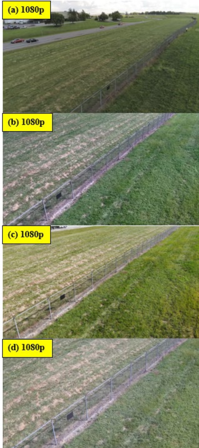
Figure 70. Recorded Visual Camera Footage of Test Area 3 from 20 ft AGL: (a) ANAFI Triple, (b) Z30, (c) M2ED, and (d) XT2 9mm
