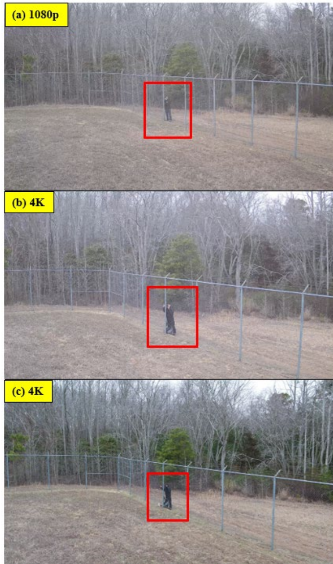
Figure 25. Recorded Visual Camera Footage of Human Subject from 10 ft AGL: (a) XT2 9mm, (b) XT2 13mm, and (c) X5S
