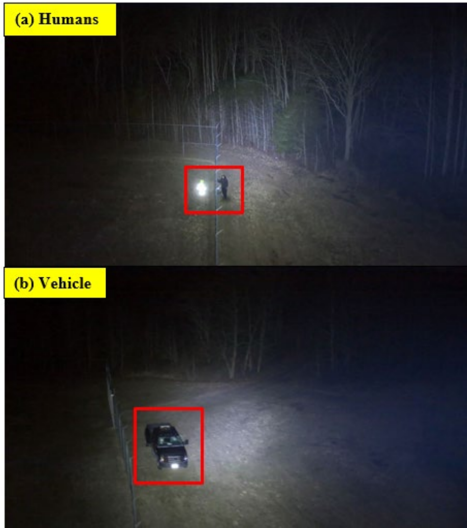
Figure 31. Z15 Spotlight and XT2 13mm Visual Camera Performance from 40 ft AGL: (a) Human Subject and (b) Vehicle
