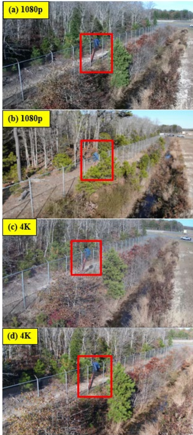
Figure 35. Recorded Visual Camera Footage of Ladder and Blanket from 20 ft AGL: (a) Z30, (b) M2ED, (c) XT2 9mm, and (d) X5S
