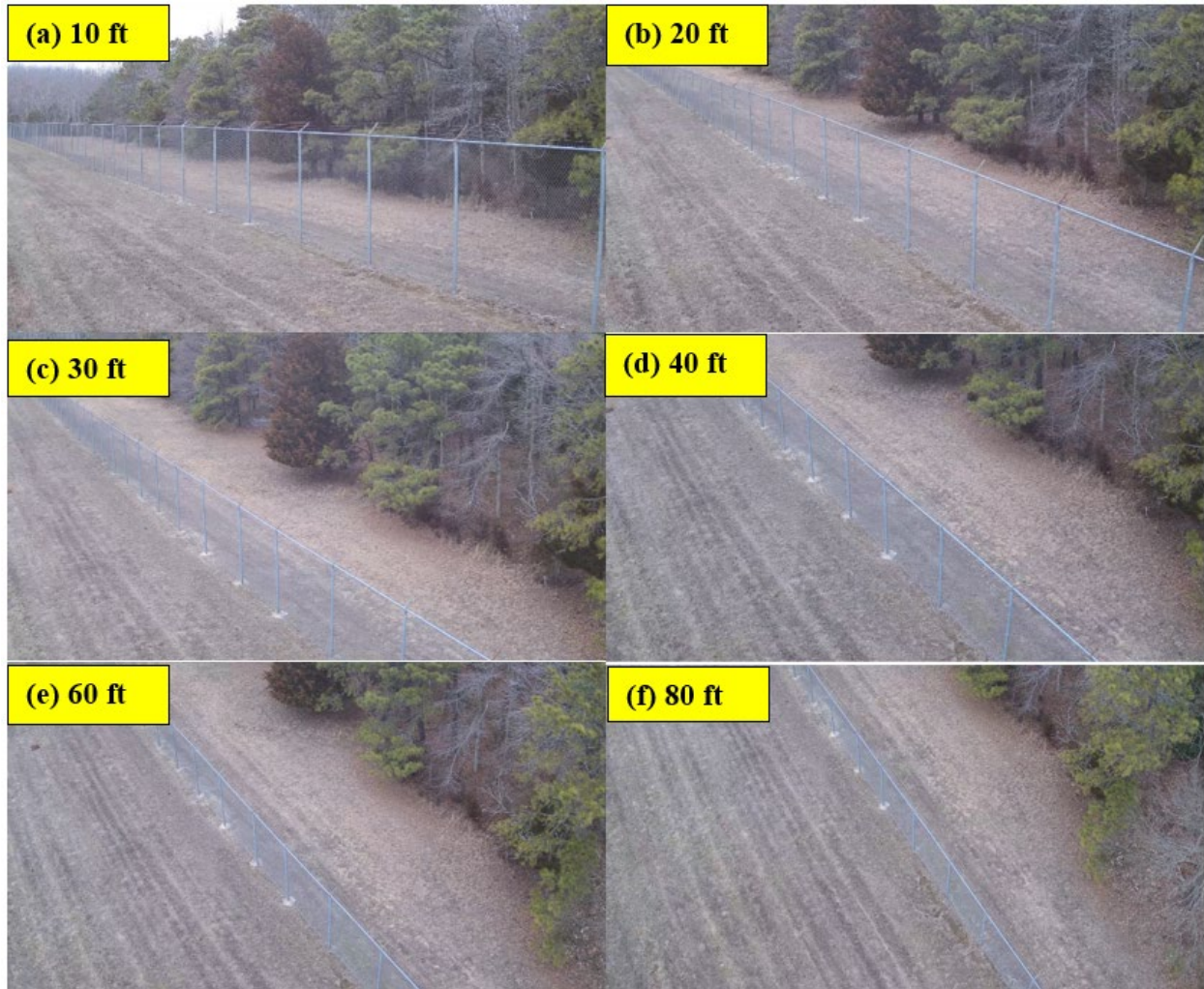
Figure 22. 0-ft Offset and 0-Degree Horizontal Camera Angles at Different AGL Altitudes from Zenmuse X5S
