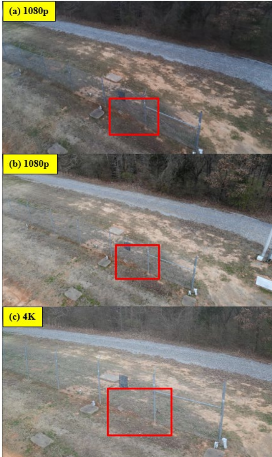
Figure 52. Twilight Recorded Visual Camera Footage of Shovel from 20 ft AGL: (a) ANAFI Triple, (b) M2ED, and (c) XT2 9mm
