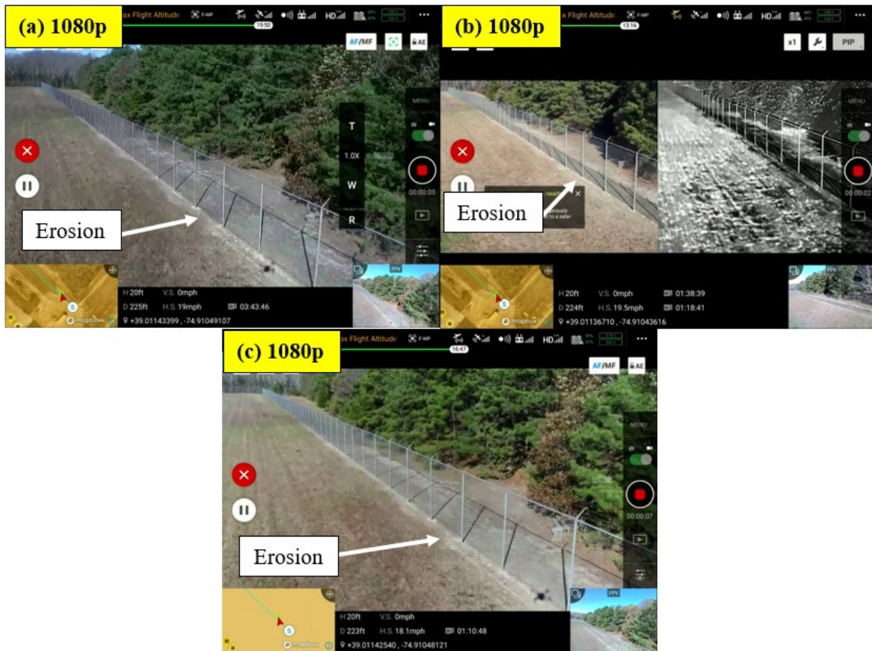
Figure 39. Live-Streamed Camera Footage of Erosion from 20 ft AGL: (a) Z30, (b) XT2 13mm, and (c) X5S
