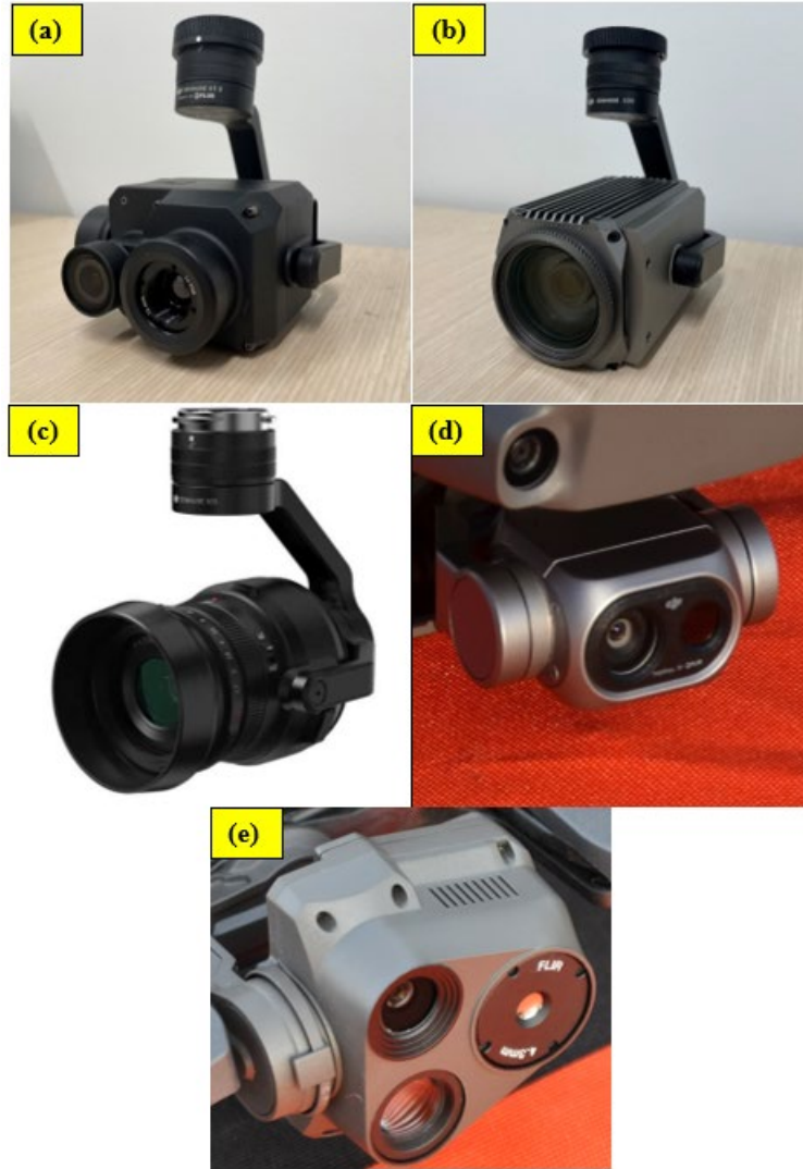
Figure 7. Unmanned Aircraft System Camera Payloads: (a) DJI Zenmuse XT2, (b) DJI Zenmuse Z30, (c) Zenmuse X5S, (d) M2ED Integrated Camera, and (e) Parrot ANAFI Triple
