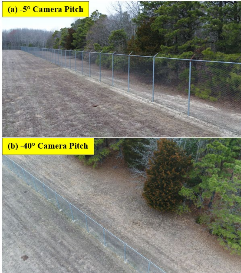
Figure 24. Camera Pitch Angles: (a) -5° Pitch from 10 ft AGL and (b) -40° Pitch from 60 ft AGL
